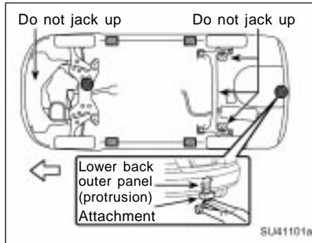
When jacking up your vehicle with the jack, position the jack correctly as shown in the illustration.
