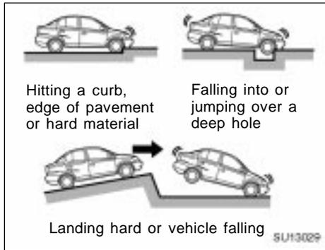
**The front SRS airbags may also deploy if a serious impact occurs to the underside of your vehicle. Some examples are shown in the illustration.**
