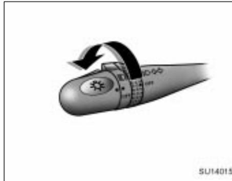
To turn on the front fog lights, twist the band of the headlight and turn signal switch lever. They will come on when the tail lights are turned on.
