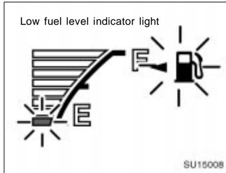
If the low fuel level indicator light blinks, fill the fuel tank as soon as possible.
