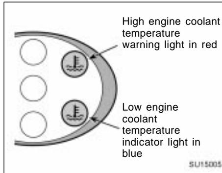
**The indicator and warning lights indicate the engine coolant temperature when the ignition switch is on. The engine operating temperature will vary with changes in weather and engine load.**
