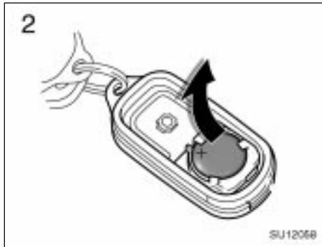
2. Remove the discharged transmitter battery.
