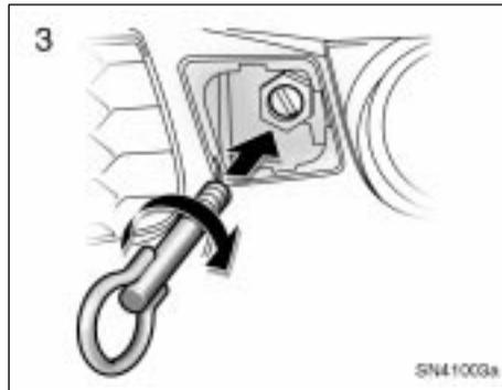
3. Secure the front towing eyelet to the hole on the bumper by turning clockwise.
