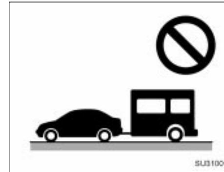
Toyota does not recommend towing a trailer with your Echo. It is not designed for trailer towing.
