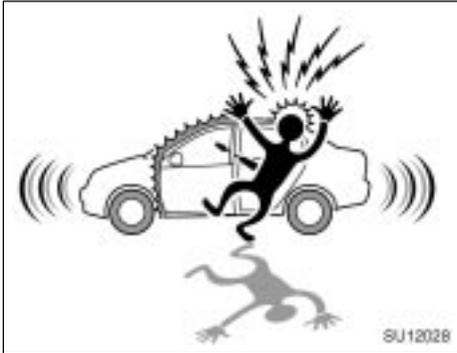
To deter the vehicle theft, the system is designed to sound an alarm if any of the doors, trunk or hood is forcibly unlocked or the battery terminal is disconnected and then reconnected when the vehicle is locked.
