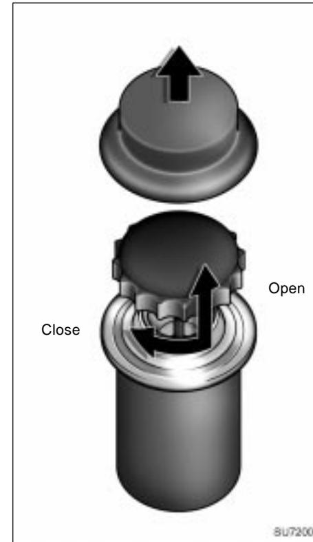
**Check the fluid level through the reservoir. If necessary, add automatic transmission fluid DEXRON®II or III.**
