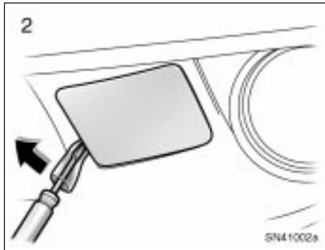
2. Remove the front towing eyelet cover on the front bumper, using a flat-bladed screwdriver which is wrapped with a cloth.
