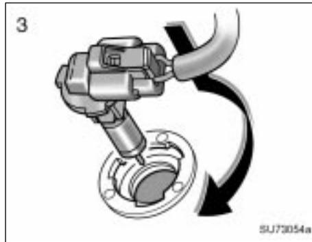
**3. Install a new bulb base by turning it
