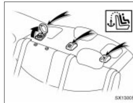
2. Open the anchor bracket cover with the mark shown in the illustration.
