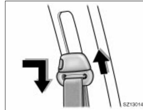
Seat belts with an adjustable shoulder anchor (4-door models)—
