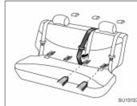
On the vehicle with non-separate non-foldable fixed type seatback, a seat belt for the rear center seat is prepared in the front of a lower anchor. Therefore, in case of fixing the child restraint system to the rear left seat, slide the seat belt for the rear center seat as shown in the illustration and fix it to the lower anchor.
