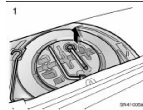
1. Remove the front towing eyelet as shown in the illustrations.
