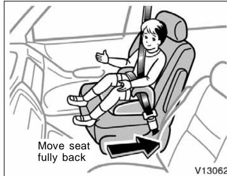
● On vehicles with side airbags, do not allow the child to lean against the front door or around the front door even if the child is seated in the child restraint system. It is dangerous if the side airbags inflate, because the impact could cause death or serious injury to the child.
