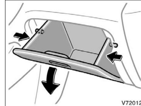
2. Open the glove box and push each side of the glove box to disconnect the claws.
