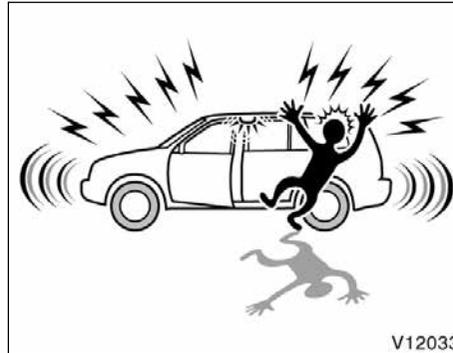
**To deter the vehicle theft, the system is designed to sound an alarm if any of the side doors, back door or hood is forcibly unlocked or the battery terminal is disconnected and then reconnected when the system is set.**
