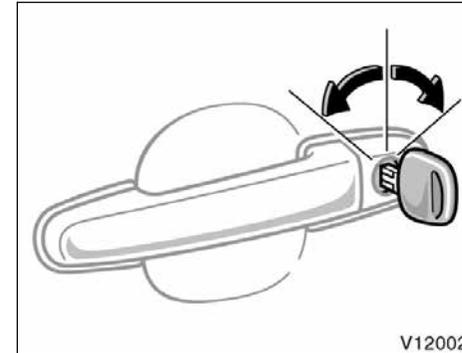
**LOCKING AND UNLOCKING WITH KEY**
