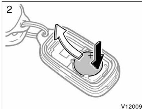
2. Remove the discharged transmitter battery.
