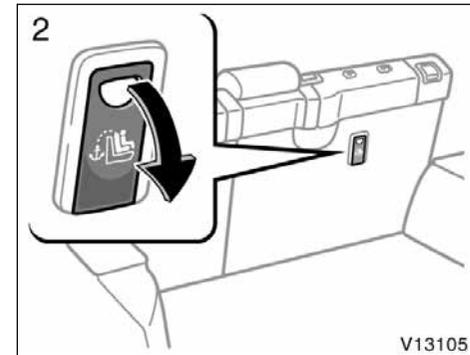
**2. Open the anchor bracket cover with the symbol as shown in the illustration.**
