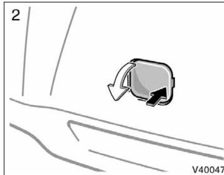
2. Remove the front towing eyelet cover on the front bumper by pushing the outside of the cover.
