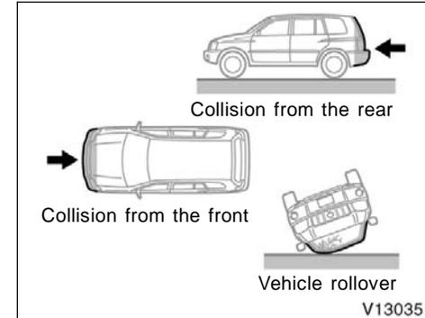
The SRS side airbags are not designed to inflate if the vehicle is involved in a front or rear collision, if it rolls over, or if it is involved in a low-speed side collision.
