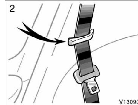
2. Make sure the outer seat belts pass through the hangers when folding the rear seat.
