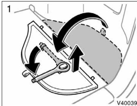
1. Pull up the deck board and remove the front towing eyelet by turning it counterclockwise. (For the towing eyelet location, see “—Required tools and spare tire” on page 221 in this section.)
