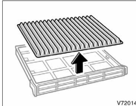
5. Remove the filter from the filter case.
