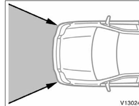
The SRS front airbag system is designed to activate in response to a severe frontal impact within the shaded area between the arrows in the illustration.
