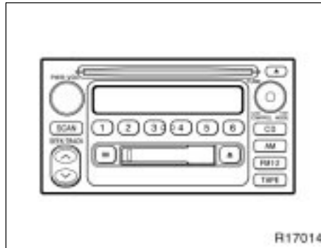
Type 3: AM-FM radio/cassette player/compact disc player (with compact disc auto changer controller)
