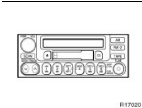
Type 2: AM-FM radio/cassette player (with compact disc changer controller)
