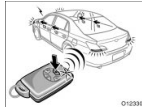
Locking operation (vehicles with smart key system)
