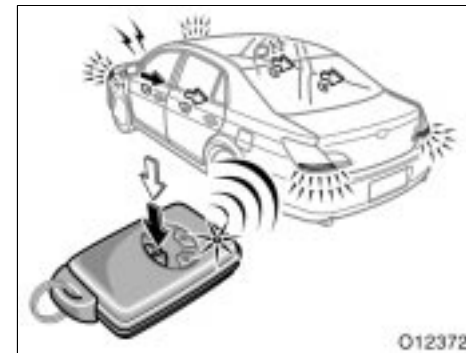
Unlocking operation (vehicles with smart key system)
