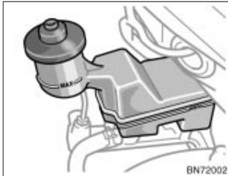
If the level is low, add SAE J1703 or FMVSS No.116 DOT 3 brake fluid to the brake reservoir.
