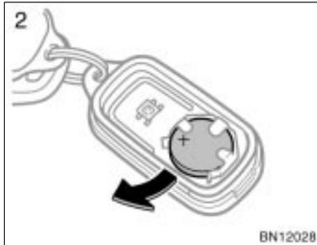
2. Remove the discharged transmitter battery.
