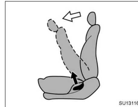
Lift the seatback release lever—the seatback will tilt forward.
