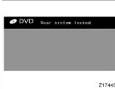
When the rear system lock is on and any button is pushed on the remote controller or the operation panel, the screen shown above is displayed for approximately 6 seconds.
