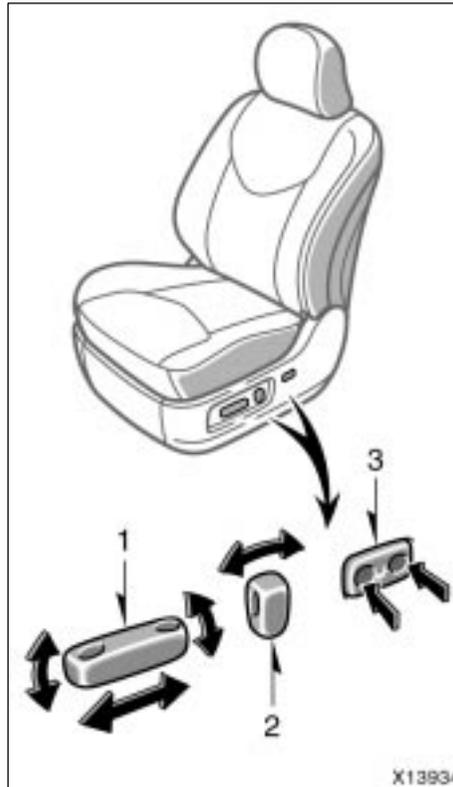
**1. SEAT POSITION, SEAT CUSHION ANGLE AND SEAT HEIGHT ADJUSTING SWITCH**
