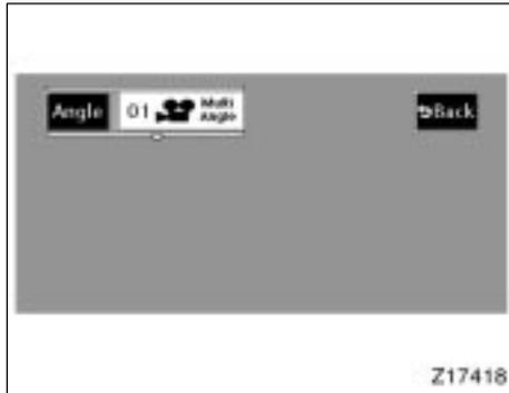
The angle can be selected for discs that are multi-angle compatible when the “
