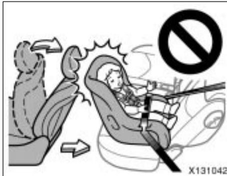
● Do not install a child restraint system on the rear/second or third seat if it interferes with the lock mechanism of the front or second seats. Otherwise, the child or front or second seat occupant(s) may be killed or seriously injured in case of sudden braking or a collision.
