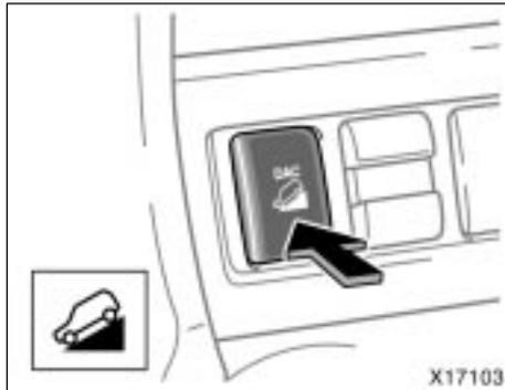
**2. Push the “DAC” switch to turn the system on. The downhill assist control system indicator light will come on.**
