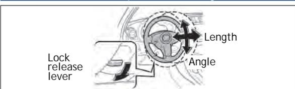
Hold wheel, push lever down, set angle and length, then return lever.
