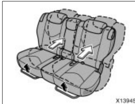
After installing the child restraint system, move the rear/second seat to the rear-most lock position to prevent the child restraint system from interfering with the front seat.
