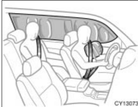
The SRS (Supplemental Restraint System) side airbags and curtain shield airbags are designed to provide further protection for the driver, front passenger and rear seat passengers\*1/second seat passengers\*2 in addition to the primary safety protection provided by the seat belts.
