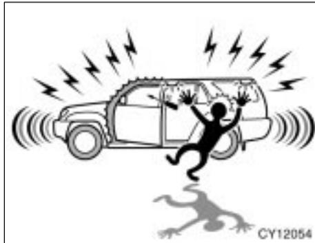
To deter vehicle theft, the system is designed to sound an alarm if any of the side doors, back door or hood is forcibly unlocked or opened or the battery terminal is disconnected and then reconnected when the vehicle is locked. The alarm blows the horn intermittently and flashes the headlights, tail lights and turn signal lights, and turns on the interior and luggage compartment lights.
