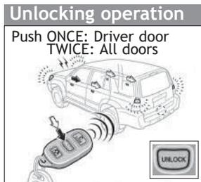
**NOTE:** After unlocking, if a door is not opened within 30 seconds, all doors will relock for safety.
