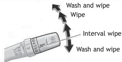
**NOTE:** Rear wiper and washer operate only when rear window is fully closed. If battery is disconnected, rear washer will not function until rear window is reinitialized by being fully opened and then closed.
