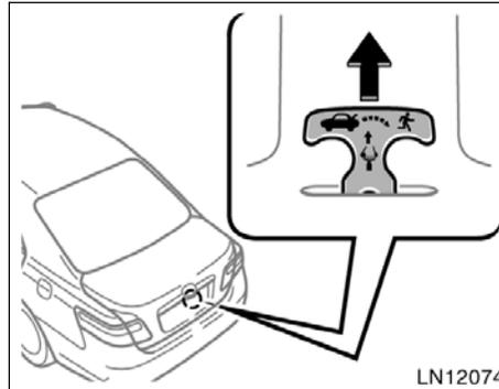
If a person is locked in the trunk, he/she can pull up the phosphorescent strap on the inside of trunk lid to open the trunk lid.
