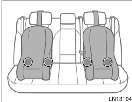
**Lower anchorages for the child restraint systems interfaced with the FMVSS225 or CMVSS210.2 specifications are installed in the rear seat.**
