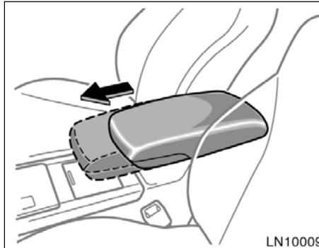
On some models—it is possible to use the rear console box lid as an armrest by moving it. To move it, grasp the front of the lid and pull forward as shown in the illustration.
