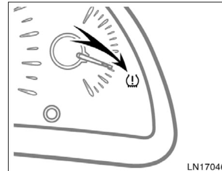
The tire pressure warning light comes on when the ignition switch is set at ON and goes off after a few seconds. This means the tire pressure warning system is operating properly. If the tire inflation pressure becomes low, the light comes on again. In this case, adjusting the tire inflation pressure will turn off the light after a few minutes. If the light comes on after blinking for 1 minute, the tire pressure warning system is not working properly.
