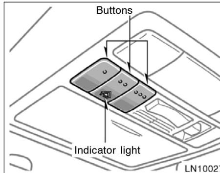
The garage door opener (**HomeLink<sup>®</sup>** Universal Transceiver) is manufactured under license from HomeLink<sup>®</sup> and can be programmed to operate garage doors, gates, entry doors, door locks, home lighting systems, and security systems, etc.
