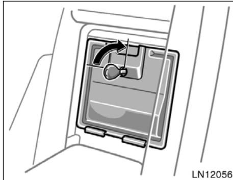
2. Vehicles with trunk storage extension—After closing the door located behind the rear seat armrest, insert the master key (vehicles with key cylinder-type ignition switch) or mechanical key (vehicles with smart key system) and turn it clockwise to lock the door.
