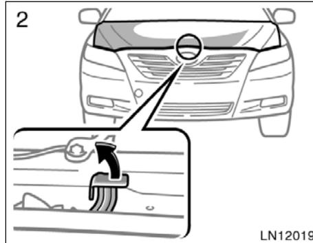
2. In front of the vehicle, pull up the auxiliary catch lever and lift the hood.
