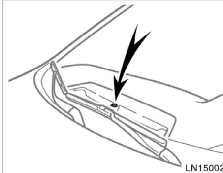
The automatic light control sensor is on the top of the instrument panel.
