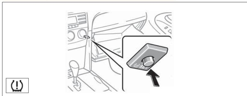
If tire pressure becomes low on any of the tires (including spare/excluding compact spare), indicator comes on. Pushing reset button should not turn off the light. Correctly adjusting tire inflation will turn off the light after a few minutes. Push and hold reset button, until the indicator light blinks 3 times, after replacing tire or wheels.
