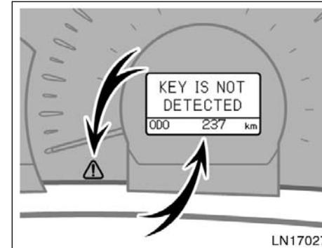
If a buzzer sounds and the master warning light comes on for 5 seconds when pressing the “ENGINE START STOP” switch, this indicates that the key is not in the vehicle. The “KEY IS NOT DETECTED” message will also appear on the multi-information display.
