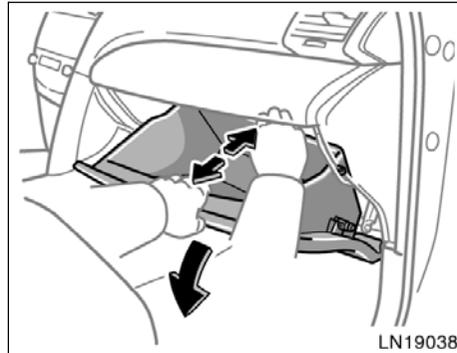
2. Apply pressure to the glove box as shown to disengage the claws.
