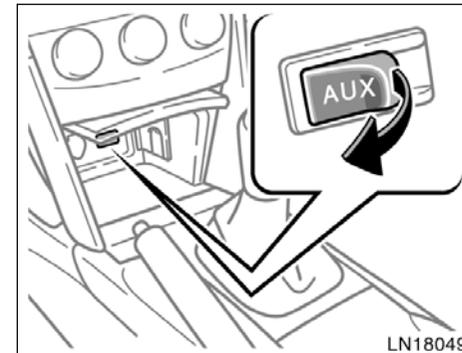
**An AUX adapter is installed inside the auxiliary box.**
