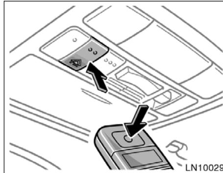
3. Simultaneously press and hold the hand-held garage transmitter button along with the selected HomeLink® button.
