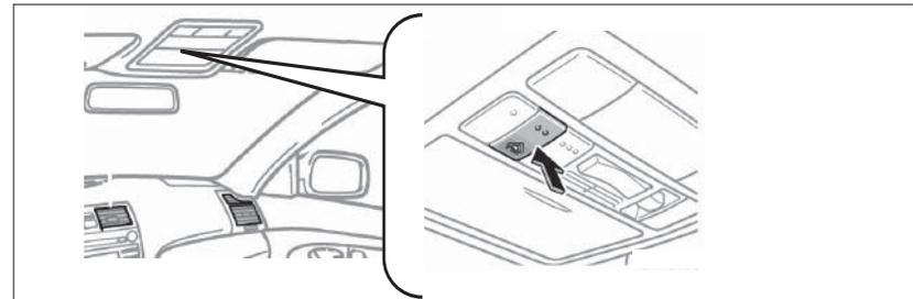
Garage door openers manufactured under license from HomeLink®\* can be programmed to operate garage doors, estate gates, security lighting, etc.
