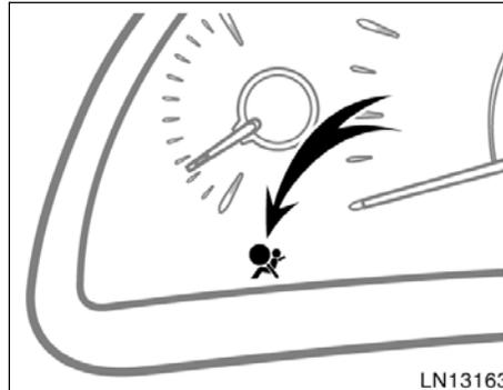
**This indicator comes on when the ignition switch is set at ON. It goes off after about 6 seconds. This means the SRS side airbags and curtain shield airbags are operating properly.**
