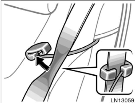
2. Pinch the two edges of the shoulder belt for the rear seat outside position with your fingers and slide the belt past the slot of the guide as shown above. At this time, the elastic cord must be behind the seat belt.
