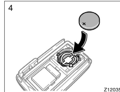
4. Put in a new battery with the positive (+) side up. Install the cover and insert the mechanical key into the transmitter. Close the transmitter case securely.
