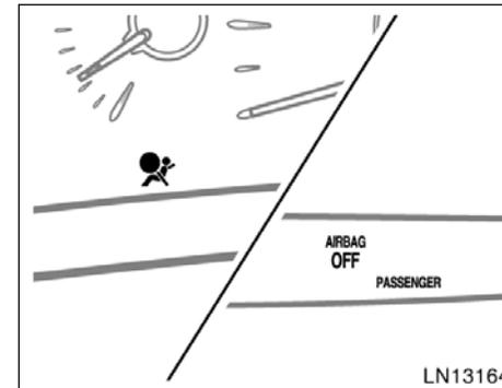
The SRS warning and “AIRBAG OFF” indicator lights will come on if there is a malfunction in the front passenger occupant classification system.
