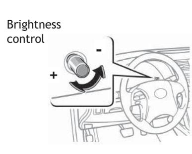
With the knob turned fully clockwise, instrument panel lights will not dim when the headlights are turned on.
