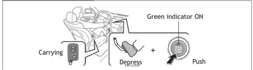
**NOTE:** Gear shift lever must be in Park and brake pedal depressed.
