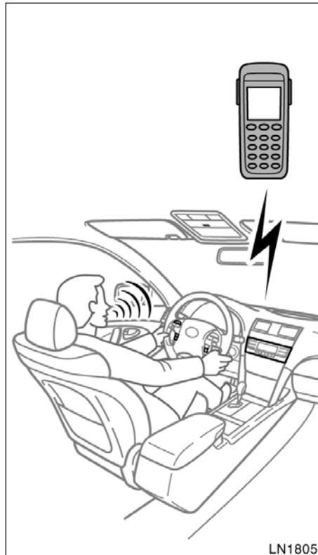
This system supports Bluetooth®, a wireless system that allows you to make or receive calls without taking your hands from the steering wheel and without using cables to connect the phone and system.
