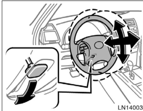
To adjust the steering wheel position, hold the steering wheel, push down the lock release lever. Then tilt the steering wheel to the desired angle, push or pull it to the desired steering column length and return the lever to its original position.
