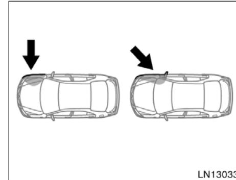
The SRS side airbag and curtain shield airbag system may not activate if the vehicle is subjected to a collision from the side at certain angles, or a collision to the side of the vehicle body other than the passenger compartment as shown in the illustration.
