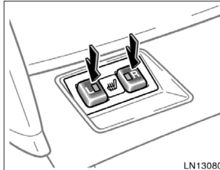
To turn on the seat heater, push the switch. At this time, the indicator light will illuminate to indicate the seat heater is operating.
