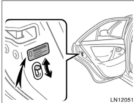
Move the lock lever to the “LOCK” position as shown on the label.
