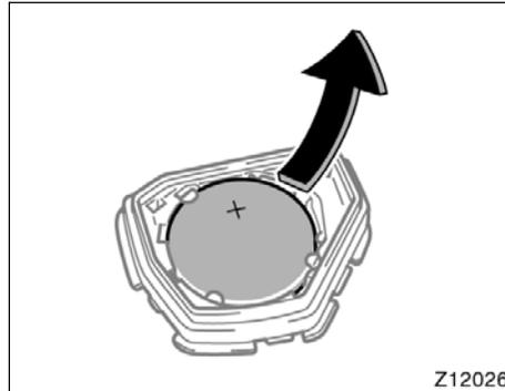
4. Take out the discharged transmitter battery and put in a new battery with the positive (+) side up.
