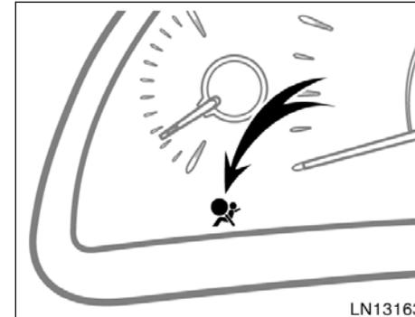
This indicator comes on when the ignition switch is set at ON. It goes off after about 6 seconds. This means the seat belt pretensioners are operating properly.
