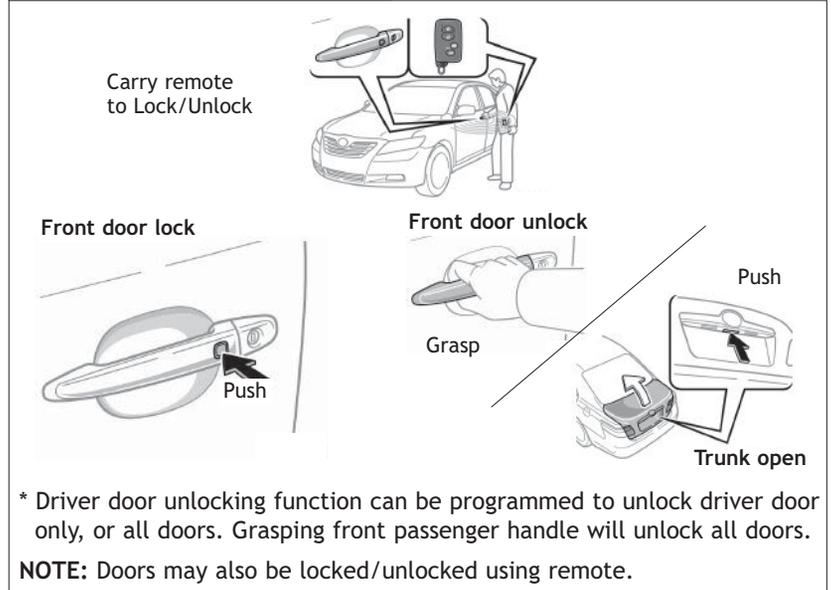
\* Driver door unlocking function can be programmed to unlock driver door only, or all doors. Grasping front passenger handle will unlock all doors.
