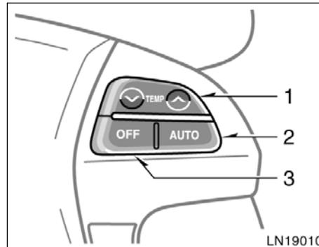
Some parts of the air conditioning system can be adjusted using the switches on the steering wheel.
