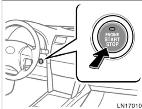
When the key is in the vehicle, pressing the “ENGINE START STOP” switch (engine switch) allows you to start and stop the engine or choose at the ACC, ON, or ignition switch off.
