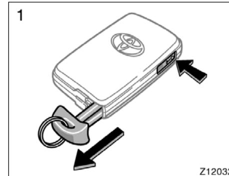
1. Push the release button and take out the mechanical key.
