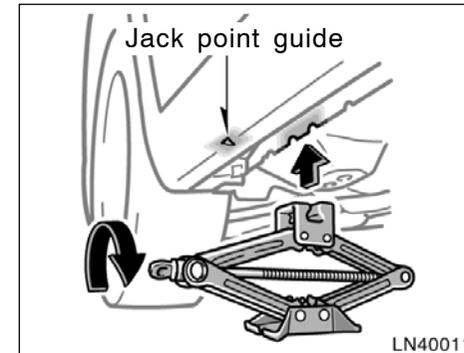
The jack point guides are located under the rocker panel. They indicate the jack point positions.
