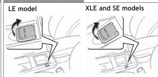
Designed for 12V car accessories. Key/Engine switch must be in the “ACC” or “ON” position to be used.
