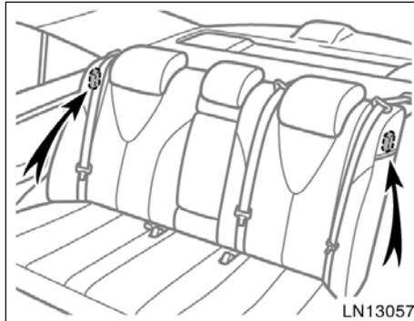
Seat belt comfort guides are stored in the both pockets on the sides of the rear seatback.
