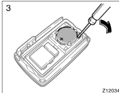
3. Remove the discharged transmitter battery by flathead screwdriver or equivalent. Insert the guide groove and lift as shown in the above illustration.
