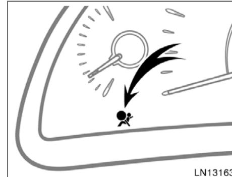
The indicator comes on when the ignition switch is set at ON. It goes off after about 6 seconds. This means the SRS front airbags are operating properly.
