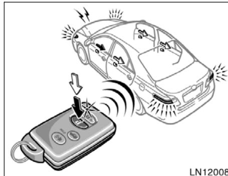
Unlocking operation (vehicles with smart key system)
