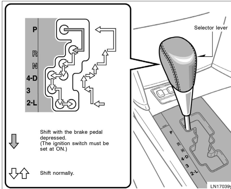
Your automatic transmission has a shift lock system to minimize the possibility of incorrect operation. This means you can only shift out of "P" position when the brake pedal is depressed (with the ignition switch is set at ON).
