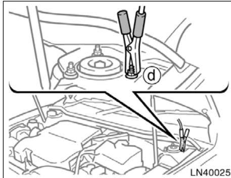
The recommended connecting point is (d) in the above illustration.
