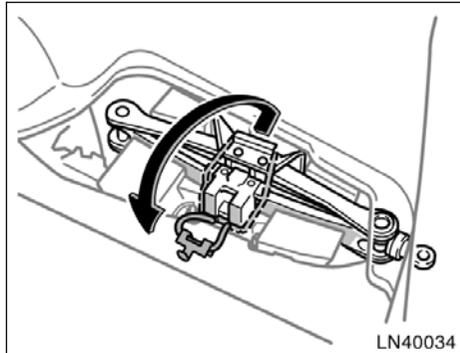
Before removing the jack, unhook the tightening strap.
