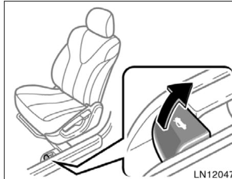
**To open the trunk lid from the driver's seat, pull up on the lock release lever.**
