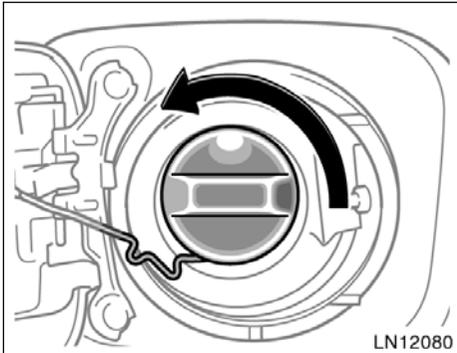
2. To remove the fuel tank cap, turn the cap slowly counterclockwise, then pause slightly before removing it.
