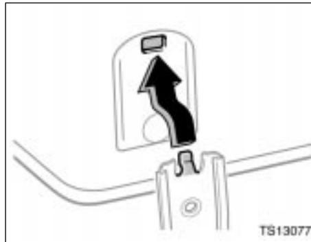
When the bottom cushion is reinstalled, click the claw of the hinge into the hole of the bottom cushion before refastening the dial.
