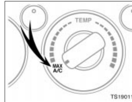
For quick cooling, turning the temperature selector knob fully towards COLD (MAX A/C) changes the air intake selector mode to RECIRCULATE.
