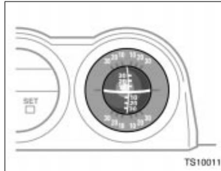
The clinometer shows longitudinal and lateral inclination of the vehicle. The display ranges between 30° and -30°.
