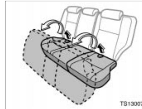
1. Swing the bottom cushion up by pulling the lock release strap.
