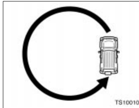
3. Drive the vehicle in a circle at 8 km/h (5 mph). If there is not enough space to drive in a circle, drive around the block.
