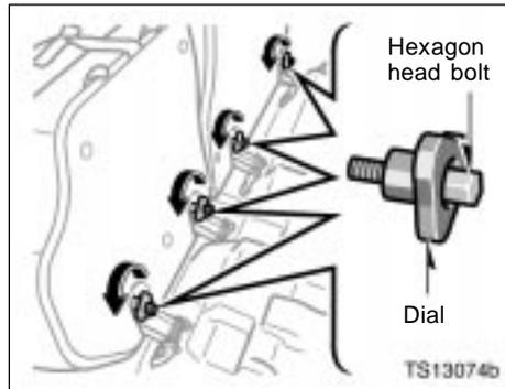
**2. Loosen the bolts with the wrench at first and turn the dials with hands to remove them.**
