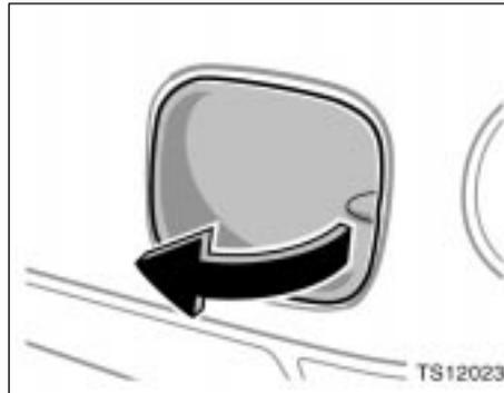
1. To open the fuel filler door, pull the door toward out as shown.
