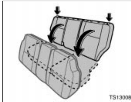
**3. Push the lock release button and fold down the seatback.**
