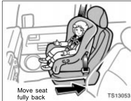
▶ On vehicles with side airbags and curtain shield airbags, do not allow the child to lean his/her head or any part of his/her body against the door or the area of the seat, front or rear pillar or roof side rail from which the side airbags or curtain shield airbags deploy even if the child is seated in the child restraint system. It is dangerous if the side airbag and/or curtain shield airbag inflate, and the impact could cause death or serious injury to the child.
