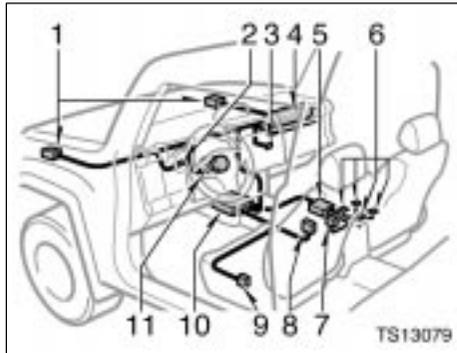
The SRS front airbag system consists mainly of the following components, and their locations are shown in the illustration.
