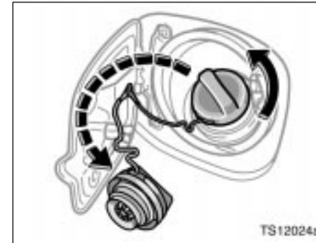
2. To remove the fuel tank cap, turn the cap slowly counterclockwise, then pause slightly before removing it. After removing the cap, hang the tether as shown in the illustration.
