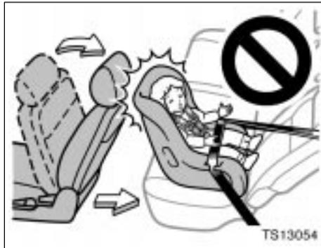
► Do not install a child restraint system on the rear seat if it interferes with the lock mechanism of the front seats. Otherwise, the child or front seat occupant(s) may be killed or seriously injured in case of sudden braking or a collision.
