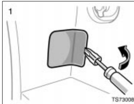
Use a flathead screwdriver which is wrapped with a cloth.
