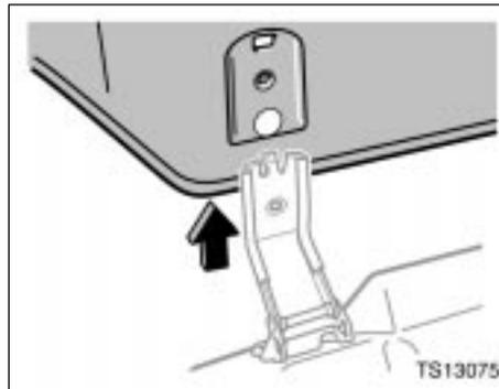
**3. Separate the bottom cushion from the hinge.**
