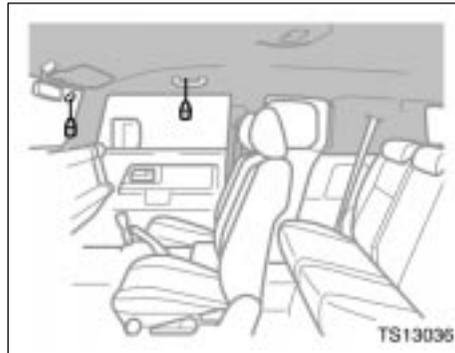
▶ Do not attach a microphone or any other device or object around the area where the curtain shield airbag activates such as on the windshield glass, side door glass, front and rear pillars, roof side rail and assist grips. When the curtain shield airbag inflates, the microphone or other device or object will be thrown away with great force or the curtain shield airbags may not activate correctly, resulting in death or serious injury.
