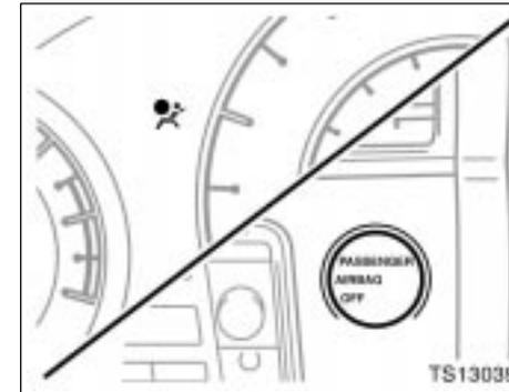
The SRS warning light will come on and front passenger occupant classification indicator light will indicate "OFF" if there is a malfunction in the front passenger occupant classification system. Contact your Toyota dealer as soon as possible.
