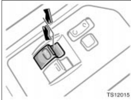
**The windows can be operated with the switch on either front door.**
