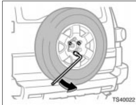
2. Turn the hold-down nuts counter-clockwise with the wheel nut wrench and remove them.
