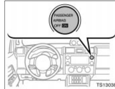
The front passenger occupant classification indicator light indicates the actuation of the front passenger airbag, side airbag on the front passenger seat.
