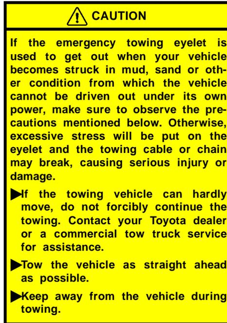
**—Tips for towing a stuck vehicle**
