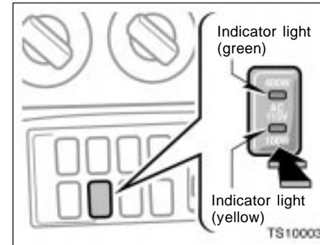
**To use the power outlet, push the main switch located on the instrument panel.**
