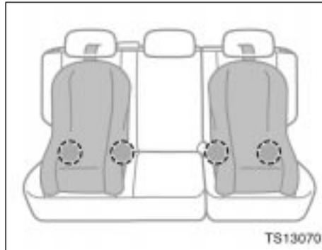
**Lower anchorages for the child restraint systems complying with the FMVSS225 or CMVSS210.2 specifications are installed in the rear seats.**
