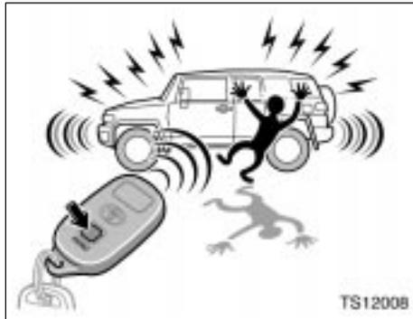
**Pushing the “PANIC” switch blows the horn intermittently and flashes the headlights, tail lights, turn signal lights and outside rear view mirror illumination light (on some models), and turns on the interior and luggage compartment lights.**
