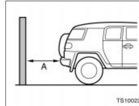
The intuitive parking assist is designed to inform you of the approximate distance between your vehicle and an obstruction by buzzer while driving at approximate 10 km/h (6 mph) or less when parking the vehicle. This system uses sensors to detect obstructions.
