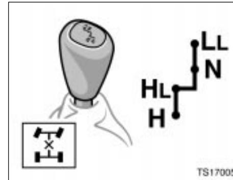
Use the four-wheel drive control lever to select the following transfer modes.
