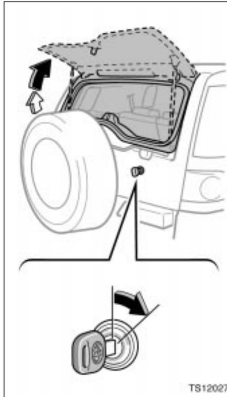
**To open the back window, turn the key clockwise and hold it for about 1 second.**
