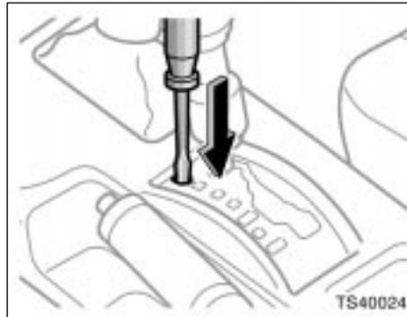
3. Insert the screwdriver or equivalent into the hole to push down the shift lock override button. You can shift out of the “P” position only while pushing the button.
