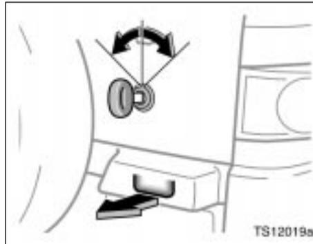
**Insert the key into the key hole and turn it.**
