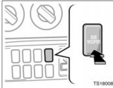
To operate the sub woofer, push the sub woofer on-off switch.
