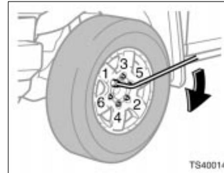
**10. Lower the vehicle completely and tighten the wheel nuts.**
