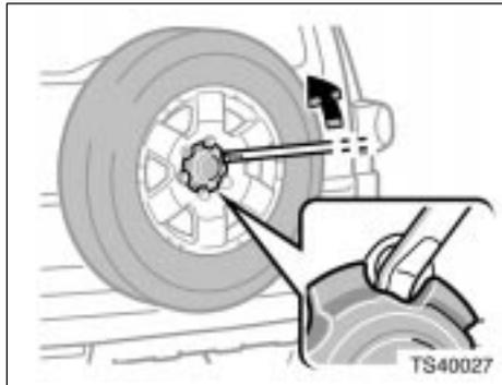
To remove the spare tire on the back door:
