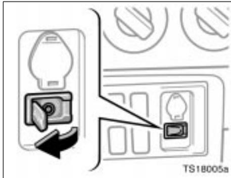
An AUX adapter is installed on the instrument panel.
