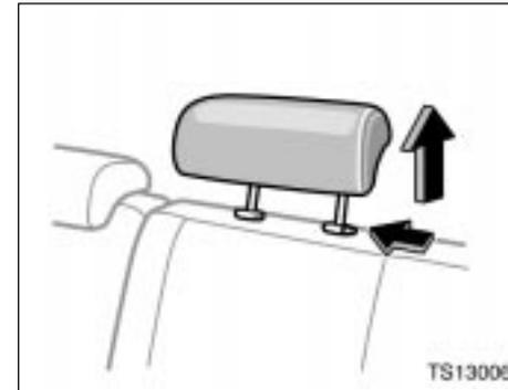
1. Remove the head restraint.
