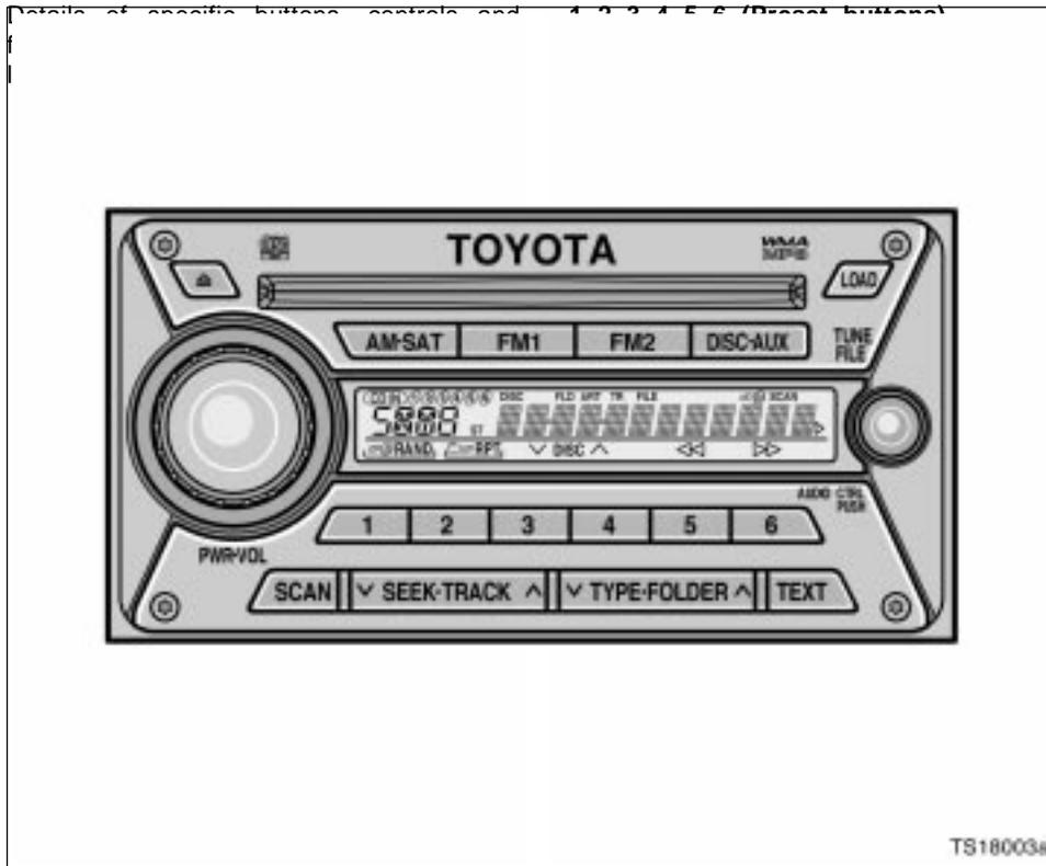
To recall a preset channel: Push the button for the channel you want. The preset button number and channel number will appear on the display.
