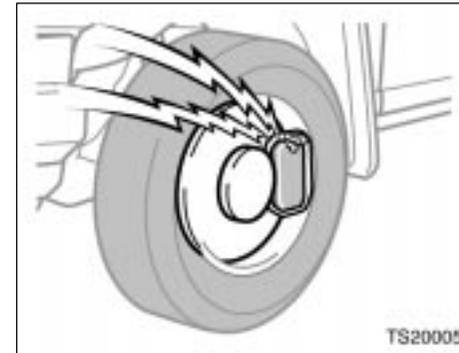
**The brake pad wear limit indicators on your disc brakes give a warning noise when the brake pads are worn to where replacement is required.**
