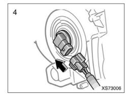
4. Install the connector to the bulb.
