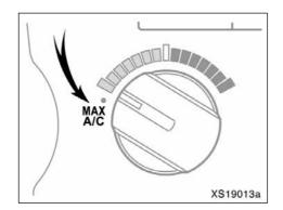
For quick cooling, turn the temperature selector knob to the "MAX A/C" position. The air conditioning will automatically turn on and the air intake selector will be set to RECIRCULATE.
