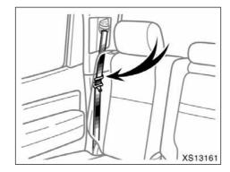
Make sure the shoulder belt passes through the hanger when folding the rear seat.
