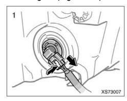
1. Open the hood. Unplug the connector while depressing the lock release.
