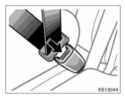
To remove the infant seat: Press the buckle release button and allow the belt to retract completely. The belt will move freely again and be ready to work for an adult or older child passenger.
