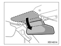
On some models: To block the glare from the front when the main sun visor is swung to the lateral side (position 2), swing down the sub visor.
