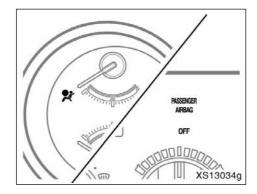
The SRS warning light will come on and the passenger airbag on-off indicator light will indicate "OFF" if there is a malfunction in the front passenger occupant classification system. Contact your Toyota dealer as soon as possible.
