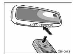
Simultaneously press and hold the hand-held garage transmitter button along with the selected HomeLink<sup>®</sup> button.
