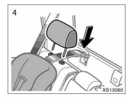
4. Replace the passenger head restraint.
