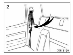
Make sure the shoulder belt passes through the hanger when folding the front passenger's seat.
