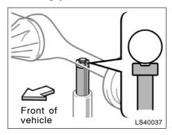
5. After making sure that no one is in the vehicle, as the jack touches the vehicle and begins to lift, double-check that it is properly positioned.
