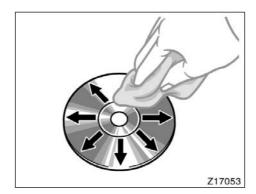
To clean a disc: Wipe it with a soft, lint-free cloth that has been dampened with water. Wipe in a straight line from the center to the edge of the disc (not in circles). Dry it with another soft, lint-free cloth. Do not use a conventional record cleaner or anti-static device.
