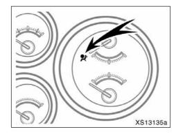
This indicator comes on when the ignition switch is turned to the "ON" position. It goes off after about 6 seconds. This means the seat belt pretensioners are operating properly.
