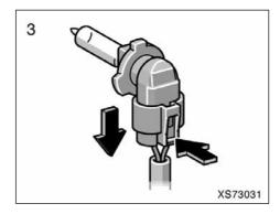
3. Pull the bulb out of the base. Install a new bulb.
