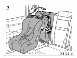
Pull the seatback release lever and swing the seatback forward slightly, then latch the hook onto the anchor bracket. Return the seatback to its original position.
