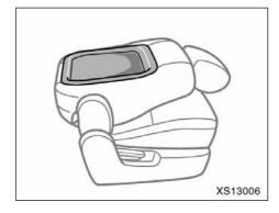
You should use the seatback as a temporary table only when the vehicle is stopped.
