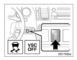
When getting the vehicle out of mud or newly fallen snow, etc., it may be beneficial to turn off the vehicle stability control system. This system that controls engine performance interferes with the process of freeing rear wheels (two-wheel drive models) or 4 wheels (four-wheel drive models).
