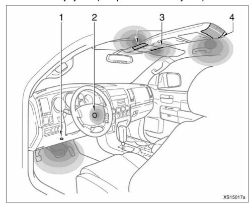
The following lights will come on when any of the doors are opened. After all the doors are closed, the lights remain on for about 15 seconds before fading out.
