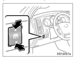
The back window can be operated with the switch on the instrument panel.
