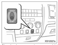
Glass breakage sensor (on some models)
