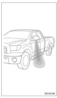
The lights will come on when the doors are unlocked simultaneously using either the power door lock switches or the wireless remote control. This light remains on for 15 seconds before fading out when any door is opened, and additional 15 seconds after all the doors are closed.
