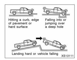
The SRS side and curtain shield airbags may deploy if a serious impact occurs to the underside of your vehicle. Some examples are shown in the illustration.
