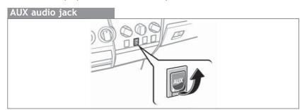
By inserting a mini plug into the AUX audio jack, you can listen to music from a portable audio device through the vehicle's speaker system.
