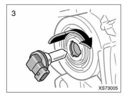
3. Plug in a new bulb install it into the mounting hole.
