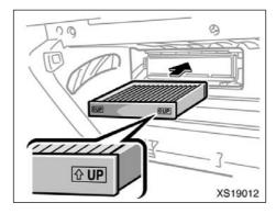
When installing the filter in the filter outlet, keep the arrow pointing up.
