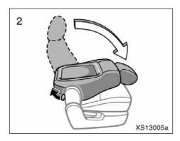
2. Pull the seatback folding lever and fold the seatback down.
