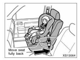
● A forward-facing child restraint system should be allowed to be installed on the front passenger seat only when it is unavoidable. Always move the seat as far back as possible even if the passenger airbag on-off indicator light indicates "OFF", because the front passenger airbag could inflate with considerable speed and force. Otherwise, the child may be killed or seriously injured.
