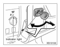
The passenger airbag system is equipped with a off switch and indicator light. Turning the passenger airbag off switch clockwise to the "AUTO" position makes the front passenger airbag system operational. To disable the front passenger airbag system, turn the off switch counterclockwise to the "OFF" position and remove the key. The "OFF" indicator light on the passenger airbag off switch will come on when the front passenger airbag system has been disabled.
