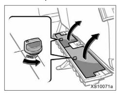
Before using the box, lift up the rear seats. (For detailed information, see "—Raising rear seat cushion (Double cab models)" on page 59 in Section 1-3.)
