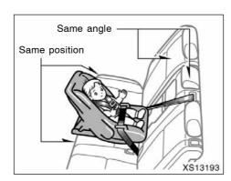
• Crew Max models: When installing a child restraint system in the rear seat center position, adjust both seat cushions to the same position and align both seatbacks at the same angle. Otherwise, the child restraint system cannot be securely restrained and this may cause death or serious injuries in a collision.
