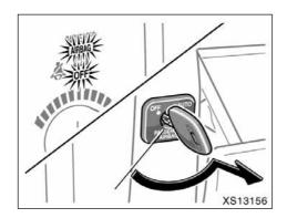
When you install a rear-facing child restraint system which belongs to a passenger risk group on the right front passenger seat, turn the passenger airbag off switch counterclockwise to the "OFF" position and remove the key. (For details, see "—SRS driver airbag and front passenger airbag" on page 75 in this Section.)
