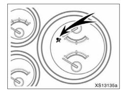
This indicator comes on when the ignition switch is turned to the "ON" position. It goes off after about 6 seconds. This means the SRS side airbags and curtain shield airbags are operating properly.
