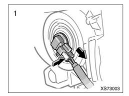
1. Open the hood. Unplug the connector while depressing the lock release.
