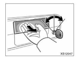
LOCKING AND UNLOCKING WITH KEY Insert the master key into the keyhole and turn it to lock or unlock the tailgate.
