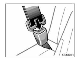
To remove the convertible seat: Press the buckle release button and allow the belt to retract completely. The belt will move freely again and be ready to work for an adult or older child passenger.
