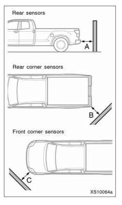
This system is designed to inform you of the approximate distance between your vehicle and an obstacle by indicator and buzzer.
