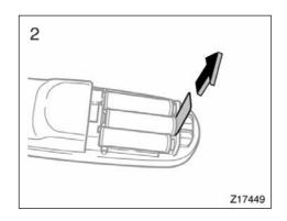
2. Remove the insulating sheet.
