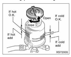
Check the fluid level through the reservoir. If necessary, add automatic transmission fluid DEXRON®II or III.
