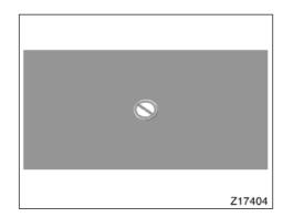
If " $\mathbf{O}$ " appears on the screen when you select a switch, it indicates that the switch cannot work.
