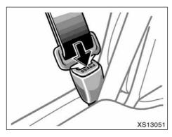
To remove the booster seat: Press the buckle release button and allow the belt to retract.
