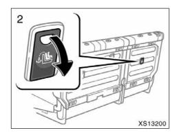
Open the anchor bracket cover with the symbol as shown in the illustration.
