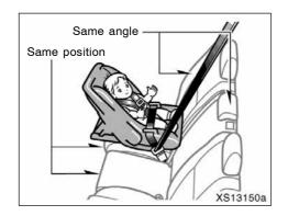
• Bench seat: In order to firmly secure the child restraint system to the right front passenger seat, align the seatback angle and seat position of the right front passenger seat to match the center front passenger seat. Otherwise, it could cause death or injury in a collision.
