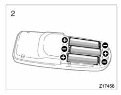
Remove the discharged batteries and put in the new batteries as shown. Install the cover.
