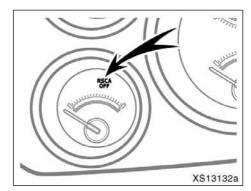
• Make sure the "RSCA OFF" indicator light is off. The curtain shield airbags will not inflate in a vehicle rollover if this indicator light is on and you may be killed or seriously injured. For details, see "—Roll sensing of curtain shield airbags off switch" on page 113 in this Section.
