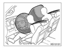
The SRS (Supplemental Restraint System) front airbags are designed to provide further protection for the driver and right front passenger in addition to the primary safety protection provided by the seat belts.
