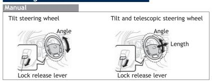
Hold wheel, push lever down, set angle and length, then return lever.
