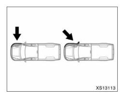
The SRS side airbags and curtain shield airbag system may not activate if the vehicle is subjected to a collision from the side at certain angles, or a collision to the side of the vehicle body other than the passenger compartment as shown in the illustration.
