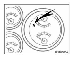
This indicator comes on when the ignition switch is turned to the "ON" position. It goes off after about 6 seconds. This means the SRS airbags are operating properly.
