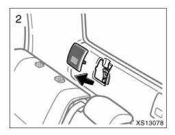
2. Lightly push down on the top surface of the anchor bracket cover, then pull it forward to remove.
