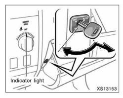
This off switch is designed to disable the front passenger airbag in order to allow usage, if necessary, of a member of a passenger risk group identified in TABLE 1 is occupying the right front passenger seating position. (For details, see "—SRS driver airbag and front passenger airbag" on page 75 in this Section.)
