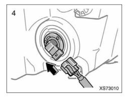
4. Install the connector to the bulb.
