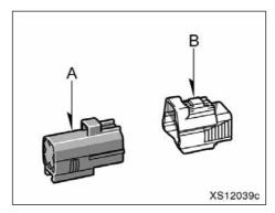
These connector covers are used when removing the tailgate, to prevent the wire harness connectors from being contaminated. Store the connector covers in the glove box in the plastic bag when not using.
