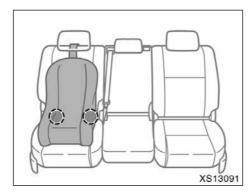
Lower anchorages for the child restraint systems complying with the FMVSS225 or CMVSS210.2 specifications are installed in the front seat.
