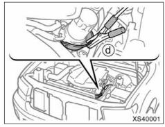
Connecting point for 4.0 L V6 (1GR-FE) engine
