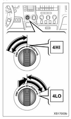
Use the front drive control switch knob to select the following transfer modes. "2WD" (high speed position, two-wheel
