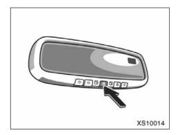
Test the operation of the HomeLink<sup>®</sup> by pressing the newly programmed button. If programming a garage door opener, check to see if the garage door opens and closes.
