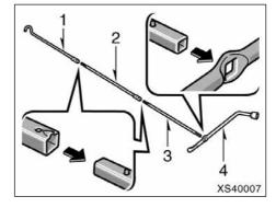
Put a wheel nut wrench, jack handle extension and jack handle end together as shown in the illustration.
