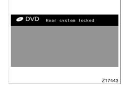
When the rear system lock is on and any button is pushed on the remote controller or the operation panel, the screen shown above is displayed for approximately 6 seconds.
