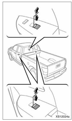
Passenger's door switches (Double cab and Crew Max models)
