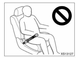
• If the seat belt extender has been connected to the driver's seat belt buckle without the driver actually wearing the seat belt, the SRS driver's airbag system will judge that the driver is wearing it. In this case, the driver's airbag may not activate correctly, causing death or serious injury in the event of collision. Be sure to wear the seat belt with the seat belt extender.
