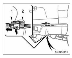
To disconnect the wire harness connectors, press and hold the lock of the connector 1 and pull apart. The connectors are located on the vehicle body frame, behind the bumper.
