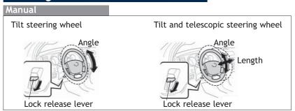
Hold wheel, push lever down, set angle and length, then return lever.
