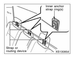
Use the strap or routing device and the inner anchor strap rings to attach the top strap.
