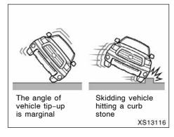
The SRS curtain shield airbags may inflate if the angle of vehicle tip-up is marginal or if the skidding vehicle's tires hit a curb stone laterally as shown in the illustration.
