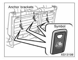
Use the anchor brackets behind the rear seat seatbacks to secure the top strap.
