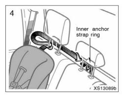
4. Latch the hook onto the inner anchor strap ring and tighten the top strap.
