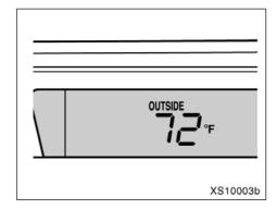
The displayed temperature ranges from  $-40^{\circ}\text{C}$  ( $-40^{\circ}\text{F}$ ) up to  $50^{\circ}\text{C}$  ( $122^{\circ}\text{F}$ ).
