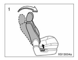
Pull the seatback angle adjusting lever and raise the seatback to its upright position.
