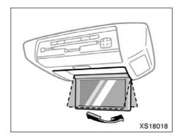
Pull the display down to an easily viewable angle (between 90° and 125°)
