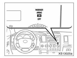
The passenger airbag on-off indicator light indicates the actuation of the front passenger airbag, side airbag on the front passenger seat and front passenger seat belt pretensioner.
