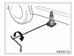
6. After making sure that no one is in the vehicle, raise it high enough so that the temporary spare tire can be installed.
