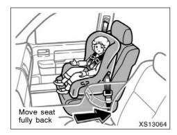
• A forward-facing child restraint system should be allowed to be installed on the front passenger seat only when it is unavoidable. Always move the seat as far back as possible even if the passenger airbag on-off indicator light indicates "OFF", because the front passenger airbag could inflate with considerable speed and force. Otherwise, the child may be killed or seriously injured.
