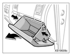
2. Push in each side of the glove box to disconnect the claws.
