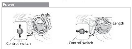
Push the control switch, set angle and length.
