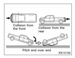
The SRS curtain shield airbags are not generally designed to inflate if the vehicle is involved in a front or rear collision, if it pitches end over end, or if it is involved in a low-speed side collision.
