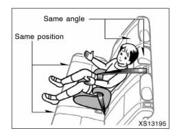
• Crew Max models: When installing a child restraint system in the rear seat center position, adjust both seat cushions to the same position and align both seatbacks at the same angle. Otherwise, the child restraint system cannot be securely restrained and this may cause death or serious injuries in a collision.
