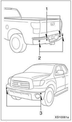
The intuitive parking assist is designed to inform you of the approximate distance between your vehicle and an obstruction by indicator and buzzer when parking the vehicle. This system uses sensors to detect obstructions.
