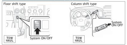
Tow/Haul mode can be used when carrying heavy loads. As fuel economy is reduced while in Tow/Haul mode, deactivating when driving without a load is recommended.
