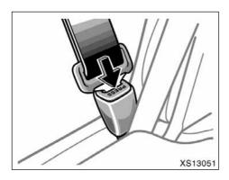
To remove the convertible seat: Press the buckle release button and allow the belt to retract completely. The belt will move freely again and be ready to work for an adult or older child passenger.
