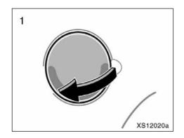
1. To open the fuel filler door, pull the door toward out as shown.
