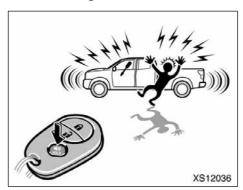
Holding the "(1)" (alarm) switch blows the horn intermittently and flashes the headlights, tail lights, turn signal lights, interior light and personal lights.
