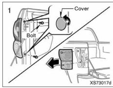
Remove the covers (seal type) and bolts.
