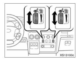
To turn on the seat heater, move the dial upward ("L" dial for the left front seat or "R" dial for the right front seat). At this time, the indicator light will illuminate to indicate the seat heater is operating.
