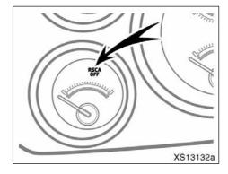
The seat belt pretensioners will not operate in a vehicle rollover if the "RSCA OFF" indicator light is on. For details, see "—Roll sensing of curtain shield airbags off switch" on page 113 in this Section.
