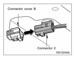
2. Attach the connector cover B (white) to the connector 2.
