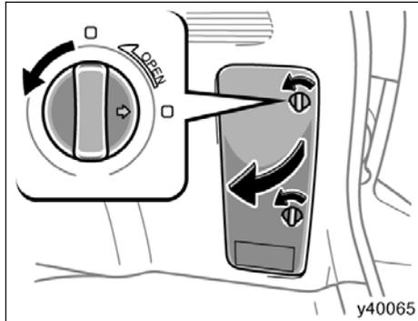
To remove the tools, turn the knob counterclockwise and remove the cover.
