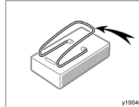
Please note if transmitter has wire clip for sun visor, this clip must be removed prior to adhesion of the fastener.
