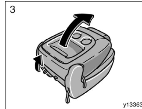
3. Pull the rear leg release lever (red) and swing up the seat.
