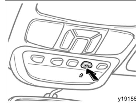
5. Test the operation of the HomeLink® by pressing the newly programmed button. If programming a garage door opener, check to see if the garage door opens and closes.
