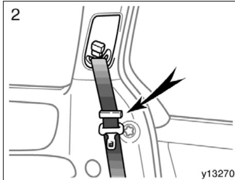
2. Make sure the shoulder belts pass through the hangers when folding the second seat.
