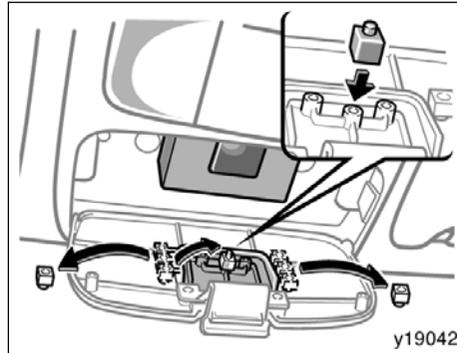
Remove spacers from the center panel. Place one spacer on the pin that would be below transmitter button when the cover is closed. Close the cover.
