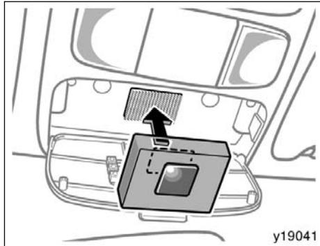
Place the transmitter with the fastener facing inside of box into the box. Make sure the transmitter button is located above button pins.
