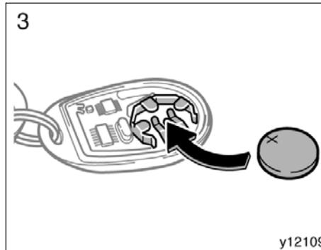
3. Put in a new transmitter battery with positive (+) side up.
