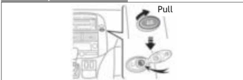
By inserting a mini plug into the AUX audio jack, you can listen to music from a portable audio device through the vehicle’s speaker system.
