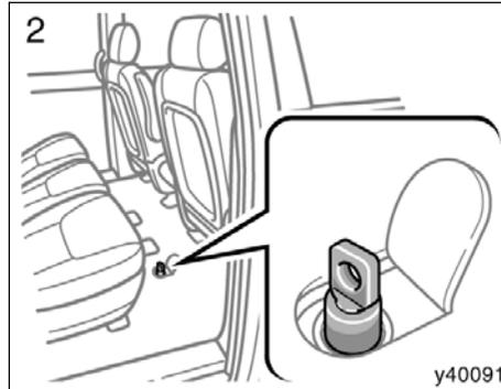
2. Attach the adapter socket over the spare tire clamp bolt.
