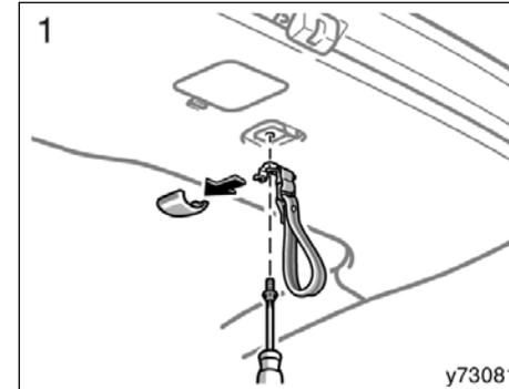
Remove the strap with a Phillips-head screwdriver.
