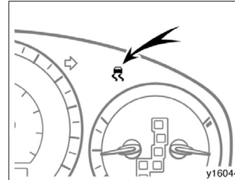
If the vehicle is going to skid during driving, the slip indicator light blinks and an alarm sounds intermittently. Special care should be taken while driving.
