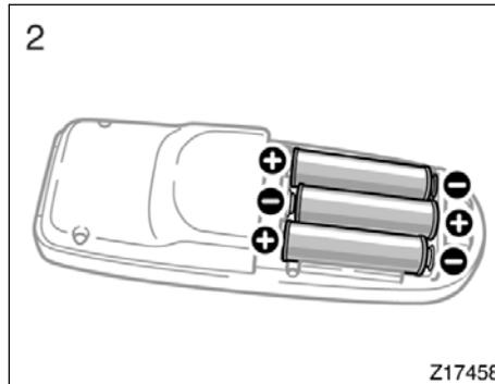
2. Remove the discharged batteries and put in the new batteries as shown. Install the cover.
