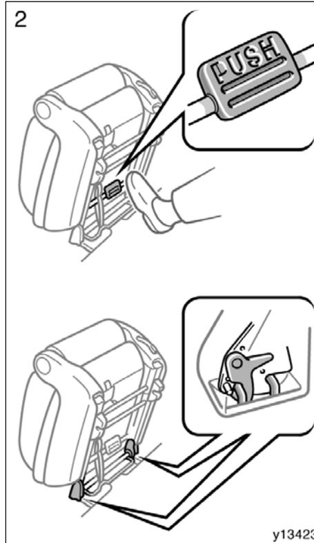
2. Push the foot pedal forward to securely latch the front leg locks. Make sure the front leg is locked securely, fold down the seat and engage the rear leg lock.
