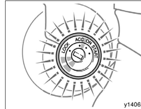
For easy access to the engine switch, the engine switch light comes on when any of the side doors and back door is opened or when the engine switch is turned to the “LOCK” position.
