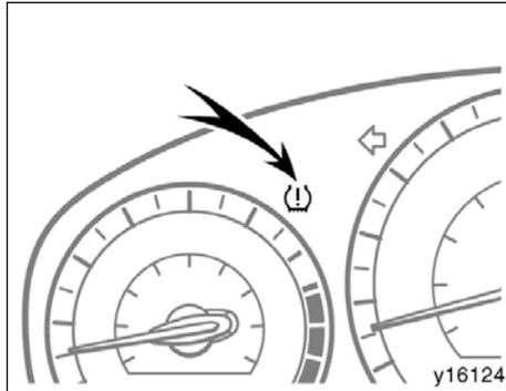
The tire pressure warning light comes on when the engine switch is in "ON" position and goes off after a few seconds. This means the tire pressure warning system is operating properly. If the tire inflation pressure becomes low, the light comes on again. In this case, adjusting the tire inflation pressure will turn off the light after several minutes. If the light comes on after blinking for 1 minute, the tire pressure warning system is not working properly.
