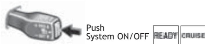
The distance control mode will cruise at a set speed, decelerate to maintain a selected distance from a slower vehicle in front of you, and accelerate back up to the selected speed if the vehicle in front of you changes lanes or speeds up.
