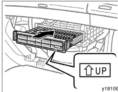
**6. Insert the filter case in the filter outlet, keeping the arrow pointing up.**
