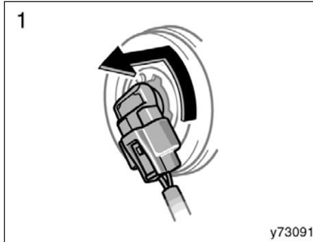
1. Open the hood. Press the bulb base slightly and turn the bulb base counterclockwise to the front of the vehicle as shown.
