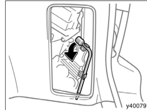
To remove the wheel nut wrench, first disengage the upper part of the wrench from the holding bracket and remove it.
