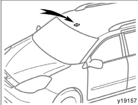
The compass sensor is on the roof of the vehicle.
