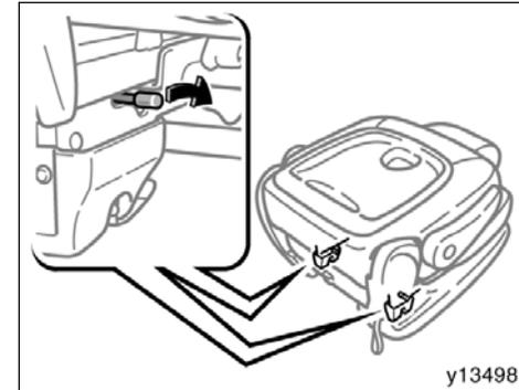
If you lock the rear legs before the front legs are locked securely, disengage the rear leg lock by pushing the red pin inside each rear leg. Then reinstall the seat following the correct procedure.
