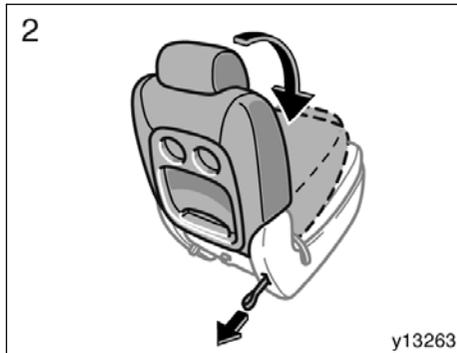
**2. Fold down the seatback while pulling the seatback angle adjusting strap.**
