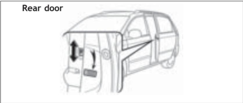
Moving the lever to "LOCK" will allow the door to be opened only from the outside.
