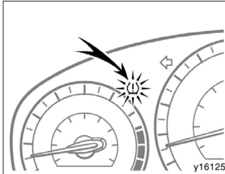
**IF THE TIRE PRESSURE WARNING LIGHT COMES ON AFTER BLINKING FOR 1 MINUTE...**
