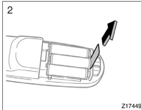
2. Remove the insulating sheet.
