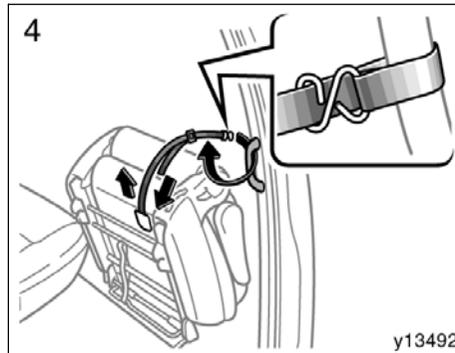
4. Take the holding strap out of the pocket. Pass the strap through the assist grip, and hook it as shown in the illustration.
