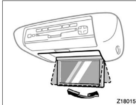
Pull the display down to an easily viewable angle (between 90° and 125°)
