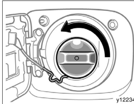
**2. To remove the fuel tank cap, turn the cap counterclockwise. Pause slightly before removing it.**
