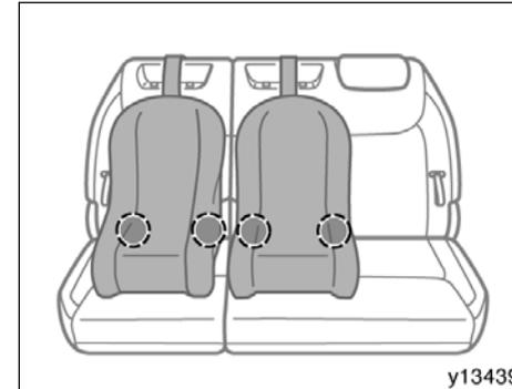
The lower anchorages for the child restraint systems complying with the FMVSS225 or CMVSS210.2 specifications are installed in the rear seat.
