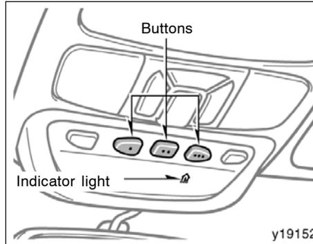
The garage door opener (**HomeLink® Universal Transceiver**) is manufactured under license from HomeLink® and can be programmed to operate garage doors, gates, entry doors, door locks, home lighting systems, and security systems, etc.
