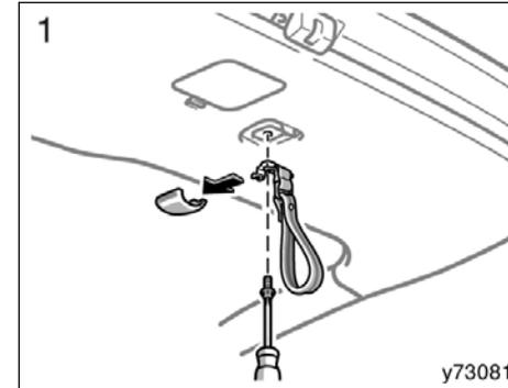
Remove the strap with a Phillips-head screwdriver.
