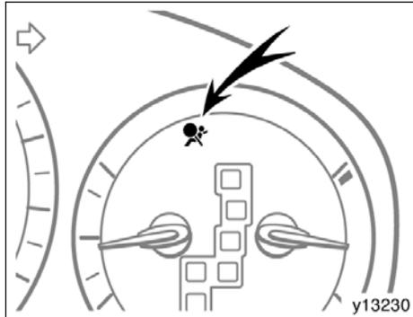
**This indicator comes on when the engine switch is turned to the “ON” position. It goes off after about 6 seconds. This means the SRS front airbags are operating properly.**
