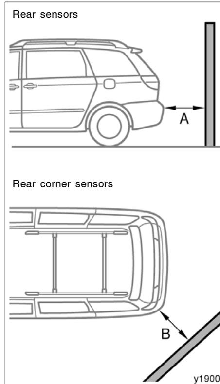
This system is designed to inform you of the approximate distance between your vehicle and an obstacle by indicator and buzzer.
