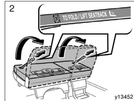
2. Pull the seatback angle adjusting strap (“TO FOLD/LIFT SEATBACK” printed on its surface) and raise the seatback.
