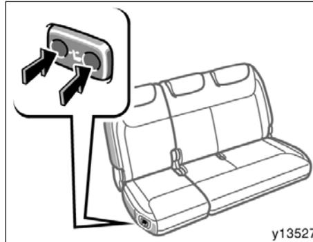
To adjust the seatback angle, push either side of the switch.
