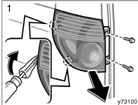
Remove the bolts. Remove the unit by using the flathead screwdriver with cloth.
