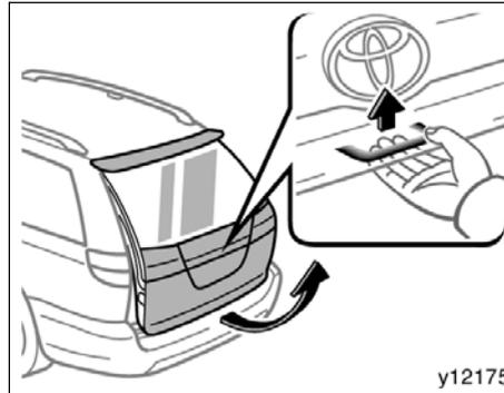
**To open the back door, push up the back door opener and raise the door.**
