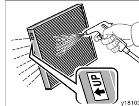
To clean the filter, blow compressed air through it from the bottom.
