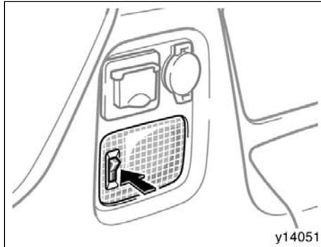
To turn on the luggage compartment light, push the luggage compartment light switch upwards. The light turns on when the personal light main switch is in the “ON” or “DOOR” position.
