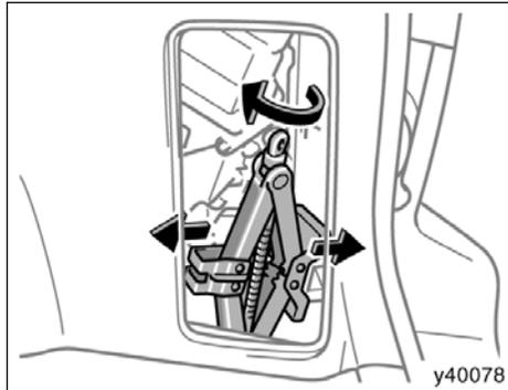
To store the jack, turn the jack joint until the jack base fits securely with the vehicle body.
