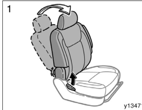
1. Pull the seatback angle adjusting lever and raise the seatback to its upright position.
