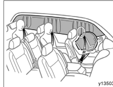
**The SRS (Supplemental Restraint System) side airbags and curtain shield airbags are designed to provide further protection for the driver and all window-side passengers in addition to the primary safety protection provided by the seat belts.**
