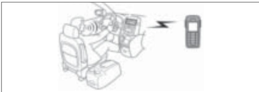
Bluetooth® technology allows dialing or receipt of calls without taking your hands from the steering wheel or using a cable to connect the telephone and the system.
