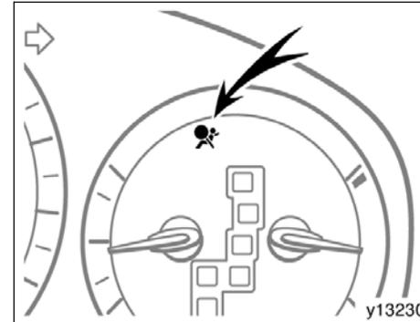
This indicator comes on when the engine switch is turned to the "ON" position. It goes off after about 6 seconds. This means the seat belt pretensioners are operating properly.
