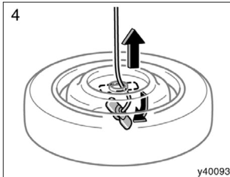
4. After the tire is lowered completely to the ground, remove the holding bracket.
