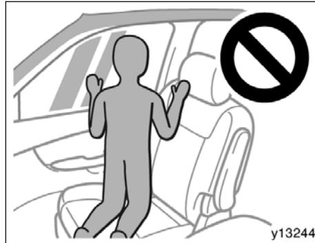
● Do not allow anyone to kneel on the seat facing the side window, since the side airbag and curtain shield airbag could inflate with considerable speed and force. Otherwise, he/she may be killed or seriously injured. Special care should be taken especially when you have a small child in the vehicle.
