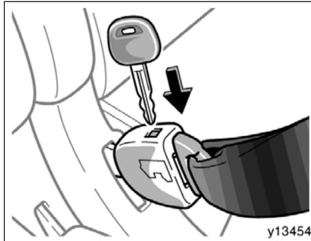
To release the hooked end tab, insert the key into the hole on buckle 1 and allow the belt to retract.
