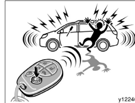
**Pushing and holding the alarm switch blows the horn intermittently and flashes the headlights, tail lights and turns on the front personal lights.**
