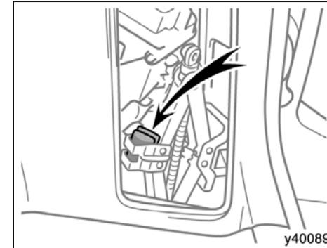
Before removing the jack, take out the adapter socket. The adapter socket is inside a bag and stored in the side of the jack, as shown in the illustration.
