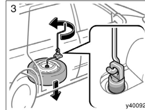
3. Connect the jack handle to the adapter socket. Loosen the spare tire clamp bolt by turning the jack handle counterclockwise.
