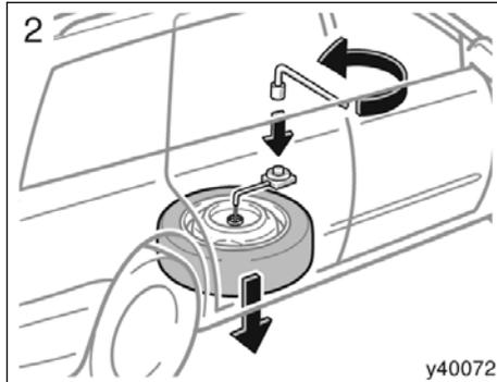
2. Loosen the spare tire clamp bolt by turning it counterclockwise with the wheel nut wrench.
