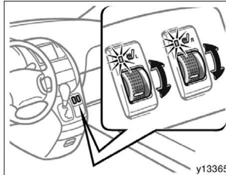
To turn on the seat heater, move the dial upward (“L” dial for the left front seat or “R” dial for the right front seat). At this time, the indicator light will illuminate to indicate the seat heater is operating.
