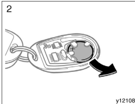
2. Remove the discharged transmitter battery.
