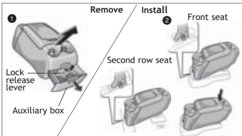
The console box can be removed and installed between the front or second row seats.
