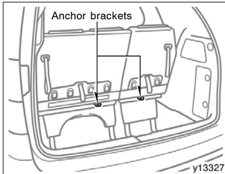
Use the anchor brackets on the back of the third seats to attach the top strap.
