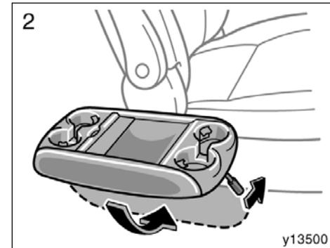
2. For vehicles equipped with the front seat side table, pull up the lock release lever and fold the table down.
