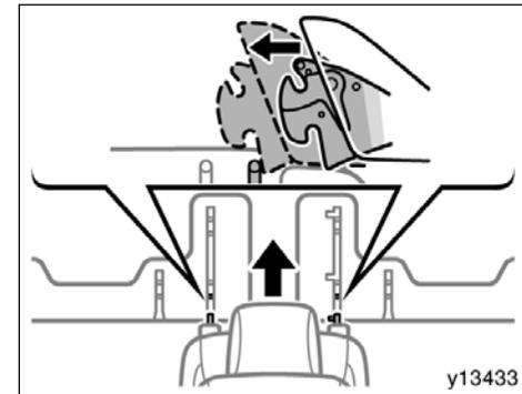
You can easily align the front leg hooks with the rear strikers by using the floor bezel. Put the front legs of the seat short of the rear strikers as shown in the illustration. Then slide the seat forward along the groove of the bezel until the front legs will reach the striker. Make sure the front legs align with the striker, swing up the seat.
