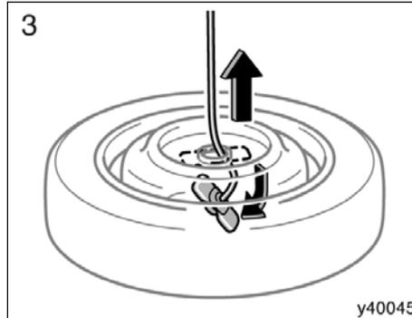
3. After the tire is lowered completely to the ground, remove the holding bracket.
