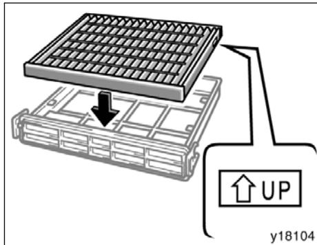
**5. Install the filter to the filter case.**
