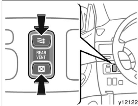
The quarter windows can be operated with the “REAR VENT” switch on the instrument panel.
