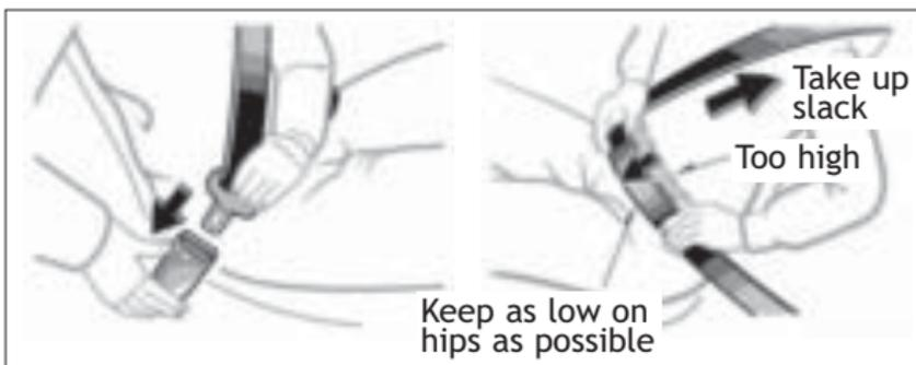
If belt is fully extended, then retracted even slightly, it cannot be re-extended beyond that point, unless fully retracted again. This feature is used to help hold child restraint systems securely.
