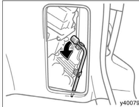
To remove the wheel nut wrench, first disengage the upper part of the wrench from the holding bracket and remove it.
