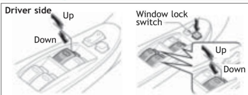
**Automatic operation\* (driver side only)** Push the switch completely down or pull it completely up and release to fully open or close. To stop window midway, lightly push the switch in the opposite direction.
