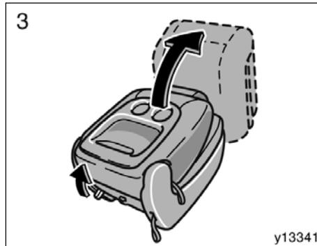
**3. Pull the seat lock release lever (red) and swing up the seat.**
