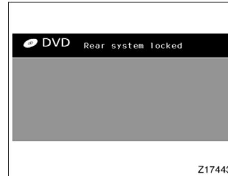
When the rear system lock is on and any button is pushed on the remote control or the operation panel, the screen shown above is displayed for approximately 6 seconds.
