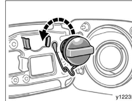
**3. The removed cap can be hanged on the cap hanger.**
