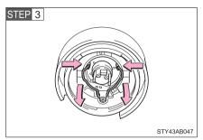
Release the bulb retaining spring.
