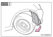
Partly remove the fender liner.
