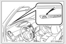
The indicator light flashes after the key has been removed from the engine switch to indicate that the system is operating.
