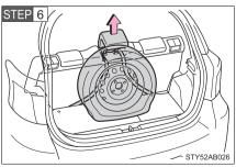
Lay the flat tire on the luggage floor so that the outer side of the tire wheel faces toward the rear of the vehicle. Detach the rear center head restraint from the seat and release the belt.
