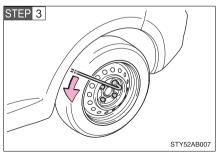
Slightly loosen the wheel nuts (one turn).
