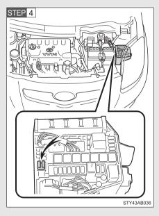
Remove the fuse with the pullout tool.
