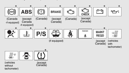
\*: These lights turn on when the engine switch is turned to the ON position to indicate that a system check is being performed. They will turn off after the engine is started, or after a few seconds. There may be a malfunction in a system if a light does not come on, or if the lights do not turn off. Have the vehicle inspected by your Toyota dealer.
