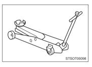
1 Lift up the vehicle using a floor jack such as the one shown in the illustration.
