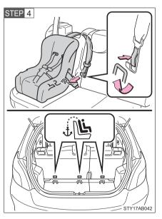
Latch the hook onto the anchor bracket and tighten the top strap.
