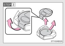
Remove the battery cover and the depleted battery.
