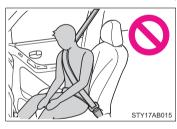
1 Vehicles with side airbags and curtain shield airbags: Do not lean against the door, the roof side rail or the front, side and rear pillars.
