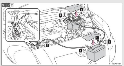
Connecting the jumper cables
