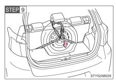
Hold the buckle and pull the belt to secure the tire.
