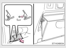
2.Pull up the box and disengage the claws. Remove the stoppers from the cutouts and remove the box.
