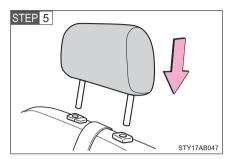
Non-split rear seat only: Reinstall the head restraint
