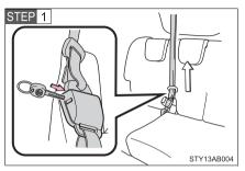
Insert the key into the hole on the center seat belt buckle to release tub (with hooked end), and allow the belt to retract.
