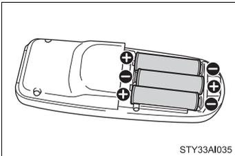
Remove the depleted batteries and install 3 new AA batteries.
