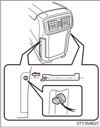
Reinstall it in a horizontal direction as indicated in the illustration. It cannot be installed in any other direction.
