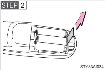
Remove the insulating sheet.
