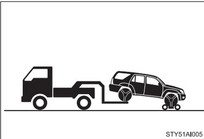
Full-time 4WD models: Use a towing dolly under the front wheels.
