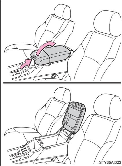
Pull up the console box lid while pushing the lock release button.
