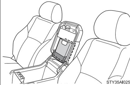
Pull up the console box lid while pushing the lock release button.
