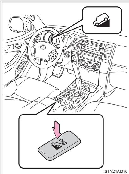
Press the DAC switch. The downhill assist control indicator will come on, and the system will operate.
