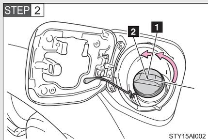
To remove the fuel tank cap, turn the cap counterclockwise by 90 degrees ( **1** ), and then turn it an additional 30 degrees ( **2** ). Pause slightly before removing it.
