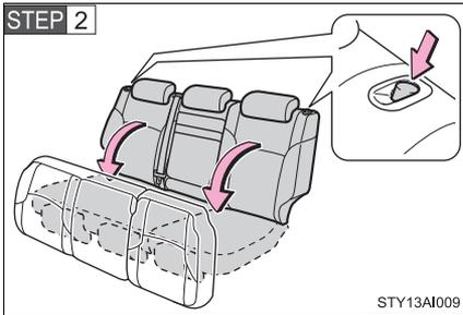
Push the lock release button and fold down the seatback.
