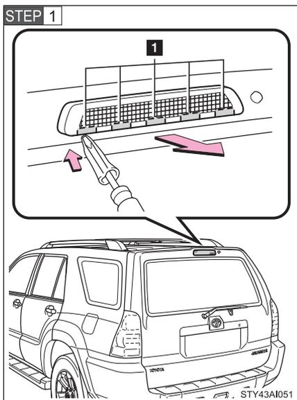
Disconnect the clips by using a flathead screwdriver which is wrapped with a cloth.
