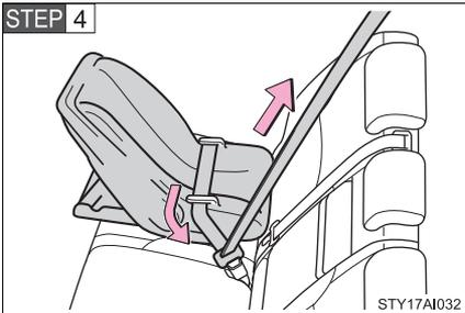
While pushing the child seat down into the rear seat, allow the shoulder belt to retract until the child seat is securely in place.
