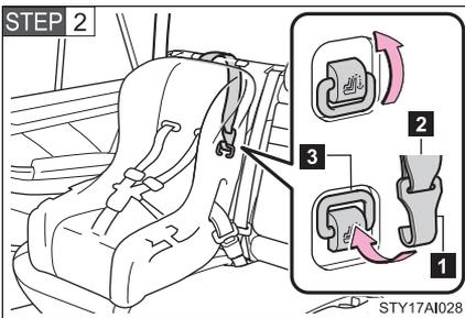
Raise the anchor bracket, latch the hook onto the anchor bracket and tighten the top tether strap.
