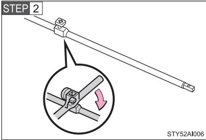
When connecting the jack handle extensions, use the jack handle to tighten the square head bolt. Make sure that the bolt fits into the depression on the joint.
