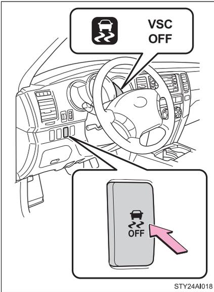
Stop the vehicle completely, and press the VSC OFF switch for more than 3 seconds.
