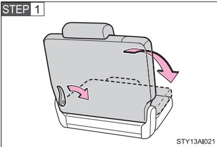
Fold down third seat by pushing the lock release lever forward.
