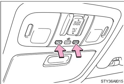
Press and hold down the 2 outside buttons for 20 seconds until the indicator flashes.
