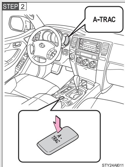
Press the A-TRAC switch to activate the system.
