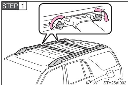
Turn the knobs counterclockwise to loosen the cross rails.
