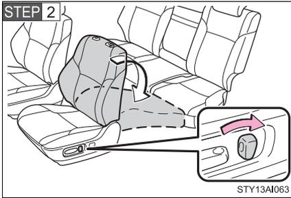
Move the seatback angle adjustment switch backward to flatten the seatback.
