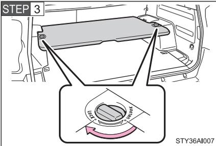
Turn the knobs to the LOCK position.
