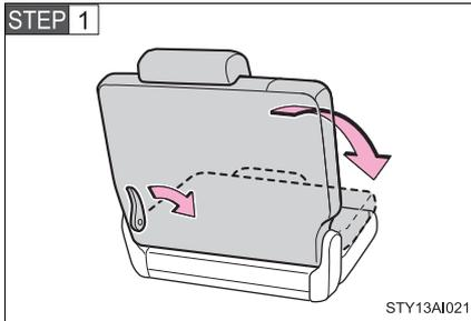
Fold down the third seat by pushing the lock release lever forward.
