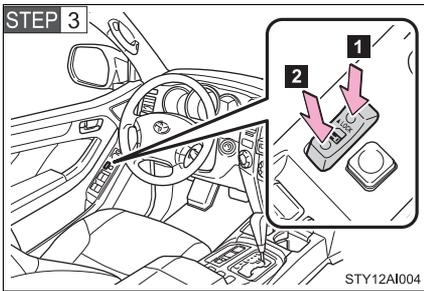
Shift the shift lever to P or N, press and hold the driver's door lock switch (**1** or **2**) for approximately 5 seconds and then release.
