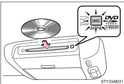
Insert the disc into the slot with the label side up.
