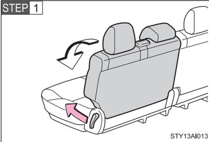
Pull the lever to unlock the seat-back and then fold the seatback down.
