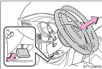
**STEP 1** Hold the steering wheel and press the lever down.
