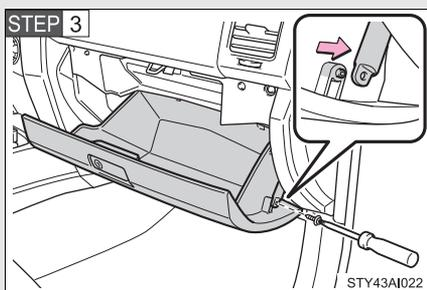
Remove the screw with a Phillips-head screwdriver and slide off the damper.
