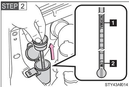
Check the washer fluid level on the level gauge.
