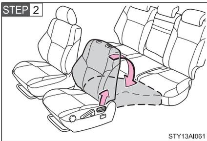
Pull the seatback angle adjustment lever to unlock the seatback and then push down the seatback.
