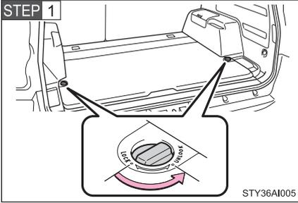
Turn the knobs to the UNLOCK position.
