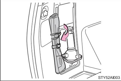
Remove the cover and loosen the strap.
