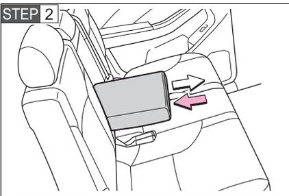
To open, press in and release the cup holder on the armrest.
