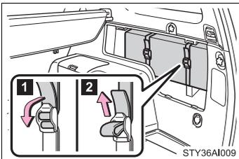
**1** To loosen: Pull the buckle forward.
