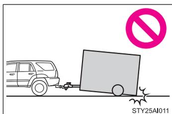
No matter which class of tow hitch applies, for a safe trailer hookup, the trailer ball setup on must be the proper height for the coupler on the trailer.
