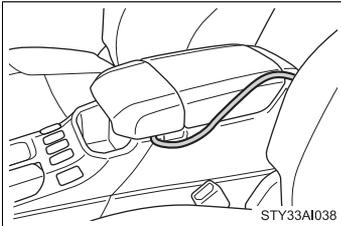
Let it go through the gap between the console box and the tray. Use a cord which is thin enough to go through the gap. Close the console box lid.
