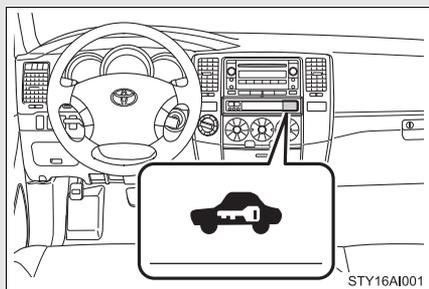
Close the doors and hood, and lock all doors using the wireless remote control or key. The system will be set automatically after 30 seconds.
