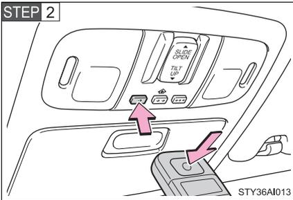
Press and hold down one of the buttons on the HomeLink<sup>®</sup> and the button on the transmitter. When the indicator on the HomeLink<sup>®</sup> changes from a slow to a rapid flash after 20 seconds, you can release both buttons.
