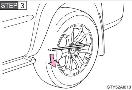
Slightly loosen the wheel nuts (one turn).
