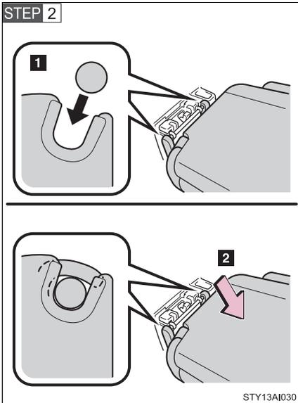
**1** Hold the seat and engage the seat striker to the seat lock, then place the seat on the floor.
