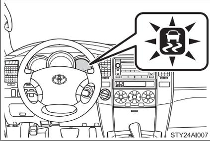
If all wheels spin, the slip indicator flashes to indicate that the active traction control system have been engaged.
