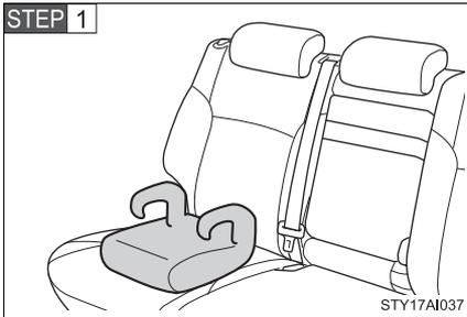
Place the booster seat on the seat facing the front of the vehicle.
