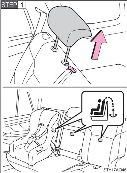
Secure the child restraint using the LATCH anchors or seat belt, and remove the head restraint.
