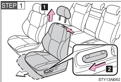
**1** Remove the head restraint.
