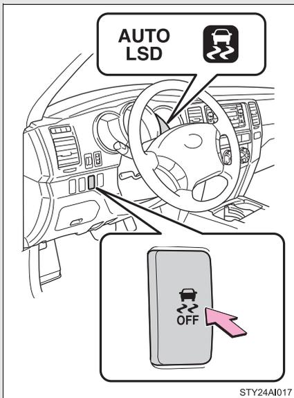
Press the VSC OFF switch to turn on the system.
