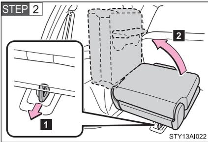
1 Unlock the seat leg by pulling the handle.
