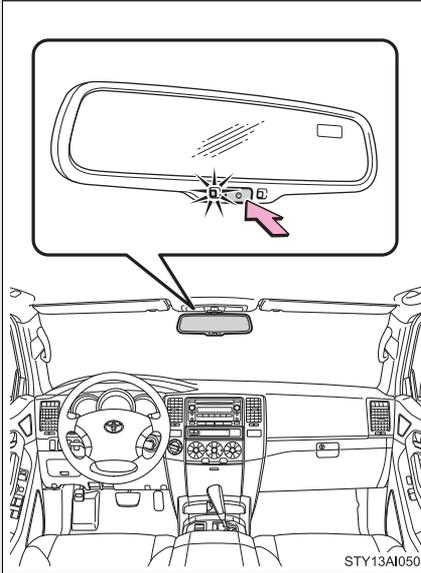
Press the button for longer than 3 seconds to turn auto mode ON/OFF.
