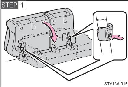
Push the knob to unlock the seat and swing the whole seat down.
