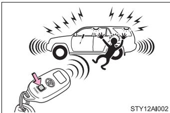
When PANIC switch is pushed for longer than about one second, an alarm will sound for about 60 seconds and the vehicle lights will flash to deter any person from trying to break into or damage your vehicle.
