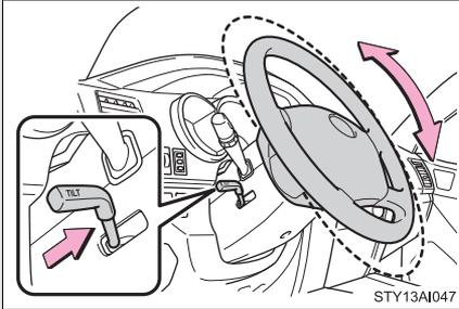
**STEP 1** Hold the steering wheel and pull the lever.
