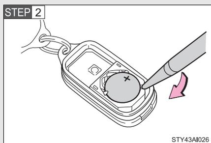
Remove the depleted battery.
