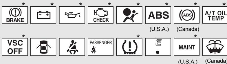
\*: These lights turn on when the engine switch is turned to the ON position to indicate that a system check is being performed. They will turn off after the engine is started, or after a few seconds. There may be a malfunction in a system if a light does not come on, or if the lights do not turn off. Have the vehicle inspected by your Toyota dealer.
