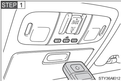
Point the remote control transmitter for the device 1 to 3 in. (25 to 75 mm) from the HomeLink<sup>®</sup> control buttons.
