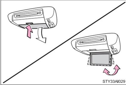
Press the lock release button to open the display.
