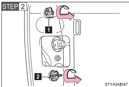
Turn the bulb bases counter-clockwise.
