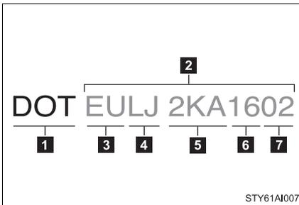
**1** DOT symbol\***2** Tire Identification Number (TIN)**3** Tire manufacturer's identification mark**4** Tire size code**5** Manufacturer's optional tire type code (3 or 4 letters)**6** Manufacturing week**7** Manufacturing year
