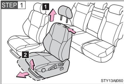
**1** Remove the head restraint.
