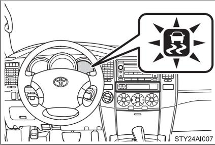
If the vehicle is in danger of slipping, the rear wheels (2WD models) or four wheels (4WD models) spin, the vehicle starts to roll backwards when starting on an incline, the slip indicator flashes to indicate that the VSC/TRAC/A-TRAC/hill-start assist control have been engaged.
