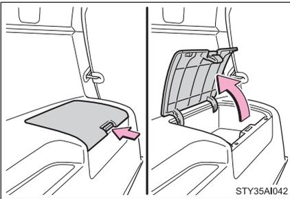
Push the knob to release the lock. Lift the lid.
