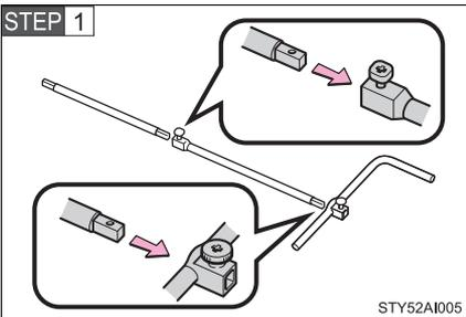
Assemble the jack handle extension as shown. Be sure to tighten each bolt securely.
