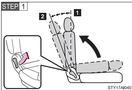
**STEP 1** Fold the seatback while pulling the lever. Return the seatback and secure it at the 1st lock position (most upright position). Adjust the seatback to the 5th lock position. (→P. 44)
