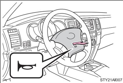
To sound the horn, press on or close to the
