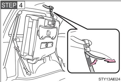
Pull the free end of the strap then fix it with the hook-and-loop fastener.
