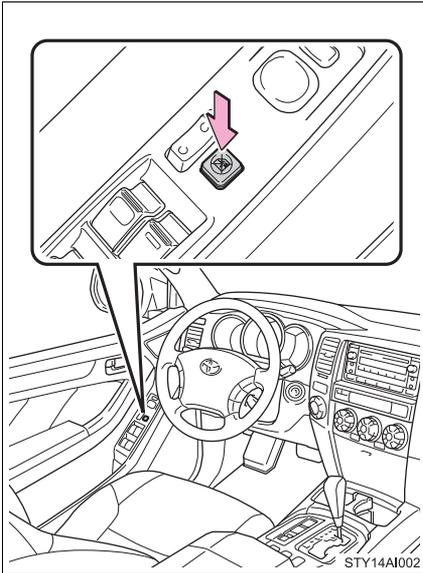
Press the switch down to lock passenger window switches and back window switch.
