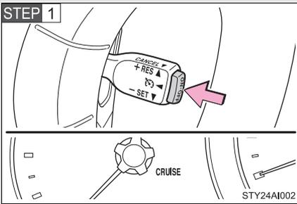
Press the ON-OFF button to turn the cruise control on.
