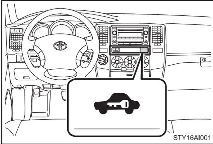
The indicator flashes after the key has been removed from the engine switch to indicate that the system is operating.
