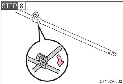
When connecting the jack handle extension(s) and jack handle end, use the jack handle to tighten the square head bolt. Make sure that the bolt fits into the depression on the joint.
