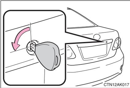
Turn the master key (vehicles without smart key system) or mechanical key (vehicles with smart key system) counterclockwise to lock the trunk opener feature.
