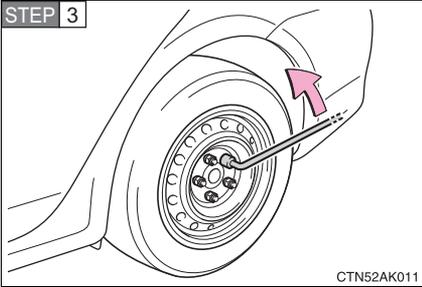
Slightly loosen the wheel nuts (one turn).
