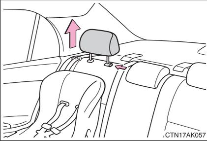
Remove the head restraint.
