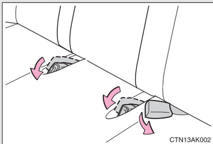
Stow the rear outside seat belt buckles and move the rear center seat belt buckle as shown.
