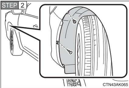
Remove the fender liner clips.
