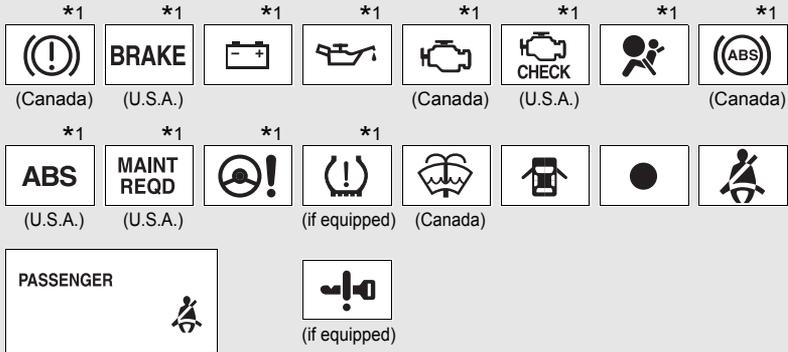
\*1: These lights turn on when the “ENGINE START STOP” switch is turned to IGNITION ON mode (vehicles with smart key system) or the engine switch is turned to the “ON” position (vehicles without smart key system) to indicate that a system check is being performed. They will turn off after the engine is started, or after a few seconds. There may be a malfunction in a system if a light does not come on, or if the lights do not turn off. Have the vehicle inspected by your Toyota dealer for details.
