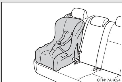
Seat belts equipped with a child restraint locking mechanism (ALR/ELR belts except driver's seat belt) (→P. 53)
