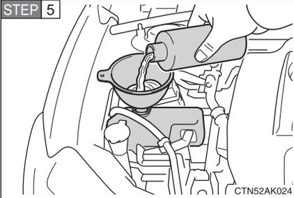
Add engine coolant if necessary.
