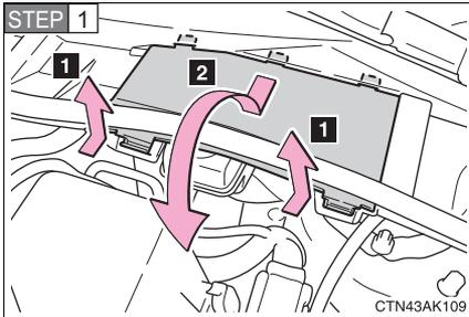
Disconnect the claws to remove the service cover as shown in the illustration.
