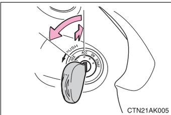
**STEP 1** Shift the shift lever to P (automatic transmission) or N (manual transmission).
