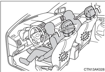
When a front seatback receives a strong impact, the head restraint moves slightly forward to help reduce the risk of whiplash on the seat occupant.
