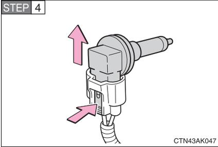
Unplug the bulb while depressing the lock release.
