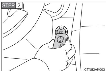
Touch the Toyota emblem side of the electronic key to the “ENGINE START STOP” switch.
