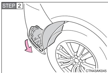
Partly remove the fender liner.
