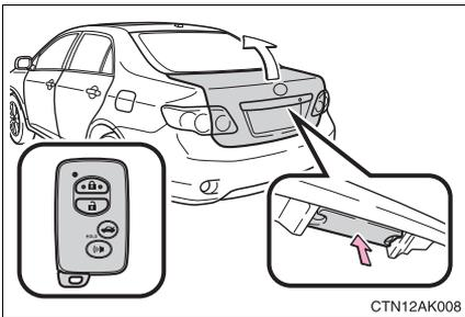
Press the button to unlock the trunk.
