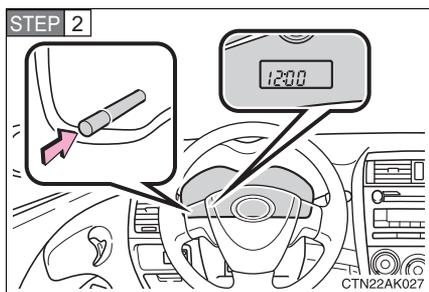
Press and hold the display button to enter the adjustment mode for the clock.
