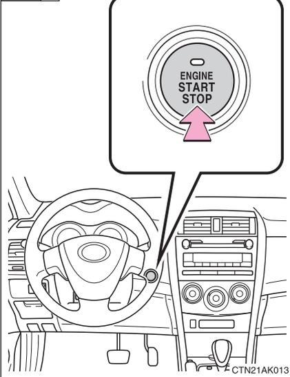
Press the “ENGINE START STOP” switch.
