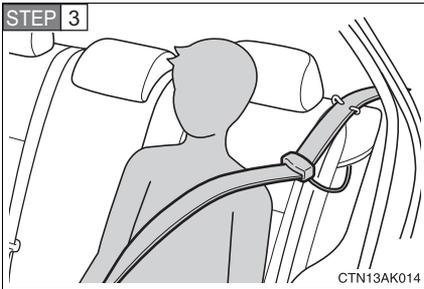
Buckle, position and release the seat belt.
