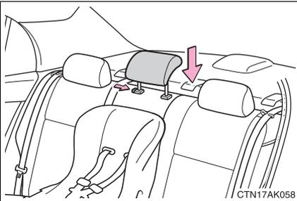
Lock the head restraint in place at the lowest position.
