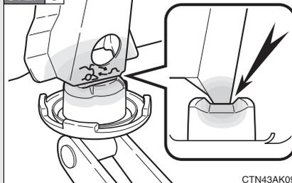
Before raising the vehicle, make sure that the floor jack is positioned so that the jack point fits securely inside the groove on the jack attachment.
