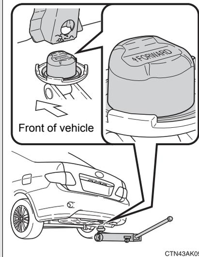
Set the jack attachment on the floor jack with the “FORWARD” facing towards the front of the vehicle, and place the jack.
