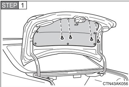
Open the trunk lid and remove the trunk panel cover clips.
