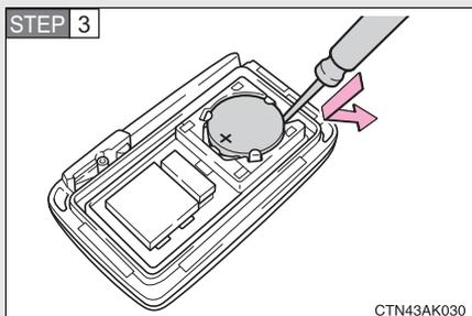
Remove the depleted battery.
