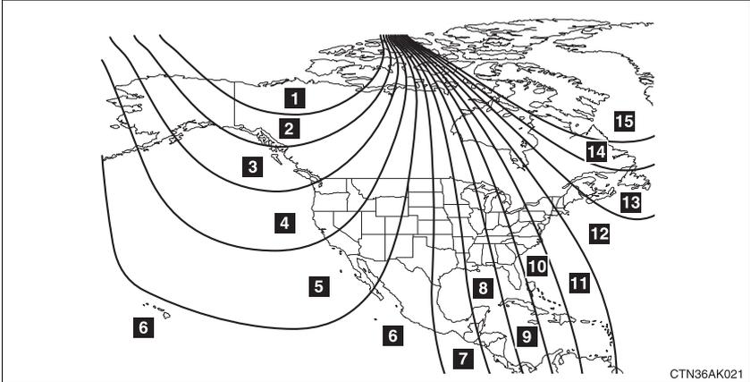
The direction display deviates from the true direction determined by the earth's magnetic field. The amount of deviation varies according to the geographic position of the vehicle.
