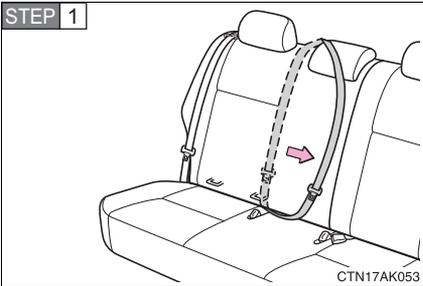
Rear right seat only: Slide the rear center seat belt to the side to prevent it from getting pinched in the lower anchorage.
