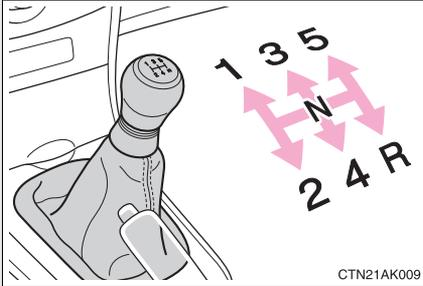
Fully depress the clutch pedal before operating the shift lever, and then release the clutch pedal slowly.
