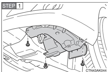
Remove the fender liner bolts and clip.
