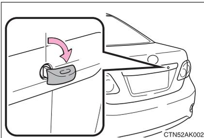
Turn the mechanical key clockwise to open.
