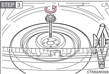
Loosen the center fastener that secures the spare tire.
