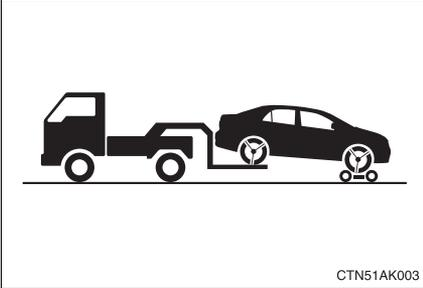
Automatic transmission: Use a towing dolly under the front wheels.
