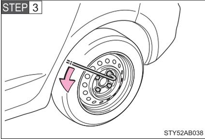
Slightly loosen the wheel nuts (one turn).
