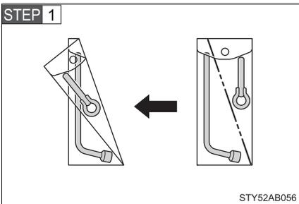
Position the tools as shown in the illustration. Fold the tool bag over.
