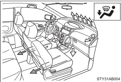
When the dial is set to
