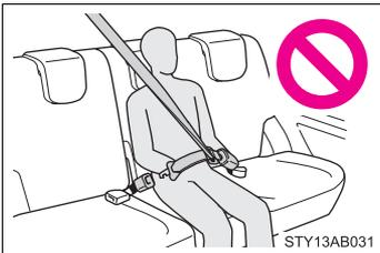
Do not use the rear center seat belt with either buckle released. Fastening only one of the buckles may result in death or serious injury in case of sudden braking or a collision.
