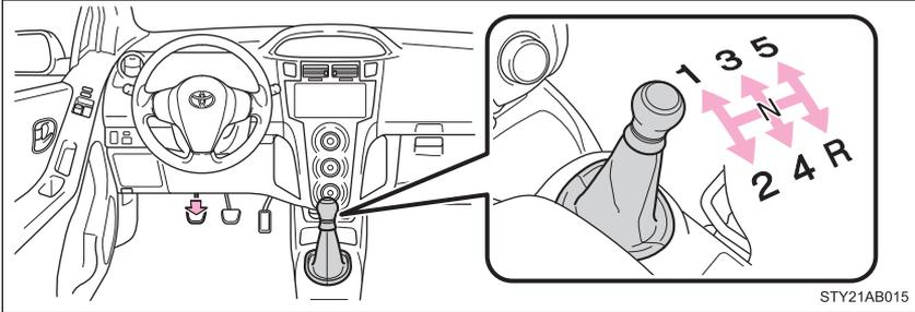
Fully depress the clutch pedal before operating the shift lever, and then release it slowly.
