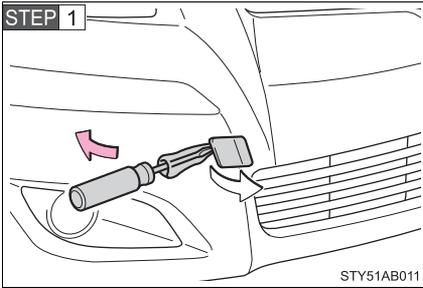
Remove the eyelet cover using a flathead screwdriver.
