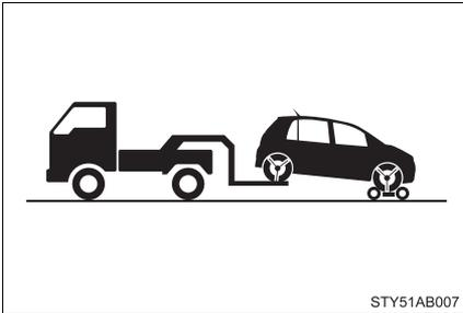
Vehicles with an automatic transmission: Use a towing dolly under the front wheels.
