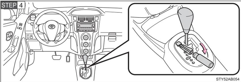
Pry the cover up with a flathead screwdriver or equivalent.
