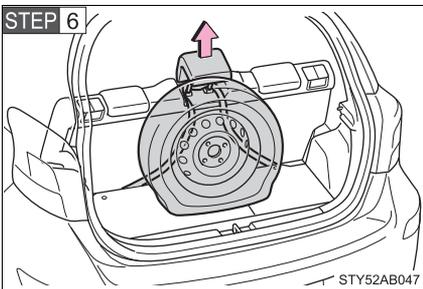
Lay the flat tire on the luggage floor so that the outer side of the tire wheel faces toward the rear of the vehicle. Detach the rear center head restraint from the seat and release the belt.
