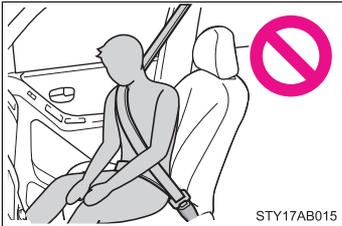
**I** Vehicles with side airbags and curtain shield airbags: Do not lean against the door, the roof side rail or the front, side and rear pillars.
