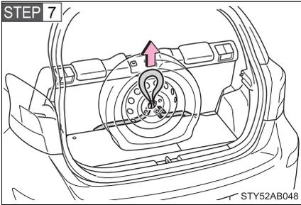
Pass the belt through the center hole of the flat tire wheel.
