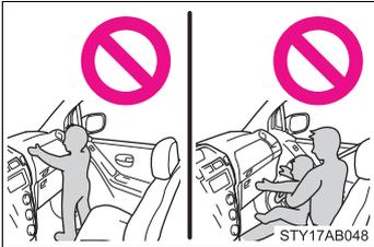
**I** Do not allow a child to stand in front of the SRS front passenger airbag unit or sit on the knees of a front passenger.
