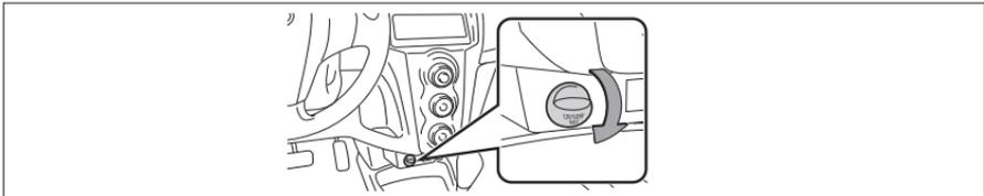
Designed for 12V car accessories. Key must be in the "ACC" or "ON" position to be used.
