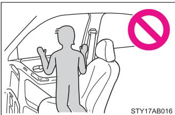
**I** Vehicles with side airbags and curtain shield airbags: Do not allow anyone to kneel on the passenger seat toward the door or put their head or hands outside the vehicle.
