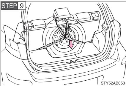
Hold the buckle and pull the belt to secure the tire.
