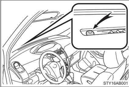
**STEP 1** Close the doors and hood, and lock all doors using the key.
