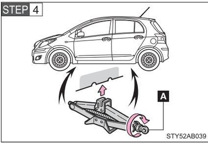
Turn the jack portion "A" by hand until the notch of the jack is in contact with the jack point.
