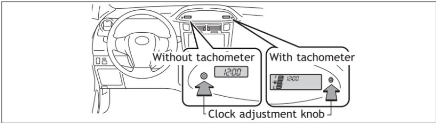
Press and hold clock reset button for adjustment mode. Press again to adjust minutes and hours, waiting 5 seconds after each.
