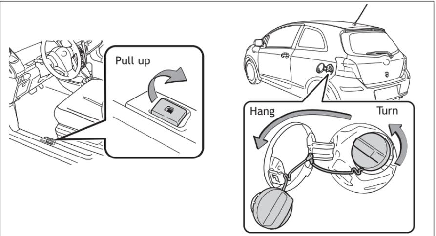
**NOTE:** Tighten until one click is heard. If the cap is not tightened enough, Check Engine “
