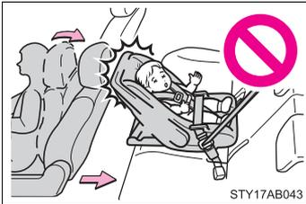
ⓘ If the driver's seat interferes with the child restraint system and prevents it from being attached correctly, attach the child restraint system to the right-hand rear seat.
