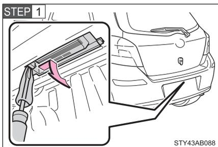
Disengage the claws and remove the license plate light.
