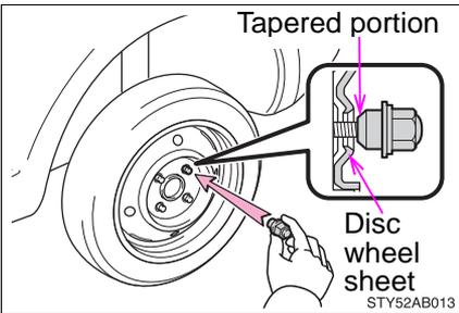
Tighten the nuts until the tapered portion comes into loose contact with the disc wheel sheet.
