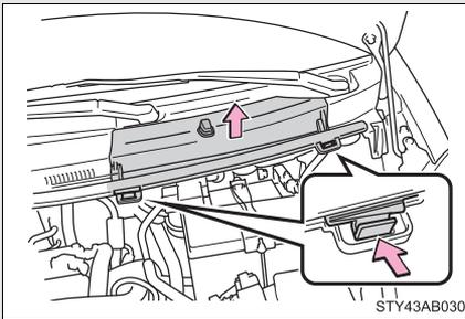
1. Push the tab in and lift the cover off.
