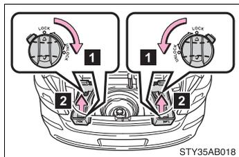
**1** Turn the knobs to the UNLOCK position.
