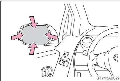
Adjust the mirror up, down, in or out by pushing the mirror surface.
