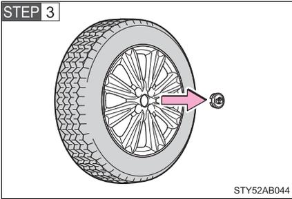
Vehicles with an aluminum wheels, remove the center wheel ornament by pushing from the reverse side.
