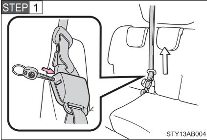
Insert the key into the hole on the center seat belt buckle to release tab (with hooked end), and allow the belt to retract.
