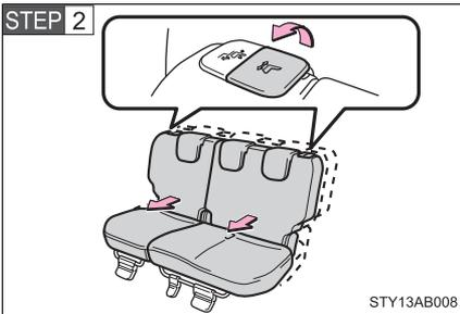
Pull the seat position adjustment lever up. Then slide the rear seat fully forward.
