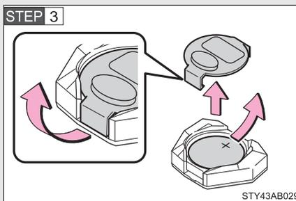
Remove the battery cover and the depleted battery.
