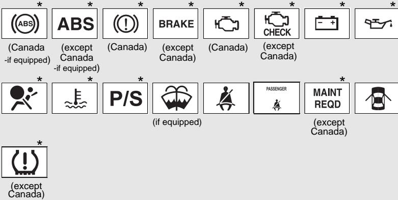
\*: These lights turn on when the engine switch is turned to the ON position to indicate that a system check is being performed. They will turn off after the engine is started, or after a few seconds. There may be a malfunction in a system if a light does not come on, or if the lights do not turn off. Have the vehicle inspected by your Toyota dealer.
