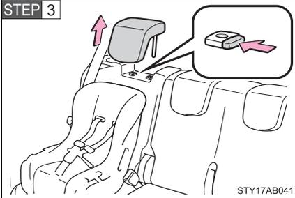
Remove the head restraint.
