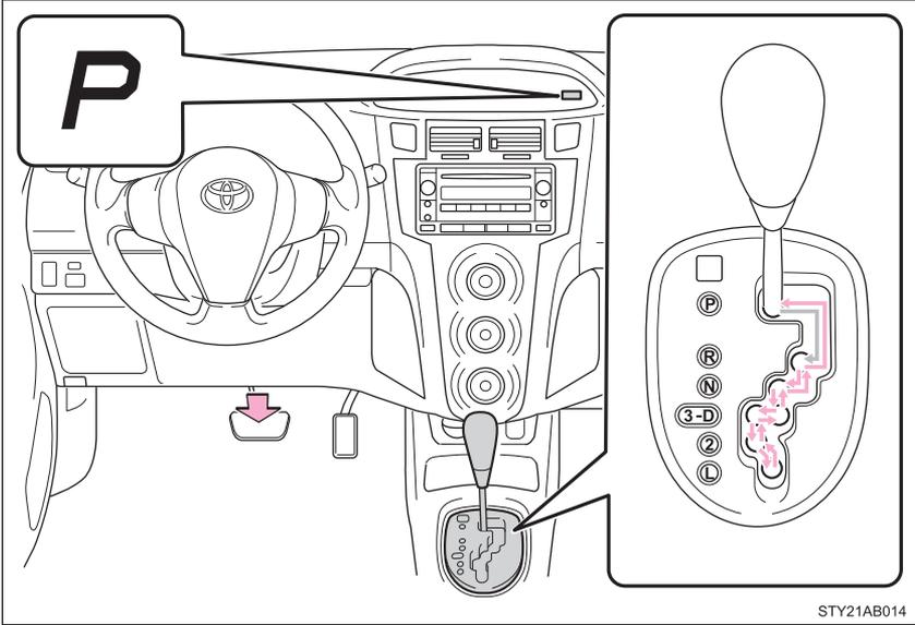
← While the engine switch is on, depress the brake pedal and move the shift lever.
