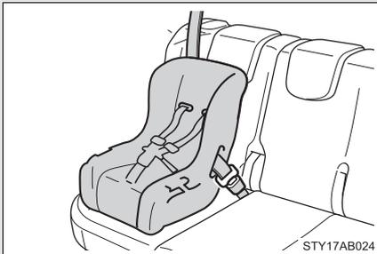
Seat belts equipped with a child restraint locking mechanism (ALR/ELR belts except driver's seat belt) (→P. 52)
