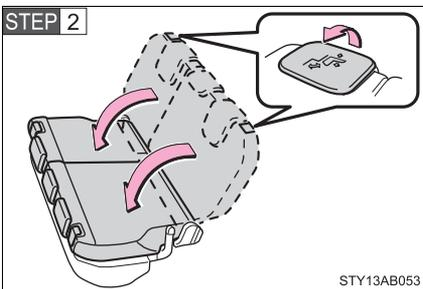
Pull the seatback angle adjustment lever up and fold the seatback down.
