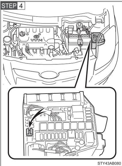
Remove the fuse with the pull-out tool.
