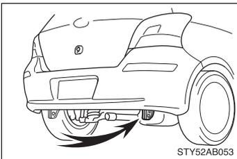
When your vehicle becomes stuck and cannot move, the emergency hook is used for another vehicle to pull your vehicle out in an emergency.
