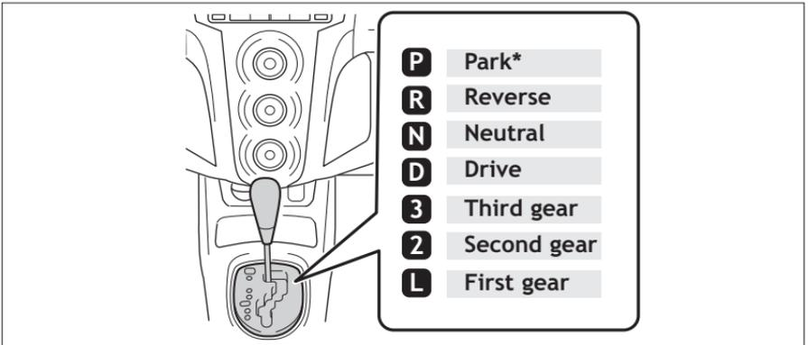
\* The ignition switch must be “ON” and the brake pedal depressed to shift from Park.
