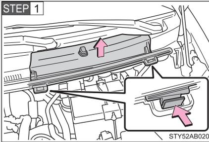
Push the tab in and lift the cover off.
