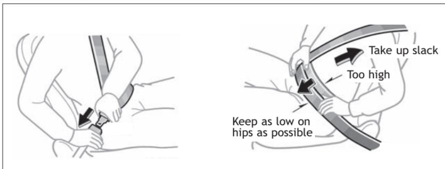
If belt is fully extended, then retracted even slightly, it cannot be re-extended beyond that point, unless fully retracted again. This feature is used to help hold child restraint systems securely.
