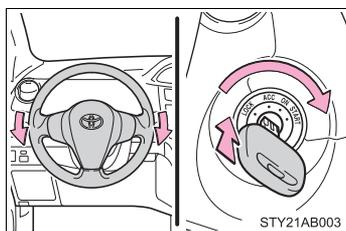
When starting the engine, the engine switch may seem stuck in the LOCK position. To free it, turn the key while turning the steering wheel slightly in either direction.
