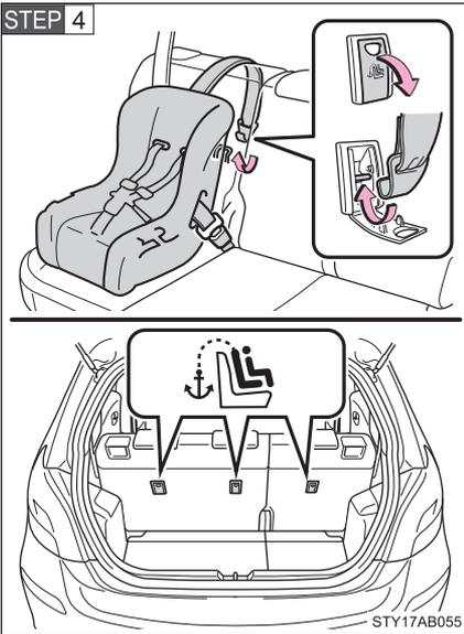
Latch the hook onto the anchor bracket and tighten the top tether strap.
