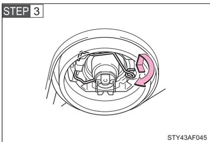
Release the bulb retaining spring.
