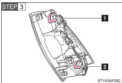
Turn the bulb bases counter-clockwise.
