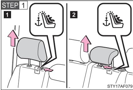
Remove the head restraint.
