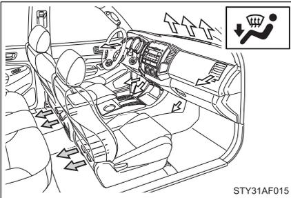
When the dial is set to
