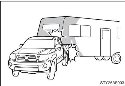
When towing a fifth wheel trailer, be careful not to hit the cabin or deck by the trailer while making a sharp turn.
