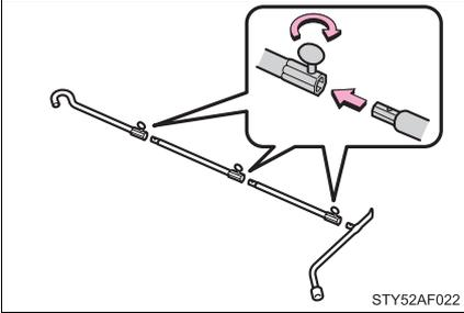
Assemble the jack handle extension as shown. Be sure to tighten each screw securely.
