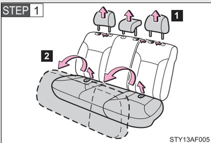
1 Remove the head restraint
