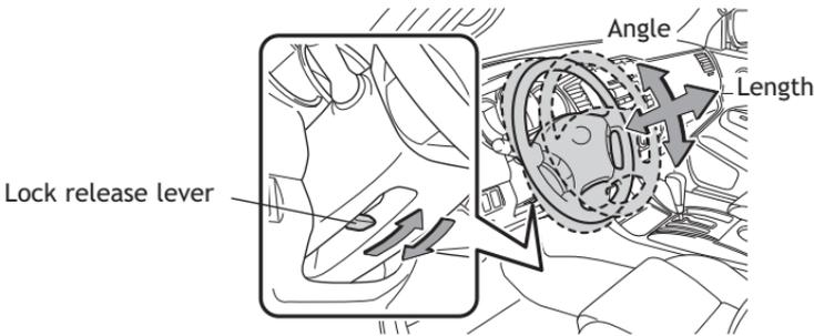
Hold wheel, push lever down, set angle and length, and return lever.
