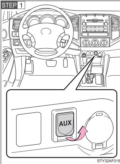
Connect the portable audio device.
