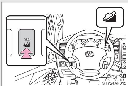
Press the DAC switch. The indicator will come on, and the system will operate.
