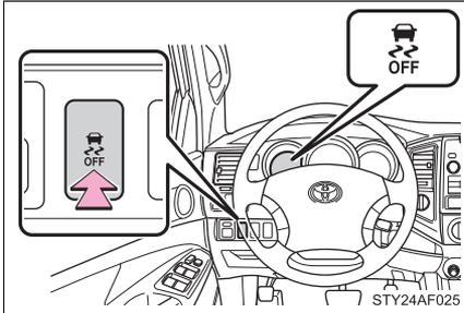
Press and hold the VSC OFF switch for more than 3 seconds while the vehicle is stopped to turn off both TRAC and VSC.
