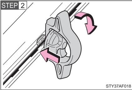
Insert the locking plate into the deck rail, rotate the tie-down cleat 90°, and release the thumb wheel.
