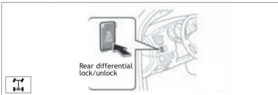
Use **ONLY** when wheel spinning occurs in a ditch, or on slippery or unpaved surfaces. **DO NOT USE THE REAR DIFFERENTIAL LOCK IN CONDITIONS OTHER THAN THOSE SPECIFIED IN THE OWNER'S MANUAL.** UNLOCK THE DIFFERENTIAL ONCE THE VEHICLE MOVES OUT OF THE TROUBLE SPOT.
