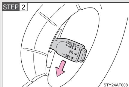
Accelerate or decelerate to the desired speed and push the lever down to set the cruise control speed.
