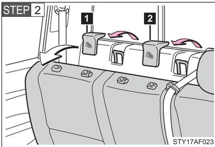
Swing the seatback forward slightly (→P. 46) and remove the anchor bracket covers.
