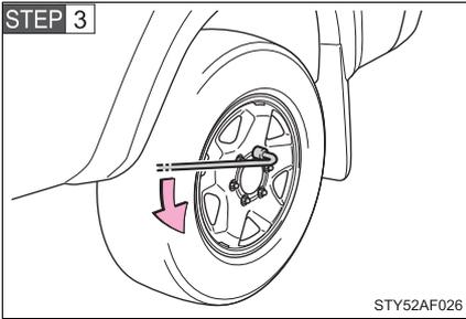
Slightly loosen the wheel nuts (one turn).
