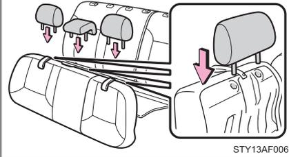
Attach the head restraints to the holders located on the back sides of the bottom cushions.
