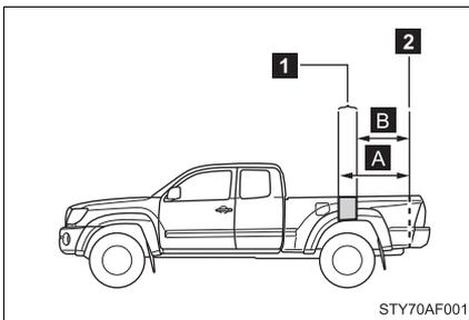
**1** Recommended location for cargo center of gravity for cargo weight rating
