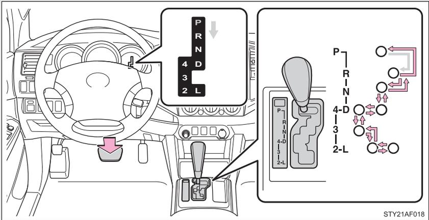
← While the engine switch is on, depress the brake pedal and move the shift lever.
