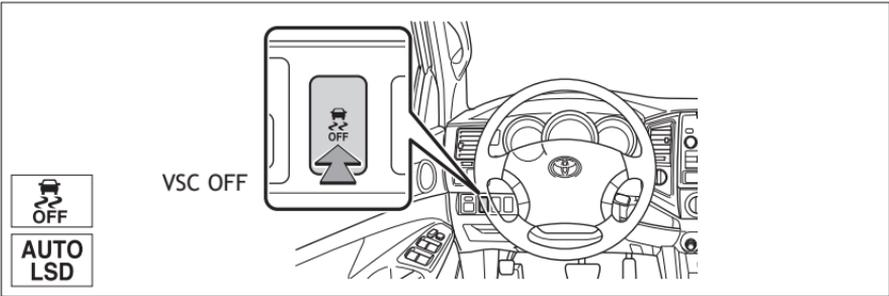
The VSC OFF button is used to switch between modes related to the TRAC, VSC and Auto LSD functions.
