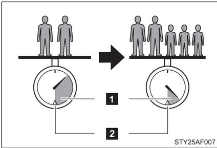
When 2 people with the combined weight of A lb. (kg) are riding in your vehicle, which has a total load capacity of B lb. (kg), the available amount of cargo and luggage load capacity will be C lb. (kg) as follows:
