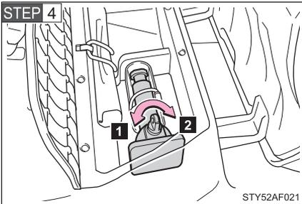
Loosen and remove the jack.
