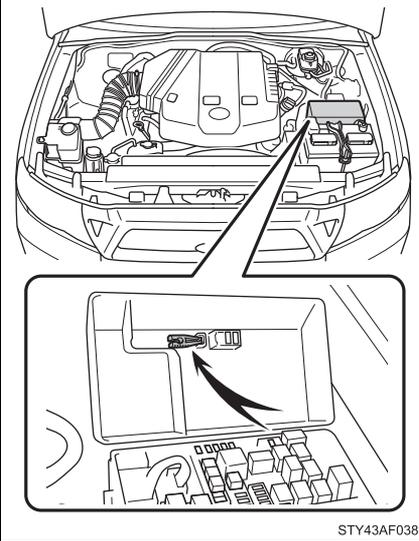
Remove the fuse with the pull-out tool.
