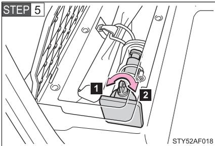
Loosen and remove the jack.
