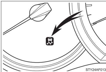
If four wheels spin, the slip indicator flashes to indicate that the active traction control system has been engaged.
