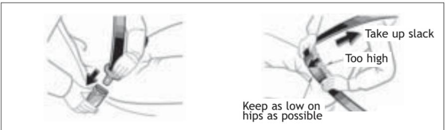
If belt is fully extended, then retracted even slightly, it cannot be re-extended beyond that point, unless fully retracted again. This feature is used to help hold child restraint systems securely.
