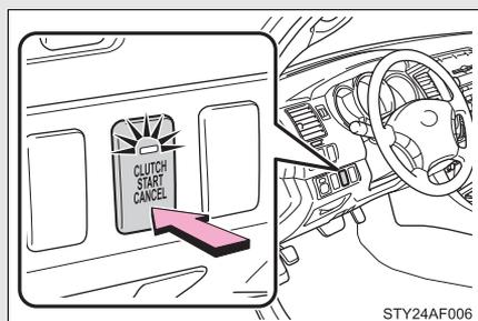
Press the CLUTCH START CANCEL switch to cancel the clutch start system when the engine switch is turned to the ON position.
