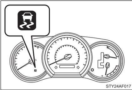
If the vehicle is in danger of slipping, the rear wheels (2WD models) or four wheels (4WD models) spin, the vehicle starts to roll backwards when starting on an incline, this indicator flashes to indicate that the VSC/TRAC/hill-start assist control systems have been engaged.
