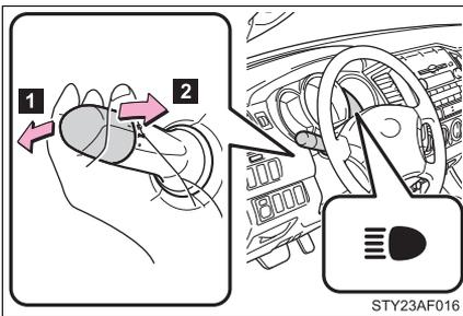
**1** With the headlights on, push the lever forward to turn on the high beams.
