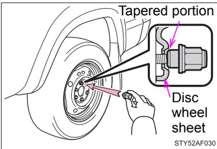
Tighten the nuts until the tapered portion comes into loose contact with the disc wheel sheet.
