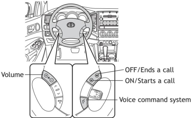
Bluetooth® technology allows you to place or receive calls without taking your hands from the steering wheel or using a cable to connect the telephone and the system.
