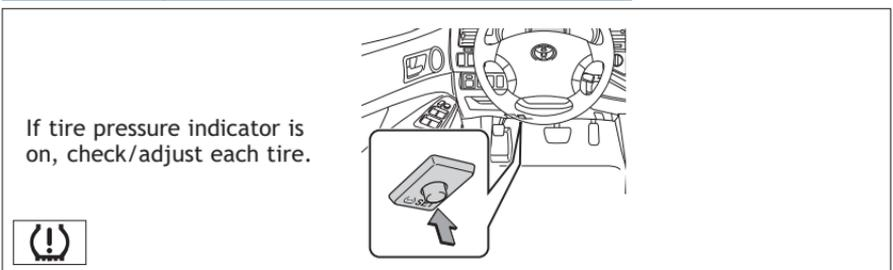
After adjusting tire pressures, or after tires have been rotated or replaced, turn the ignition switch to "ON" and press and hold the "SET" button until indicator blinks three times. Let the vehicle sit for a few minutes to allow initialization to complete.
