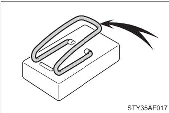
This clip must be removed prior to adhesion of the fastener.
