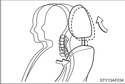
When the occupant's back presses against the seatback during a rear-end collision, the head restraint moves slightly forward to help reduce the risk of whiplash on the seat occupant.
