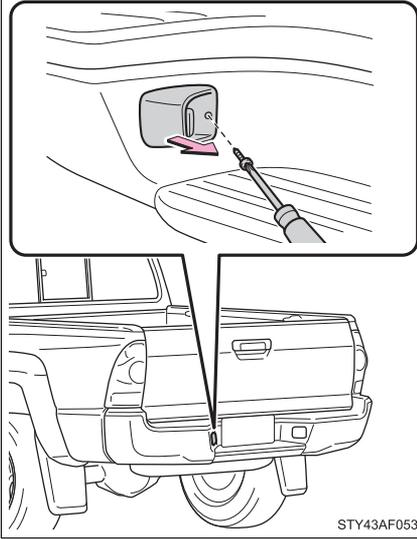
Remove the screw and light unit.
