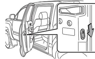
Moving the lever to "LOCK" will allow the door to be opened only from the outside.
