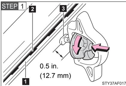
Loosen the thumb wheel in a counterclockwise motion, and depress the wheel so that the locking plate maintains 0.5 in. (12.7 mm) gap.
