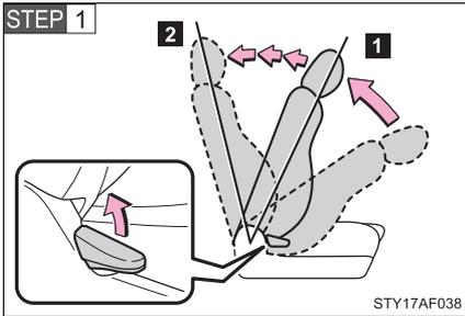
Fold down the front seat seatback and back to the 1st lock position (most upright position) until it locks into place. Adjust the seatback to the 10th lock position.
