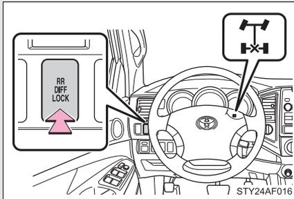
Press the RR DIFF LOCK switch to lock the rear differential.
