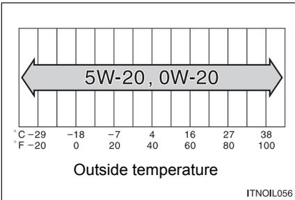
The 0W portion of the oil viscosity rating indicates the characteristic of the oil which allows cold startability. Oils with a lower value before the W allow for easier starting of the engine in cold weather.
