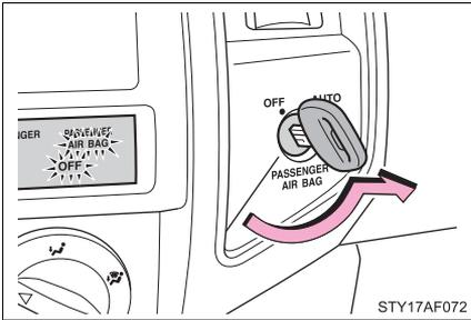
Turn the passenger airbag off switch counterclockwise to the OFF position and remove the key.
