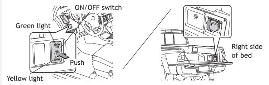
The engine must be running for use.
