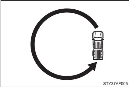
**STEP 3** Drive the vehicle at 5 mph (8 km/h) or less in a circle until the direction is displayed.
