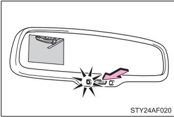
While displaying the screen, press the AUTO button on the inside rear view mirror to switch the screen ON/OFF mode.
