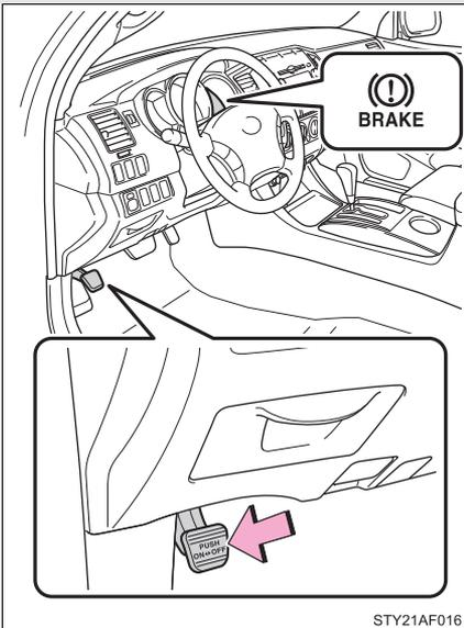
Sets the parking brake\*. (Depressing the pedal again releases the parking brake.)
