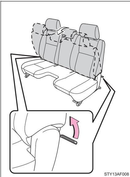
Pull the seatback lock release lever and fold down the seatback.
