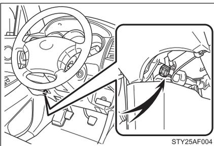
Your vehicle is equipped with a service connector for the trailer brake controller as shown.
