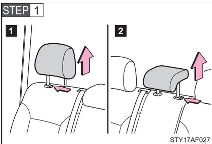
Remove the head restraint.
