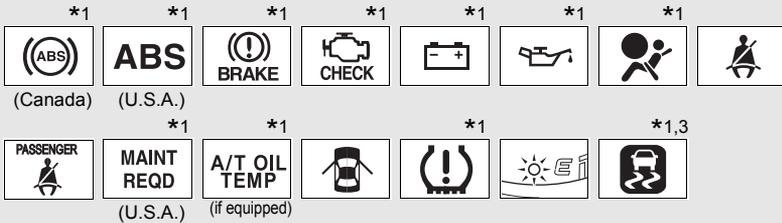
\*1: These lights turn on when the engine switch is turned to the ON position to indicate that a system check is being performed. They will turn off after the engine is started, or after a few seconds. There may be a malfunction in a system if a light does not come on, or if the lights do not turn off. Have the vehicle inspected by your Toyota dealer.
