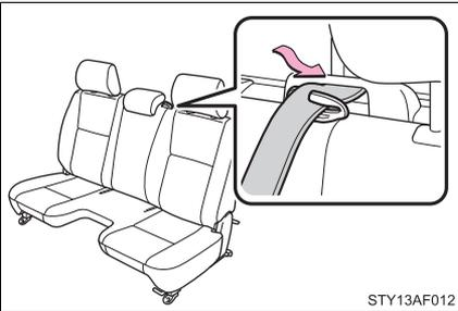
Make sure the shoulder belt pass through the guide when using the center seat belt.
