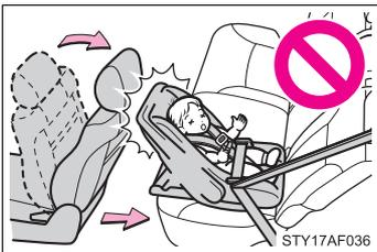
● Access Cab and Double Cab models: If the driver's seat interferes with the child restraint system and prevents it from being attached correctly, attach the child restraint system to the right-hand rear seat.
