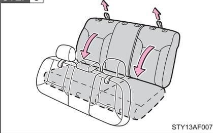
Fold down the seatback by pulling the lock release strap.
