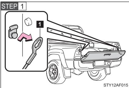
Open the tailgate to the angle where you can release the brackets on the support cables from the lugs on both sides.
