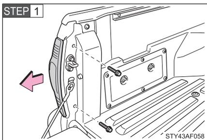
Remove the bolts and rear combination assembly.
