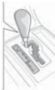
\* The engine switch must be "ON" and the brake pedal depressed to shift from Park.
