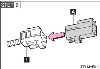
Attach the connector cover (Gray) to the tailgate wire harness connector (White).
