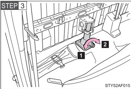
Loosen and remove the jack.
