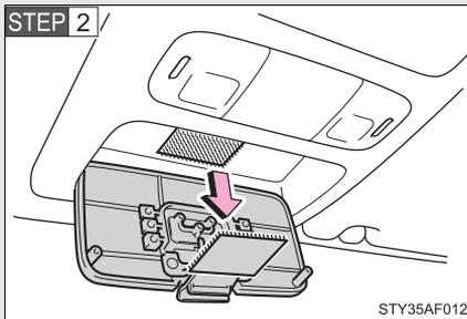
Remove the hook-and-loop fastener square.
