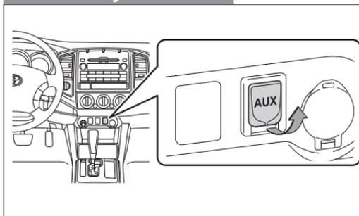
Push "DISC·AUX" button after inserting a mini plug into the AUX audio jack to listen to music from a portable audio device through the vehicle's speaker system while in AUX mode.
