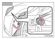
Partly remove the fender liner and turn the bulb base counterclockwise.
