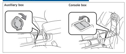
The "ENGINE START STOP" switch/engine switch must be in the "ACC" or "ON" position to be used.
