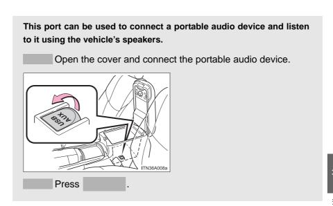
$\ensuremath{\mathrm{n}}$  Operating portable audio devices connected to the audio system
