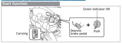
NOTE: Gear shift lever must be in Park and brake pedal depressed.
