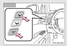
Push the "SET" button, then within 3 seconds, push button "1" or "2" until the signal beeps.
