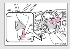
Hold the steering wheel and press the telescopic lock release lever, and adjust to the ideal position by moving the steering wheel horizontally.
