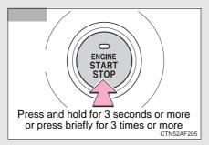
Vehicles with a smart key system: To stop the engine, press and hold the "ENGINE START STOP" switch for 3 consecutive seconds or more, or press it briefly for 3 times or more in succession.
