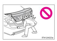
1 The trunk lid may fall if it is not opened fully. It is more difficult to open or close the trunk lid on an incline than on a level surface, so beware of the trunk lid unexpectedly opening or closing by itself. Make sure that the trunk lid is fully open and secure before using the trunk.
