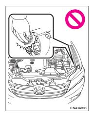
Low beam metal back cover may be very hot after operation of engine and/ or low beams. To avoid potential burn, do not touch metal back cover under these conditions.
