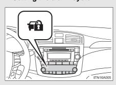
Close the doors, trunk and hood, and lock all doors. The system will be set automatically after 30 seconds.
