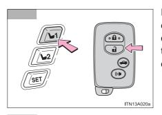
Push the "1" or "2" button on the driver's side and the button on the wireless remote control at the same time for about 1 second until you hear a beep.
