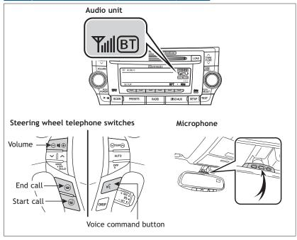
Bluetooth® technology allows dialing or receipt of calls without taking hands from the steering wheel or using a cable to connect the compatible telephone and the system.
