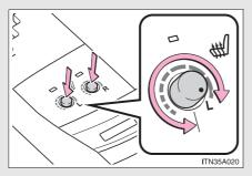
Press the knob to turn the system on, and turn the knob to the desired temperature setting.
