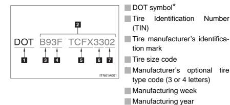
\*: The DOT symbol certifies that the tire conforms to applicable Federal Motor Vehicle Safety Standards.
