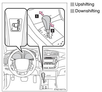
The initial shift range in S mode is set automatically to 5 or 4 according to vehicle speed. However, the initial shift range may be set to 3 if AI-SHIFT has operated while the shift lever was in the D position.  $(\rightarrow P. 159)$
