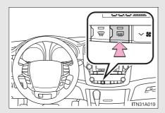
Press the button to turn on the rear window and outside rear view mirror defoggers. The defoggers will automatically turn off after approximately 15 minutes. Pressing the button again also turns the defoggers off.
