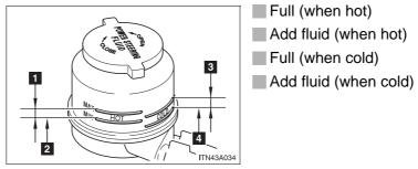
Hot: The vehicles has been driven around 50 mph (80 km/h) for 20 minutes, or slightly longer in frigid temperatures. (Fluid temperature, 140  $^{\circ}$ F - 175  $^{\circ}$ F [60  $^{\circ}$ C - 80  $^{\circ}$ C]).
