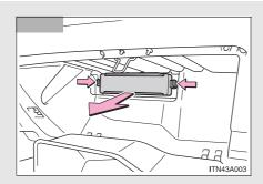
Remove the filter cover while pushing in both ends of the cover.
