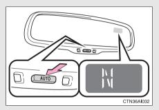
To turn the compass on or off, press and hold "AUTO" for 3 seconds.
