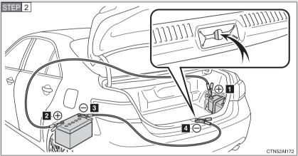
Connecting the jumper cables
