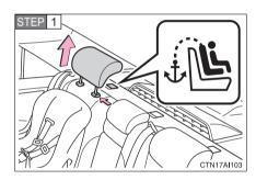
Secure the child restraint using the seat belt or LATCH anchors. Remove the head restraint.
