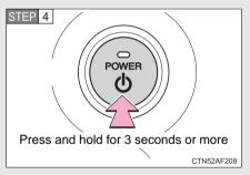
Stop the hybrid system by pressing and holding the "POWER" switch for 3 consecutive seconds or more.
