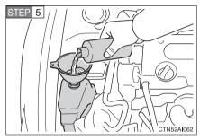
Add engine coolant if necessary.
