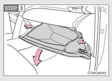
Apply pressure to the glove box as shown to disconnect the claws.
