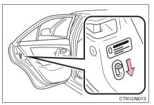
The door cannot be opened from inside the vehicle when the locks are set.
