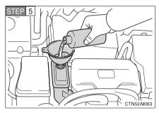
Add power control unit coolant if necessary.
