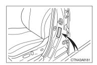
For the GAWR, see the Certification Label. For the maximum load of the tire, see the load limit at maximum cold tire inflation pressure mentioned on the sidewall of the tire. ( $\rightarrow$ P. 462)
