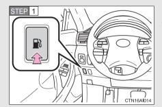
Press the fuel filler door opener switch.
