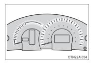
The brightness of the arcs around the fuel economy meter and speedometer change according to the eco drive level. The higher the fuel economy, the brighter the light becomes.
