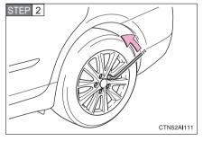
Slightly loosen the wheel nuts (one turn).
