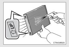
If the filter is dirty, clean by blowing compressed air through the filter from the bottom.
