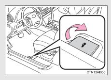
Pull the lever to release the trunk lid
