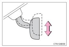
Adjust the height of the rear view mirror by moving it up and down.
