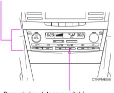
Rear window defogger switch/ Rear window defogger switch and outside rear view mirror defogger switch \* P. 191
