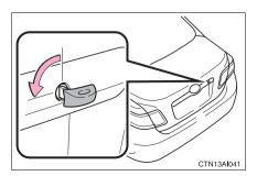
Turn the mechanical key counterclockwise to lock the trunk opener feature.
