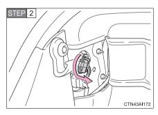
Turn the bulb bases counter-clockwise.
