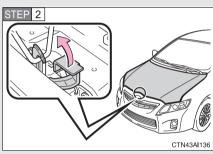
Lift the auxiliary catch lever and lift the hood.
