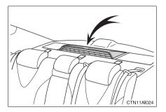
There is an air intake vent on the package tray for the purpose of cooling the hybrid battery (traction battery). If the vent becomes blocked, the hybrid battery may overheat, leading to a reduction in hybrid battery output.
