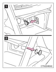
The auxiliary box of the front console is provided with a hole that allows cables to be passed into the cabin from the inside power outlet and AUX port or AUX port/ USB port.
