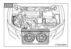
After the hybrid system has cooled down sufficiently, check the engine coolant level and inspect the radiator core (radiator) for any leaks.
