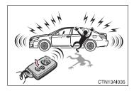
When ((i) is pressed for longer than about one second, an alarm will sound intermittently and the vehicle lights will flash to deter any person from trying to break into or damage your vehicle.
