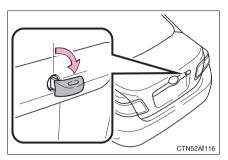
Turn the mechanical key clockwise to open.
