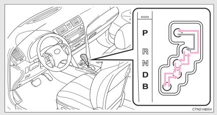
While the "POWER" switch is in ON mode, depress the brake pedal and move the shift lever.
