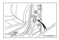
For the GAWR, see the Certification Label. For the maximum load of the tire, see the load limit at maximum cold tire inflation pressure mentioned on the sidewall of the tire.  $(\rightarrow P. 486)$
