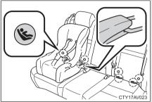
Child restraint LATCH anchors LATCH anchors are provided for the outer rear seats. (But-
