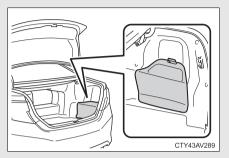
The 12-volt battery is located on the right-hand side of the luggage compartment.
