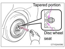
When replacing a steel wheel with a steel wheel, tighten the wheel nuts until the tapered portion comes into loose contact with the disc wheel seat.
