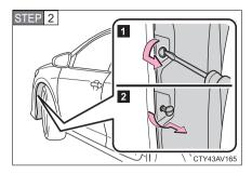
Remove the fender liner clip.
