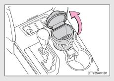
An ashtray can be installed in the cup holder. (→P. 294)
