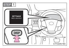
Press the "DISP" button to display the setting screen while the vehicle is stopped, and then press and hold the "DISP" button to display the customize mode screen.
