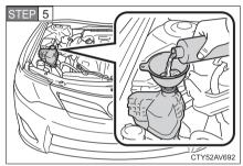
Add power control unit coolant if necessary.
