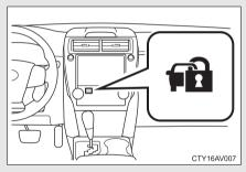
Close the doors, trunk and hood, and lock all the doors. The system will be set automatically after 30 seconds.
