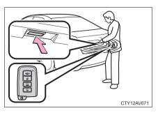
Press the button to unlock the trunk.
