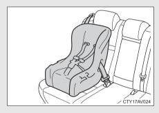
Seat belts equipped with a child restraint locking mechanism (ALR/ELR belts except driver's seat belt) (→P. 85)
