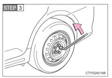
Slightly loosen the wheel nuts (one turn).
