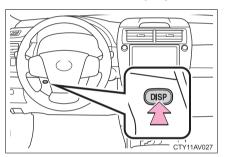
Push the "DISP" switch on the steering wheel several times to select the energy monitor display. (→P. 185)
