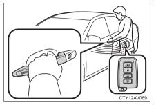
Grip the driver's door handle to unlock the door.\* (Grip the passenger's door handle to unlock all doors.)
