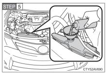
Add engine coolant if necessary.
