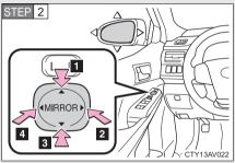
To adjust the mirror, press the switch.
