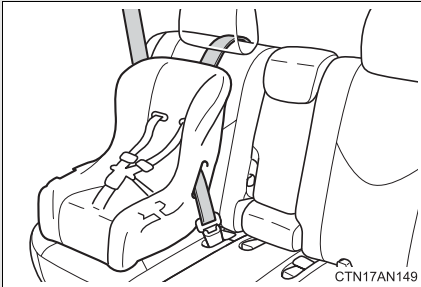
Seat belts equipped with a child restraint locking mechanism (ALR/ELR belts except driver's seat belt)
