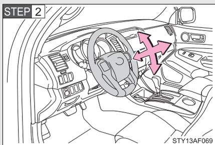
Adjust to the ideal position by moving the steering wheel horizontally and vertically.
