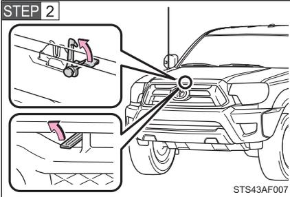
Pull up the hood catch lever and lift the hood.
