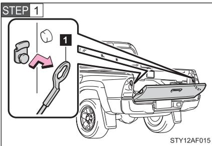
Open the tailgate to the angle where you can release the brackets on the support cables from the lugs on both sides. Lift the support cable bracket up and slide it off.
