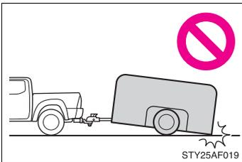
No matter which class of tow hitch applies, for a more safe trailer hookup, the trailer ball setup must be the proper height for the coupler on the trailer.
