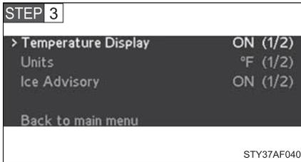
Type A: Press
