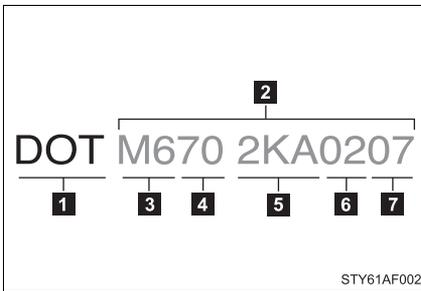
**1** DOT symbol\***2** Tire Identification Number (TIN)**3** Tire manufacturer's identification mark**4** Tire size code**5** Manufacturer's optional tire type code (3 or 4 letters)**6** Manufacturing week**7** Manufacturing year
