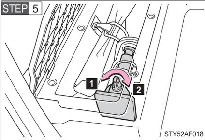
Loosen and remove the jack.
