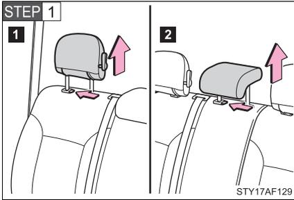
Remove the head restraint.
