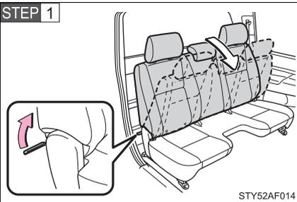
Pull the lever and fold down the seatback.
