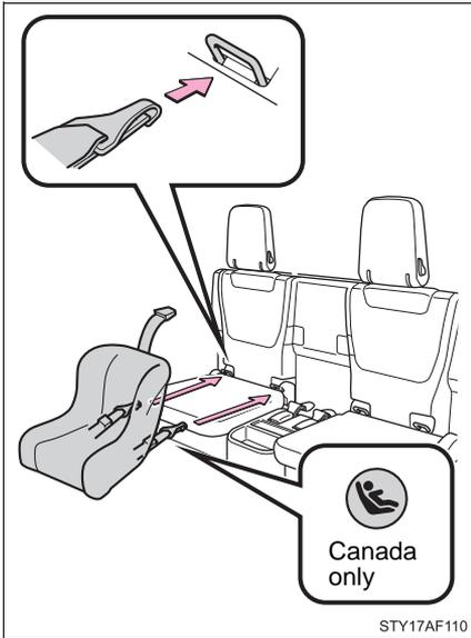
**STEP 1** Latch the hooks of the lower straps onto the LATCH anchors and tighten the lower straps.
