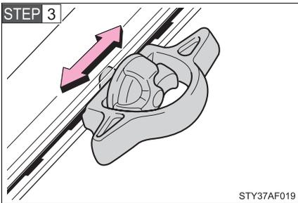
Slide the cleat to the closest detent in the rail system. You will feel that the locking plate snaps into a detent.
