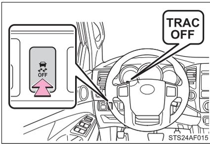
Quickly push and release the VSC OFF switch to turn off TRAC.
