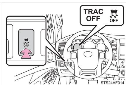
Press and hold the VSC OFF switch for more than 3 seconds while the vehicle is stopped to turn off TRAC, VSC and Trailer Sway Control.
