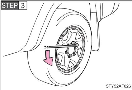
Slightly loosen the wheel nuts (one turn).
