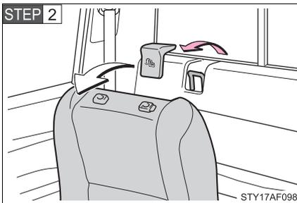
Swing the seatback forward slightly (→P. 50) and remove the anchor bracket cover.
