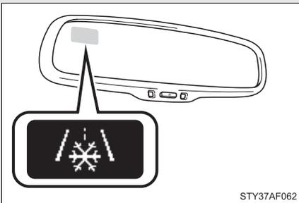
If the outside temperature lowers to 37°F (3°C) or below when the engine switch is in the ON position, the indicator will come on to warn the driver that roads may be icy. Check the road surface and drive carefully. (The indicator will go off when the outside temperature rises to 41°F [5°C].)
