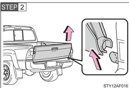
Tilt the tailgate to about 30° from vertical and pull up the right side of the tailgate to unhook the right side.
