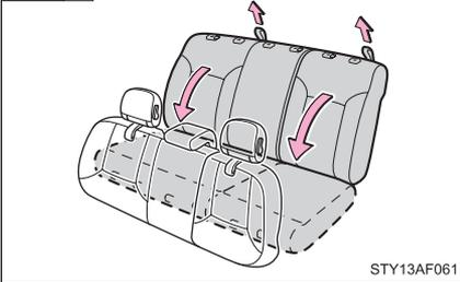
Fold down the seatback by pulling the lock release strap.
