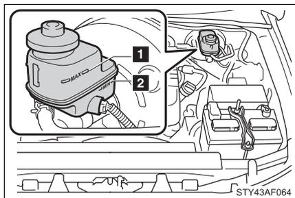
The brake fluid level should be between the MAX and MIN lines on the reservoir.
