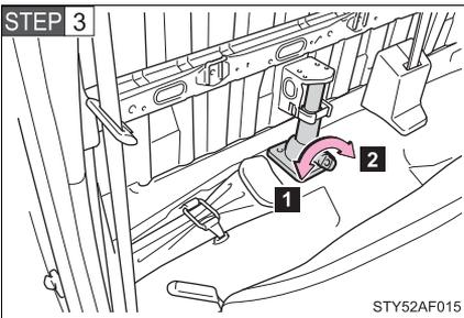
Loosen and remove the jack.
