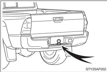
The rear bumper of your vehicle is equipped with a hole to install a trailer ball. If you have any questions, contact your Toyota dealer.
