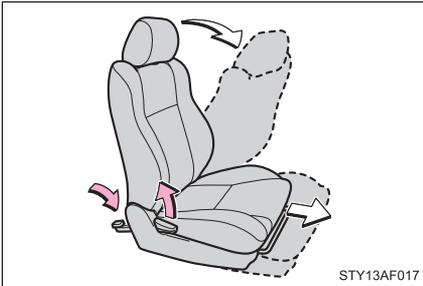
Lift the seatback angle adjusting lever or press the pedal behind the seatback. The seat will slide forward.
