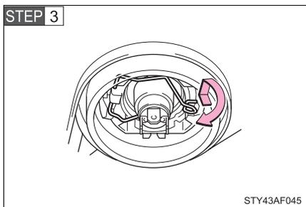
Release the bulb retaining spring.
