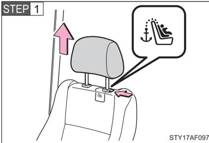
Remove the head restraint.
