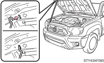
Hold the hood open by inserting the supporting rod into the slot.
