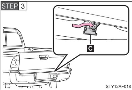
Pull out the plastic wire protector located in the vehicle bed by pressing the tabs and pulling the protector.
