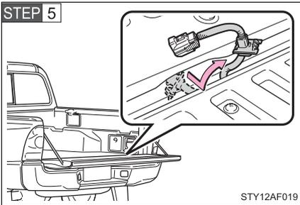
Pull out the wire harness from the vehicle bed.
