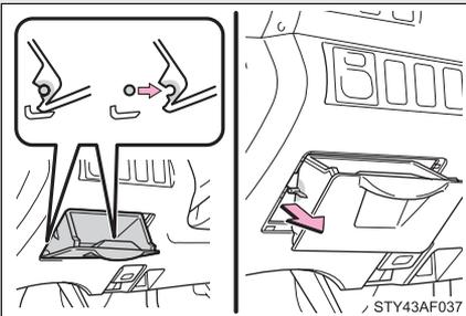
2. Pull up the box and disengage the claws. Remove the stoppers from the cutouts and remove the box.
