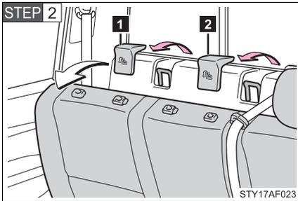
Swing the seatback forward slightly (→P. 50) and remove the anchor bracket covers.
