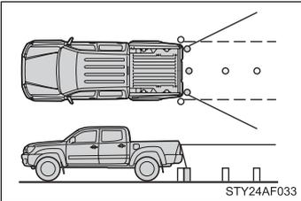
The area covered by the camera is limited. Objects that are close to either corner of the bumper or under the bumper cannot be seen on the screen.
