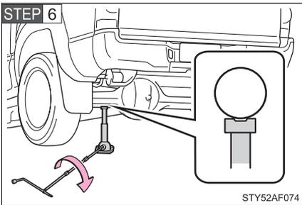
Raise the vehicle until the tire is slightly raised off the ground.
