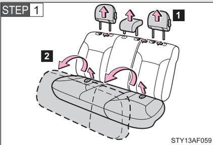
1 Remove the head restraint
