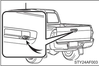
The rear view monitor system camera is located on the tailgate as shown in the illustration.
