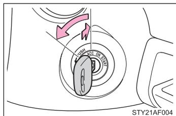
**STEP 1** Shift the shift lever to P (automatic transmission) or N (manual transmission). (→P. 146, 150)
