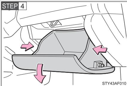
Push in each side of the glove box to disconnect the claws.
