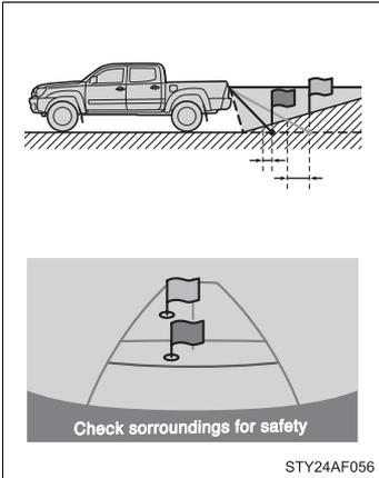
When the grade behind the vehicle slopes up sharply, objects appear to be farther away than they actually are.
