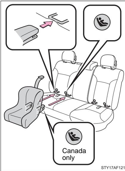
**STEP 1** Widen the gap between the seat cushion and seatback slightly.
