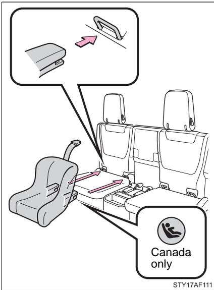
**STEP 1** Latch the buckles onto the LATCH anchors.
