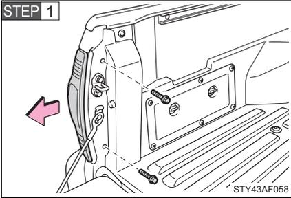
Remove the bolts and rear combination assembly.
