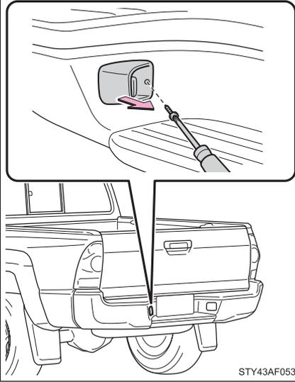
Remove the screw and light unit.
