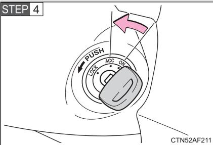
Stop the engine by turning the engine switch to the ACC position.
