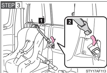
**1** Route the top tether strap through the routing device as shown in the illustration.
