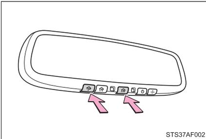
Press and hold down the 2 outside buttons for 10 seconds until the indicator flashes.
