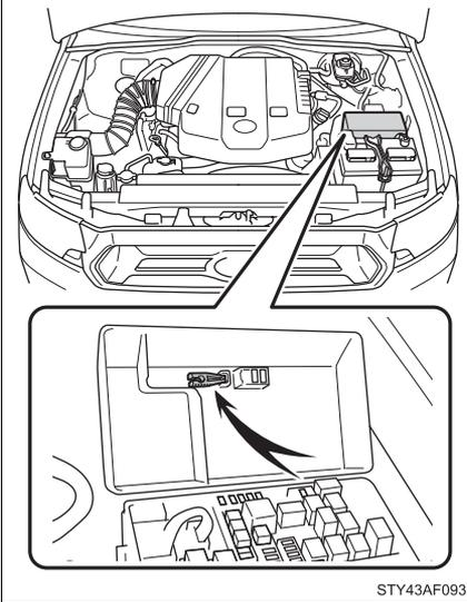
Remove the fuse with the pull-out tool.
