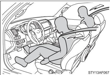
The pretensioner helps the seat belt to quickly restrain the occupant by retracting the seat belt when the vehicle is subjected to certain types of severe frontal collision or a vehicle rollover.
