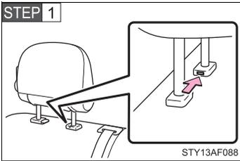
Push a flathead screwdriver into the slot. The slot is located on the left side of the right head restraint anchor.
