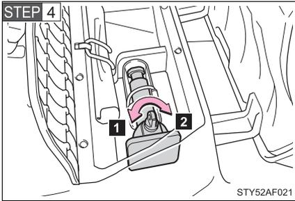
Loosen and remove the jack.
