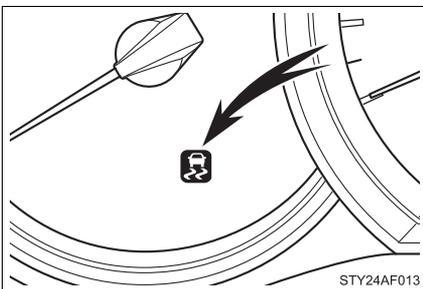
If the rear wheels spin, the slip indicator flashes to indicate that the AUTO LSD system has been controlled the spinning of the rear wheels.
