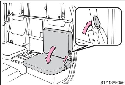
Push the bottom cushion down while pulling the lever until the bottom cushion locks into the seat position.
