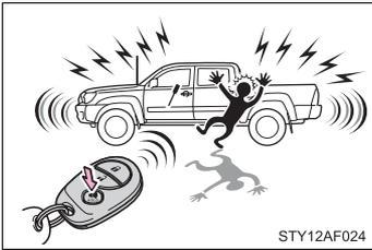
When **HOLD** is pushed for longer than about 1 second, an alarm will sound for about 60 seconds and the vehicle lights will flash to deter any person from trying to break into or damage your vehicle.
