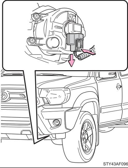
Unplug the connector while pulling the lock release.
