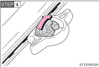
Tighten the thumb wheel in a clockwise motion until the clutch mechanism ratchets.
