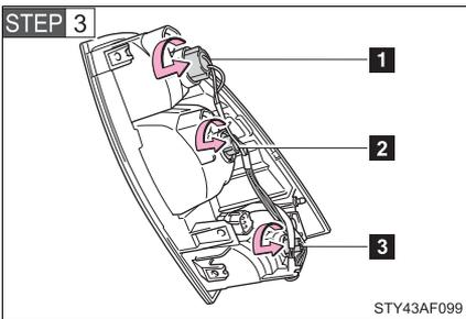
Turn the bulb bases counter-clockwise.
