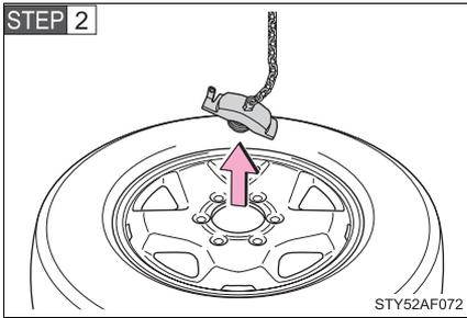
After the tire is lowered completely to the ground, remove the holding bracket.
