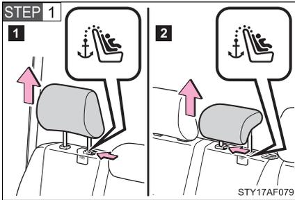
Remove the head restraint.
