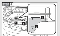
The coolant level is satisfactory if it is between the "F" and "L" lines on the reservoir.
