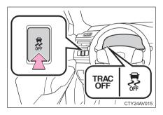
Push and hold the switch for more than 3 seconds while the vehicle is stopped to turn off TRAC and VSC.
