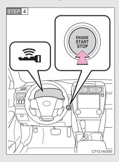
Press the "ENGINE START STOP" switch.
