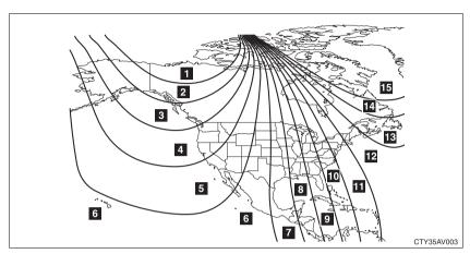
The direction display deviates from the true direction determined by the earth's magnetic field. The amount of deviation varies depending on the geographic position of the vehicle.
