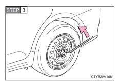
Slightly loosen the wheel nuts (one turn).
