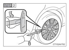
For vehicles with steel wheels, remove the wheel ornament using the wrench.
