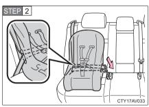
Run the seat belt through the child restraint system and insert the plate into the buckle. Make sure that the belt is not twisted.
