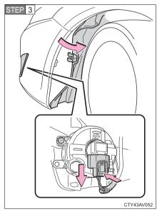
Partly remove the fender liner and unplug the connector while depressing the lock release.
