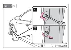
Remove the fender liner clip.
