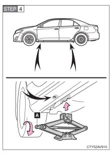
Turn the tire jack portion "A" by hand until the notch of the jack is in contact with the jack point.
