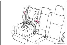
6 If the child restraint has a top tether strap, the top tether strap should be latched onto the top tether strap anchor. (→P. 71)
