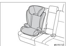
3 Sit the child in the child restraint system. Fit the seat belt to the child restraint system according to the manufacturer's instructions and insert the plate into the buckle. Make sure that the belt is not twisted.
