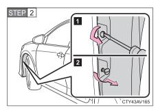
Remove the fender liner clip.
