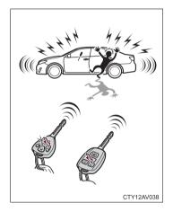
When ((i) is pressed for longer than about one second, an alarm will sound intermittently and the vehicle lights will flash to deter any person from trying to break into or damage your vehicle.
