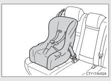
Seat belts equipped with a child restraint locking mechanism (ALR/ELR belts except driver's seat belt) (→P. 72)
