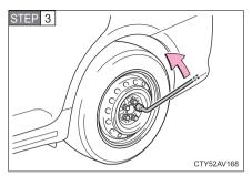
Slightly loosen the wheel nuts (one turn).
