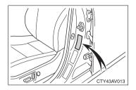
For the GAWR, see the Certification Label. For the maximum load of the tire, see the load limit at maximum cold tire inflation pressure mentioned on the sidewall of the tire. (→P. 569)
