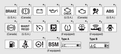
\*1: These lights turn on when the engine switch is turned to the "ON" position (vehicles without a smart key system) or the "ENGINE START STOP" switch is turned to IGNITION ON mode (vehicles with a smart key system) to indicate that a system check is being performed. They will turn off after the engine is started, or after a few seconds. There may be a malfunction in a system if a light does not come on, or if the lights do not turn off. Have the vehicle inspected by your Toyota dealer.
