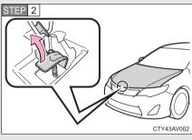
Pull up the auxiliary catch lever and lift the hood.
