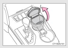
An ashtray can be installed in the cup holder. ( $\rightarrow$ P. 380)
