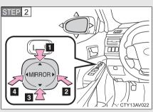
To adjust the mirror, press the switch.
