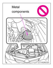
Vehicles with discharge headlights: While the low beam headlights are turned on, and for a short time after they have been turned off, metal components at the rear of the headlight assembly will be extremely hot. To prevent burns, do not touch these metal components until you are certain they
