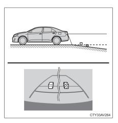
The distance guide lines will appear to be further from the vehicle than the actual distance. Because of this, objects will appear to be closer than they actually are. In the same way, there will be a margin of error between the guidelines and the actual distance/course on the road.
