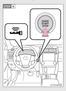
Press the "ENGINE START STOP" switch.
