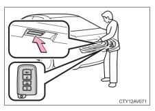
Press the button to unlock the trunk.
