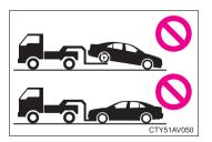
Be sure to transport the vehicle with the front wheels raised or with all four wheels raised off the ground.
