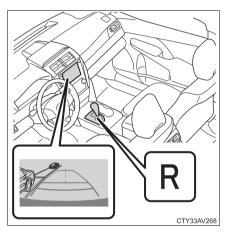
Vehicles without a smart key system: The rear view image is displayed when the shift position is in R and the engine switch is in the "ON" position.
