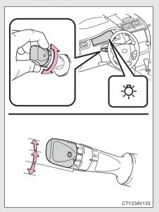
AUTO Vehicles without a smart key system: The headlights and parking lights, daytime running lights turn on and off automatically (when the engine switch is in the "ON" position).
