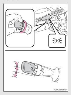
AUTO Vehicles without a smart key system: The headlights, parking lights, daytime running lights and so on turn on and off automatically (when the engine switch is in the "ON" position).
