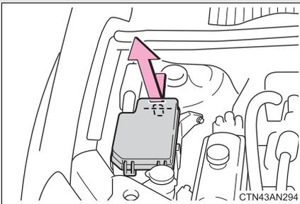
Type B: Push the tab in and lift the lid off.
