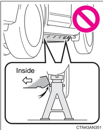
When lowering the vehicle onto jack stands, do not let the jack stands contact the traction battery or undercover. Doing so may damage the vehicle underbody. Working on the vehicle while a jack stand is contacting the traction battery is particularly dangerous because it may not only damage the traction battery, but the vehicle may fall, causing an accident that results in death or serious injury.
