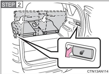
Open the back door and pull the lock release lever to fold down the rear seat.
