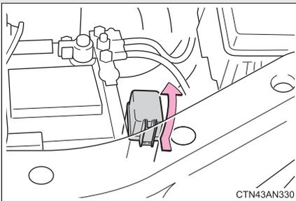
Type C: Push the tab in and lift the lid off.
