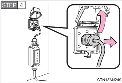
Remove the plug from the electrical receptacle when the charging equipment will not be used for a prolonged period of time.
