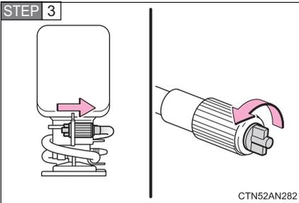
Extend the hose. Remove the air release cap from the hose.
