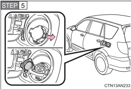
Unlock the charging port cap by moving the lock.
