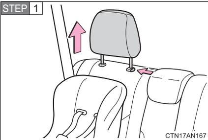
Remove the head restraint.
