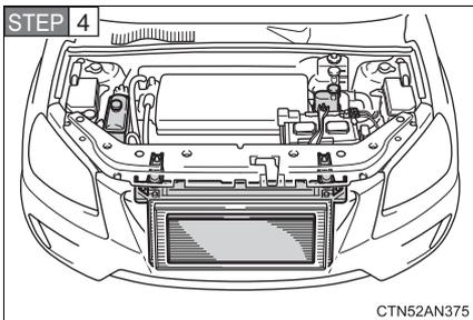
After “High Battery Temp” disappears, check the motor/traction battery coolant level and inspect the cooling system for leaks.
