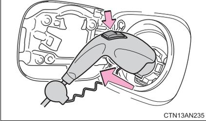
Pull the charging connector towards you while pressing the latch release button.
