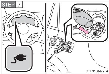
Confirm the charging cable connector's direction and insert it into the charging port.
