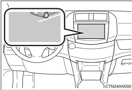
The rear view image is displayed when the shift position is in R.
