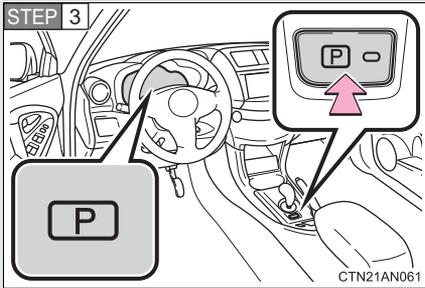
Push the P position switch to shift into P. (→P. 209)
