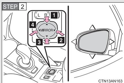
To adjust the mirror, press the switch.
