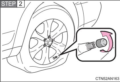
Remove the valve cap from the valve of the punctured tire.
