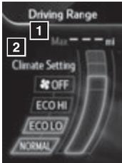
Displays an estimated driving range according to the amount of charge remaining in the traction battery and air conditioning settings.
