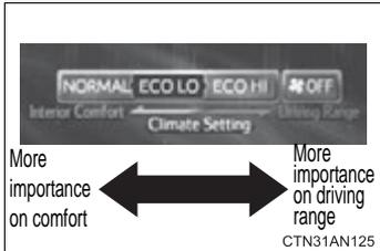
When it is desirable to set the cabin temperature to a more comfortable one, move the operating mode closer to "NORMAL" by pressing ECO. When it is desirable to increase driving range, move the selected mode closer to "OFF" by pressing ECO.
