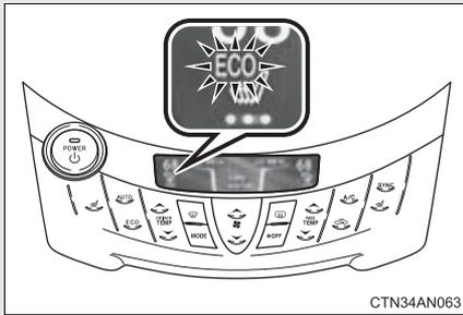
When the air conditioning is set to ECO LO or ECO HI mode, the seat heater is automatically operated and its temperature automatically adjusted according to the outside temperature and air conditioning settings.
