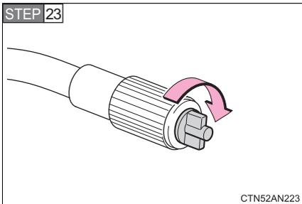
Attach the air release cap to the end of the hose.
