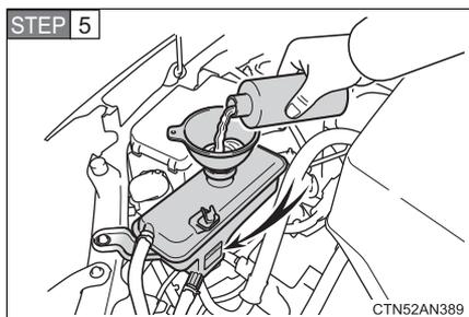
If necessary, add motor coolant up to the “FULL” line.
