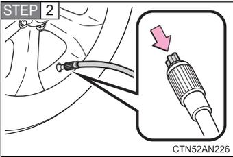
Install the air release cap to the end of the hose and push the protrusion on the air release cap into the tire valve to let some air out.
