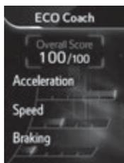
Evaluates the level of eco friendly driving according to acceleration, speed and braking. An overall score is also displayed.
