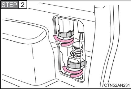
Take out the emergency tire puncture repair kit.
