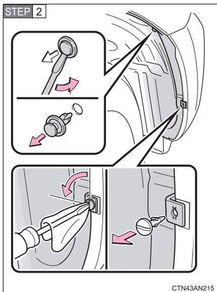
Remove the clips using a flat-head screwdriver.
