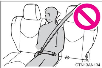
Do not use the rear center seat belt with either buckle released.
