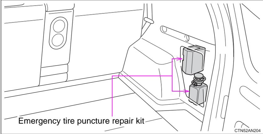
■ Emergency tire puncture repair kit components
