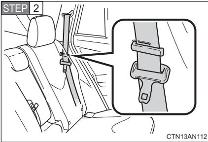
Make sure the outside seat belt passes through the hanger when folding the rear seat.
