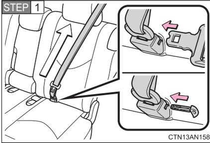
To release tab “A”, insert tab “B” or the mechanical key (→P. 94) into the hole on the buckle.
