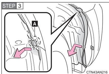
Move section "A" of the fender liner to the inner side of the vehicle, partly removing it and thereby allowing access to the front turn signal.
