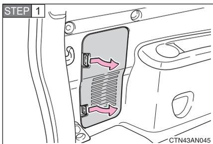
Open the back door (→P. 113) and remove the cover.
