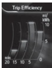
Displays the average power consumption in intervals of 5 minutes. Current power consumption is simultaneously displayed, allowing it to be compared with previous power consumption rates.
