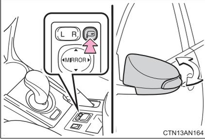
Press the switch to fold the mirrors.
