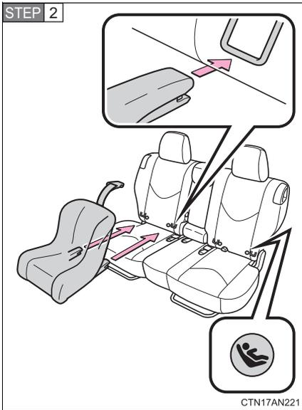
Latch the buckles onto the LATCH anchors.
