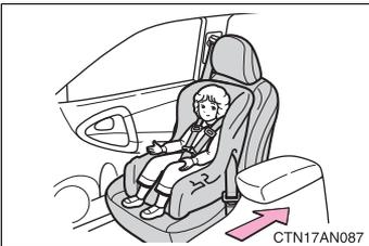
● Only put a forward-facing or booster child seat on the front seat when unavoidable. When installing a forward-facing or booster child seat on the front passenger seat, move the seat as far back as possible even if "AIR BAG OFF" indicator light is illuminated. Failing to do so may result in death or serious injury if the airbags deploy (inflate).
