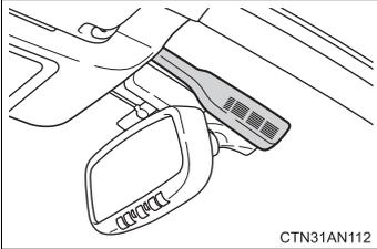
In order to detect fog on the windshield, a sensor which monitors the temperature of the windshield, the surrounding humidity, etc. is installed. (→P. 286)
