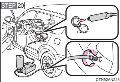
After driving for about 3 miles (5 km), stop your vehicle in a safe place on a hard, flat surface and remove the air release cap from the hose before reconnecting the repair kit.
