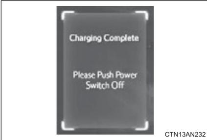
The first time the “POWER” switch is turned to ON mode after charging is completed, a message detailing the results of the charge is shown. Also, if an operation that cannot be carried out during charging was attempted, a warning message will be shown.
