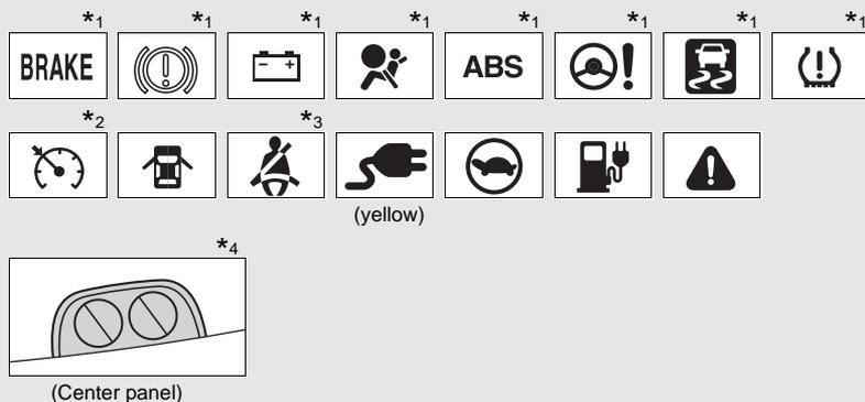
\*1: These lights turn on when the “POWER” switch is turned to ON mode to indicate that a system check is being performed. They will turn off after the EV system is started, or after a few seconds. There may be a malfunction in a system if a light does not come on, or if the lights do not turn off. Have the vehicle inspected by your Toyota dealer for details.
