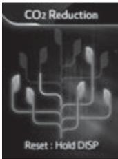
In accordance with the amount of charging performed since the function was last reset, the amount of CO<sub>2</sub> reduction when compared to a conventional gasoline vehicle is displayed as a growing tree.
