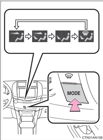
Manual mode: The air outlets switch each time
