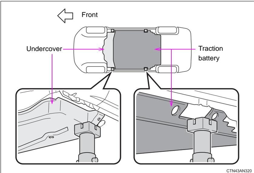
Before lowering the vehicle onto jack stands, check that the jack stands will not contact the traction battery or undercover.
