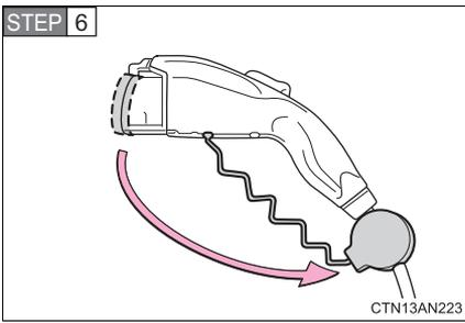
Remove the charging connector cap.
