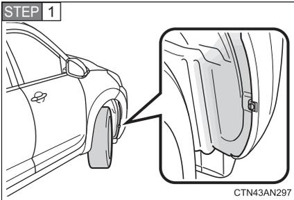
Turn the steering wheel in the opposite direction of the front turn signal that you wish to replace.
