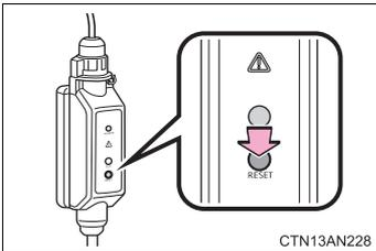
If the error warning indicator of the CCID (Charging Circuit Interrupting Device) illuminates during charging, conduct either of the following procedures.
