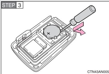
Remove the depleted battery.
