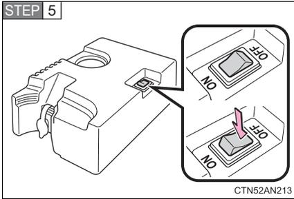
Make sure that the compressor switch is off.
