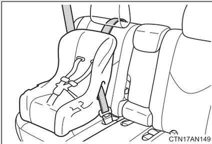
Seat belts equipped with a child restraint locking mechanism (ALR/ELR belts except driver's seat belt) (→P. 134)
