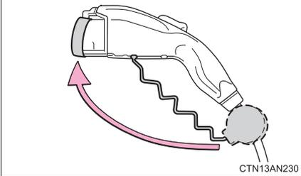
Attach the charging connector cap.
