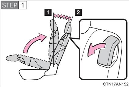
Fold the seatback while pulling the lever. Return the seatback and secure it at the 1st lock position (most upright position). Adjust the seatback to the 7th lock position. (→P. 121)
