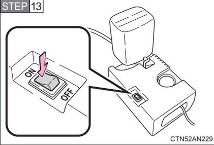
To inject the sealant and inflate the tire, turn the compressor switch on.
