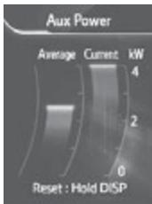
Displays average 12-volt battery power consumption and current 12-volt battery power consumption.
