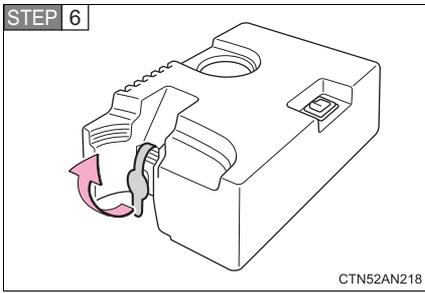
Lift the rubber stopper on the compressor.
