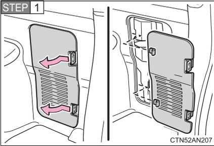
Disengage the claws and remove the cover.
