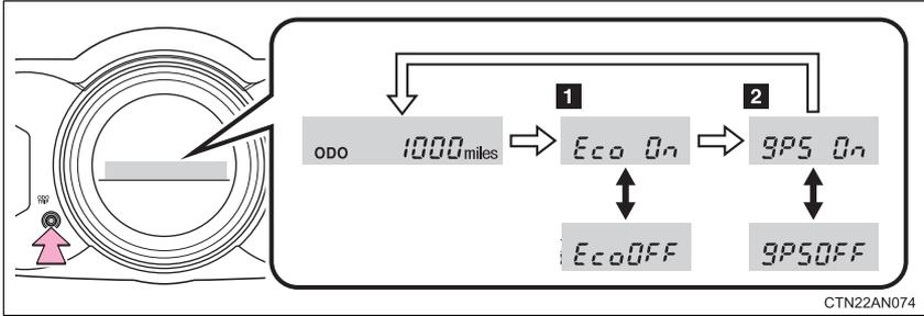
While the odometer is being displayed, customization can be performed by pressing and holding the display change button.
