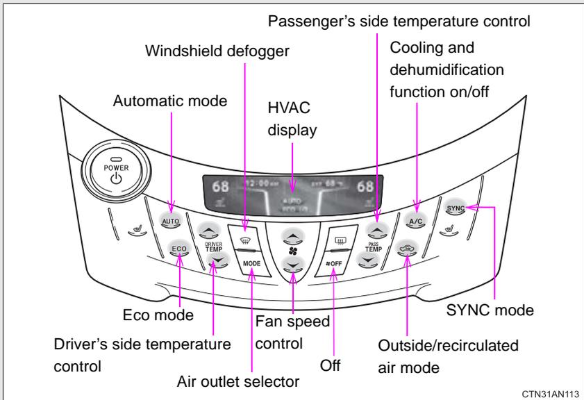
The operating section of the air conditioning panel uses capacitive touch sensors. (→P. 290)
