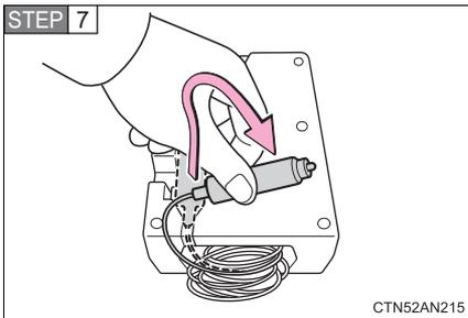
Remove the power plug from the compressor.
