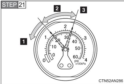
Turn the compressor switch on and wait for an approximately 5 seconds, and then turn it off. Check the tire inflation pressure.
