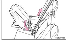
Fully extend the shoulder belt and then allow it to retract slightly in order to activate the ALR lock mode.
