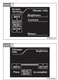
Select "Brightness" on the "Screen Settings" screen, and press the "SELECT RESET" button.
