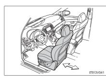
The auto away/return function enables easy access by activating when the driver attempts to enter or exit the vehicle.
