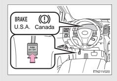
Sets the parking brake\* (Depressing the pedal again releases the parking brake.)
