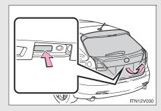
Raise the back door while pushing up the back door opener switch.
