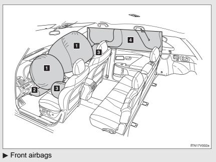
Driver airbag/front passenger airbag Can help protect the head and chest of the driver and front passenger from impact with interior components.
