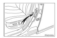
For the GAWR, see the Certification Label. For the maximum load of the tire, see the load limit at maximum cold tire inflation pressure mentioned on the sidewall of the tire. ( $\rightarrow$ P. 504)
