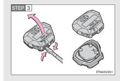
Open the case cover using a flathead screwdriver protected with tape etc. and remove the depleted battery.
