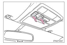
Press and hold the 2 outside buttons for 10 seconds (or 20 seconds depending on the model) until the indicator light flashes.
