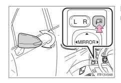
Press the switch to fold the mirrors.
