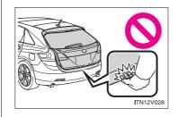
In the event that the back door is left slightly open, the back door closer will automatically close it to the fully closed position. It takes several seconds before the back door closer begins to operate. Be careful not to catch fingers or anything else in the back door, as this may cause bone fractures or other serious injuries.
