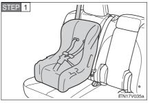
Place the child restraint system on the seat facing the front of the vehicle.
