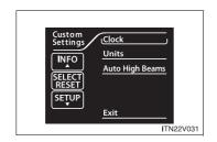
If the vehicle speed exceeds approximately 3 mph (5 km/h) while the settings are being changed, "Please Stop Vehicle to Change Settings" will be displayed on the multi-information display, and setting mode will exit after several seconds. If the "SETUP" button is pressed at a speed in excess of 3 mph (5 km/h), only some of the settings can be changed. To change the other settings, press the "SETUP" button after bringing the vehicle to a complete stop.
