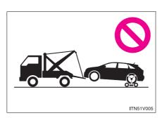
Do not tow with a sling-type truck to prevent body damage.
