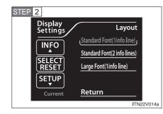
Select the desired layout by pressing the "INFO" or "SETUP" button, and press the "SELECT RESET" button.
