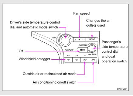
3-1. Using the air conditioning system and defogger
