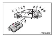
When (() is pressed for longer than about one second, an alarm will sound for about 60 seconds and the vehicle lights will flash or come on to deter any person from trying to break into or damage your vehicle.
