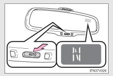
To turn the compass on or off, push and hold "AUTO" for longer than 3 seconds.
