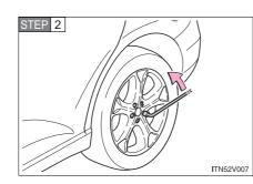
Slightly loosen the wheel nuts (one turn).
