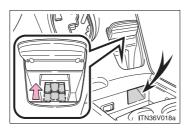
The auxiliary boxes of the front console are provided with a hole that allows cables to be passed from the power outlet and AUX port/USB port.
