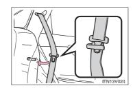
Pass the outer seat belts and plates through the seat belt hangers to prevent the shoulder belts from being damaged.
