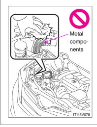
Vehicles with discharge headlights: While the headlights are turned on, and for a short time after they have been turned off, metal components at the rear of the headlight assembly will be extremely hot. To prevent burns, do not touch these metal components until you are certain they have cooled down.
