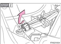
Unlock the tightening strap.
