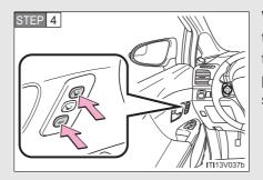
While pressing the "SET" button, or within 3 seconds after the "SET" button is pressed, press button "1" or "2" until the signal beeps.
