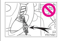
Do not attach anything to or lean anything against areas such as the dashboard or steering wheel pad or lower portion of the instrument panel. These items can become projectiles when SRS driver, front passenger and knee airbags deploy.
