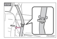
Pass the outer seat belts and plates through the seat belt hangers.
