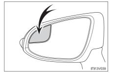
The Blind Spot Mirrors increase the view of surrounding area to assist the driver when checking surrounding area before changing lanes.
