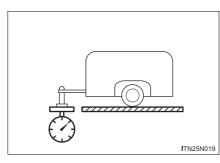
The load placed on the trailer hitch ball. ( $\rightarrow$ P. 271)
