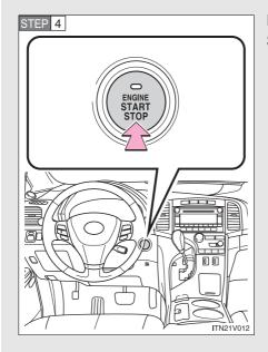
Press the "ENGINE START STOP" switch.
