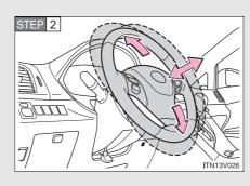
Adjust to the ideal position by moving the steering wheel horizontally and vertically.
