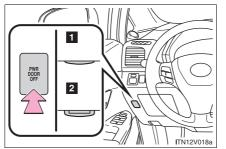
Turn the main switch to disable the power back door system.
