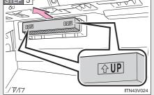
Remove the air conditioning filter and replace it with a new one.
