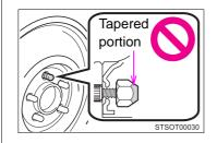
Be sure to install the wheel nuts with the tapered ends facing inward. Installing the nuts with the tapered ends facing outward can cause the wheel to break and eventually cause the wheel to come off while driving, which could lead to an accident resulting in death or serious injury.
