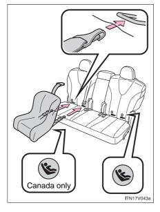
STEP 2 Widen the gap between the seat cushion and seatback slightly.
