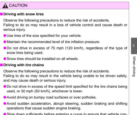
Slow down sufficiently before entering a curve to ensure that vehicle control is maintained.
