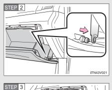
Open the glove box. Slide off the damper.
