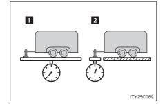
If using a weight distributing hitch when towing, return the front axle to the same weight as before the trailer connection.
