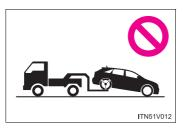
2WD models: Never tow this vehicle from the rear with the front wheels on the ground. This may cause serious damage to the transmission. If towing from the rear, use a towing dolly.
