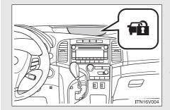
Close the doors and hood, and lock all doors using the entry function (vehicles with smart key system) or the wireless remote control. The system will be set automatically after 30 seconds.
