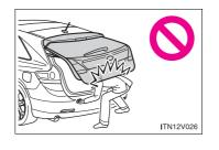
The back door may suddenly shut if it is not opened fully. It is more difficult to open or close the back door on an incline than on a level surface, so beware of the back door unexpectedly opening or closing by itself. Make sure that the back door is fully open and secure before using the luggage compartment.
