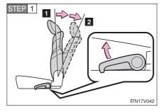
Fold the seatback while pulling the lever. Return the seatback and secure it as upright as possible (1st lock position). Adjust the seatback to the 3rd lock position.  $(\rightarrow P. 70)$
