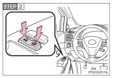
Shift the shift lever to "P" or "N", press and hold the driver's door lock switch ( $\bigcirc$  or  $\bigcirc$ ) for about 5 seconds then release.
