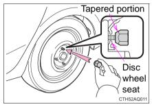
When replacing an aluminum wheel with a compact spare tire, tighten the wheel nuts until the tapered portion comes into loose contact with the disc wheel seat.
