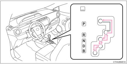
Vehicles without a smart key system: While the engine switch is in the "ON" position, move the shift lever with the brake pedal depressed.
