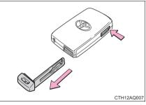
After using the mechanical key, store it in the electronic key. Carry the mechanical key together with the electronic key. If the electronic key battery is depleted or the entry function does not operate properly, you will need the mechanical key.  $(\rightarrow P. 476)$
