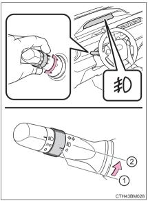
**Fog lights can be used when** The headlights are on in low beam.
