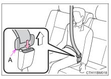
**2** To release tab "B", insert the key ( $\rightarrow$ P. 118) or tab "A" into the hole on the buckle.
