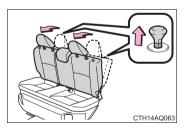
2 Pull the head restraint up while pressing the lock release button.
