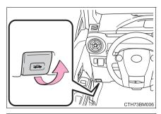
2 Pull up the auxiliary catch lever and lift the hood.
