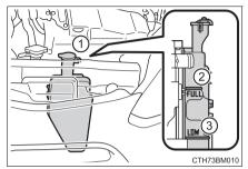
Power control unit coolant reservoir
