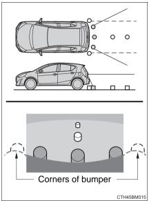
• Items which are located higher than the camera may not be displayed by the monitor.
