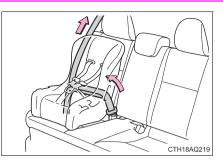
**6** If the child restraint has a top tether strap, the top tether strap should be latched onto the top tether strap anchor. ( $\rightarrow$ P. 67)
