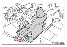
2 Push the tabs in and remove the cover by pulling it towards you.
