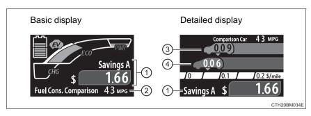
With 2 types of displays available, the cost of the consumed fuel can be displayed or the fuel consumption's comparison can be displayed.
