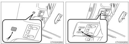
The vehicle's built in microphone is used when talking on the phone.
