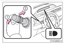
You can flash the high beams with the headlights on or off.
