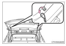
2 Pull the luggage cover backward to disengage the anchors.
