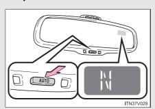
To turn the compass on or off, push and hold "AUTO" for longer than 3 seconds.
