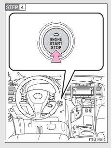
Press the "ENGINE START STOP" switch.
