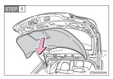
Open the back door and remove the trim board.
