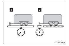
If using a weight distributing hitch when towing, return the front axle to the same weight as before the trailer connection.
