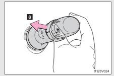
Wash/wipe operation Wipers operate automatically.
