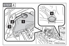
The coolant level is satisfactory if it is between the "F" and "L" lines on the reservoir.
