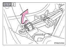
Unlock the tightening strap.
