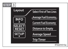
When a 2-line layout is selected in STEP 2, the "Layout" screen is displayed. First, using the "INFO" and "SETUP" buttons, select the item you wish to display in the first line, and then press the "SELECT RESET" button.
