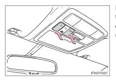
Press and hold the 2 outside buttons for 10 seconds (or 20 seconds depending on the model) until the indicator light flashes.
