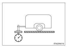
The load placed on the trailer hitch ball. ( $\rightarrow$ P. 289)
