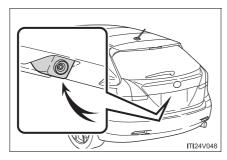
The camera for the rear view monitor system is located above the license plate.
