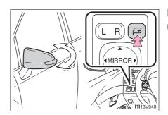
Press the switch to fold the mirrors.
