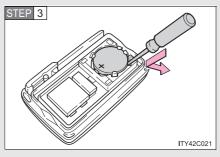
Remove the depleted battery.
