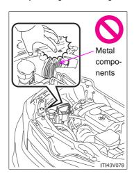
Vehicles with discharge headlights: While the headlights are turned on, and for a short time after they have been turned off, metal components at the rear of the headlight assembly will be extremely hot. To prevent burns, do not touch these metal components until you are certain they have cooled down.
