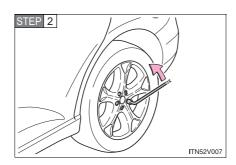
Slightly loosen the wheel nuts (one turn).
