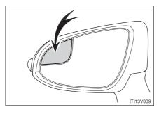
The Blind Spot Mirrors increase the view of surrounding area to assist the driver when checking surrounding area before changing lanes.
