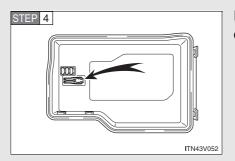
Remove the fuse with the pullout tool.
