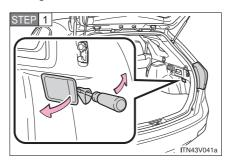
Open the back door and remove the cover.
