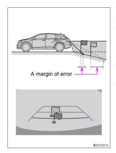
The distance guide lines will appear to be farther from the vehicle than the actual distance. Because of this, objects will appear to be closer than they actually are. In the same way, there will be a margin of error between the guide lines and the actual distance/course on the road.
