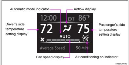
The settings display will differ according to the situation. If pressed while in automatic mode, the status of all settings will be dis-
