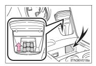
The auxiliary boxes of the front console are provided with a hole that allows cables to be passed from the power outlet and AUX port/USB port.
