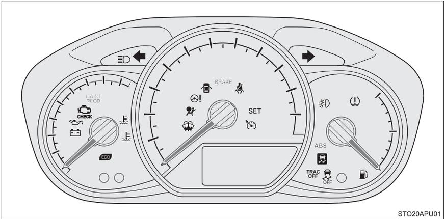
This illustration represents a meter with a tachometer and may differ from the look of the meter without a tachometer.
