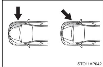
The SRS side and curtain shield airbags do not generally inflate if the vehicle is involved in a frontal or rear collision, if it rolls over, or if it is involved in a low-speed side collision.
