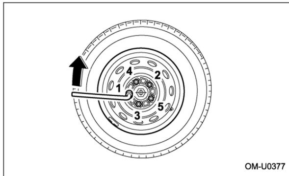
14. Use the wheel nut wrench to securely tighten
