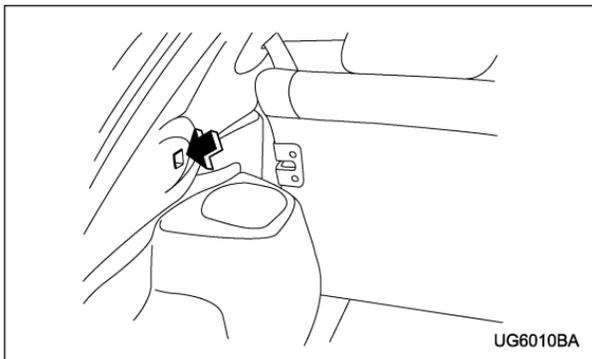
2. Insert the projections located on the both ends of the sleeve into the recesses of the retainers.
