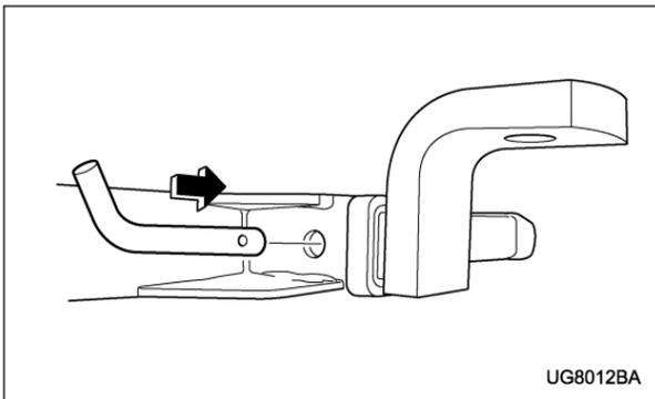
2. Insert the hitch pin into the hole on the hitch receiver tube so that the pin passes through the ball mount.
