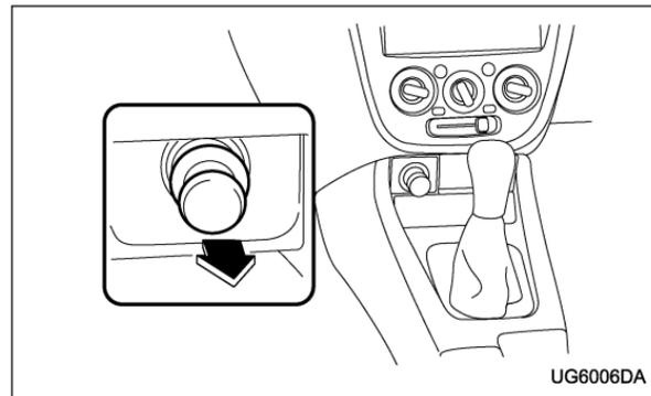
The electrical power outlet located on the lower part of the instrument panel can be used as cigarette lighter socket. A cigarette lighter plug is an optional accessory. It is available from your SUBARU dealer. The cigarette lighter socket may also be used as a power source for an in-car use electrical appliance.
