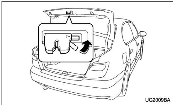
The inside trunk lid release can be cancelled to help prevent unauthorized entry into the trunk. To cancel the trunk lid release, set the lid release cancel lever (located on the inside of the trunk lid, mounted to the trunk lid latch) to the “CANCEL” position. When this lock is in the “CANCEL” position, the trunk can be opened only with the key.
