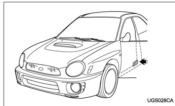
The certification plate attached to the driver's side door jamb shows GVWR (Gross Vehicle Weight Rating) and GAWR (Gross Axle Weight Rating). The GVW (Gross Vehicle Weight) must never exceed the GVWR. GVW is the combined total of weight of the vehicle, fuel, driver, all passengers, luggage, any optional equipment and trailer tongue
