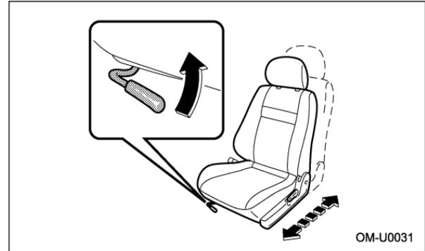
Pull the lever upward and slide the seat to the desired position. Then release the lever and move the seat back and forth to make sure that it is securely locked into place.
