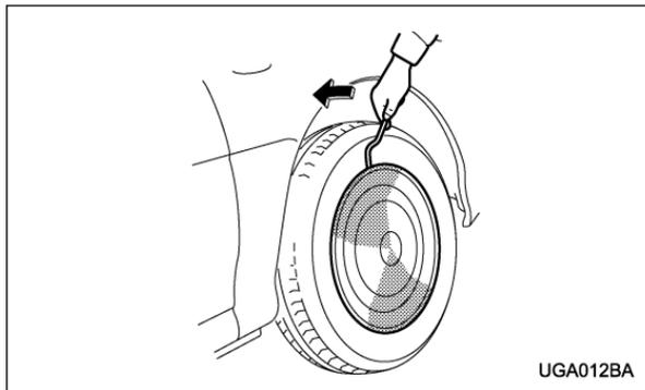
Insert the wheel cover remover into the notch provided, and pry the wheel cover off.
