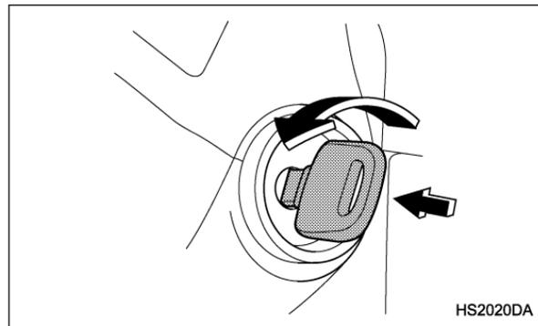
The key can be turned from “ACC” to “LOCK” only when the key is pushed in while turning it.
