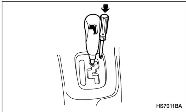
4. Insert the screwdriver into the hole.
