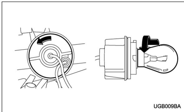
1. Remove the bulb socket from the headlight assembly by turning it counterclockwise.
