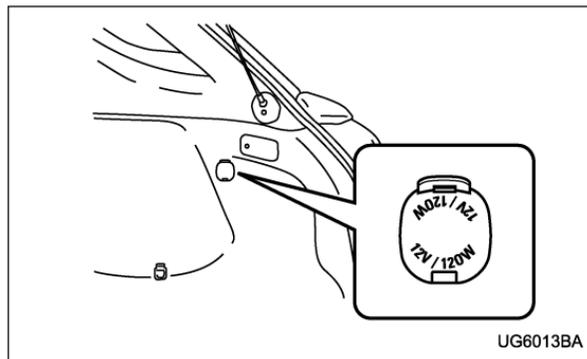
Electrical power (12V DC) from the battery is on tap at the socket when the ignition switch is either in the “ACC” or “ON” position.
