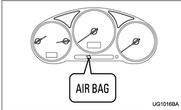
A diagnostic system continually monitors the readiness of the seatbelt pretensioner while the vehicle is being driven. The seatbelt pretensioners share the control module with the SRS airbag system. Therefore, if any malfunction occurs in a seatbelt pretensioner, the SRS airbag system warning light will illuminate. The SRS airbag system warning light will show normal system operation by lighting for about 6 seconds when the ignition key is turned to the "ON" position.
