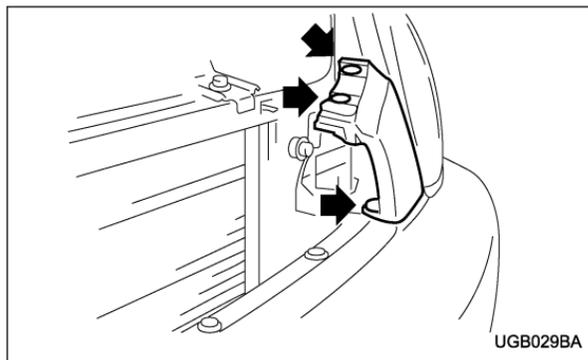
2. Loosen three clips to remove the grille side cover.
