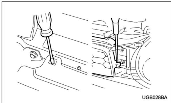
1. Remove the front grille. Use a screwdriver to detach the four clips at the top and the two hooks on each side.
