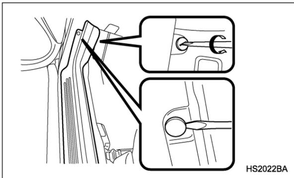
1. Remove the side sill cover on the driver's side.
