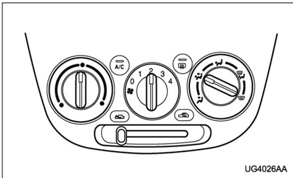
This setting allows you to direct air of different temperatures from the instrument panel and foot outlets. The air from the foot outlets is slightly warmer than
