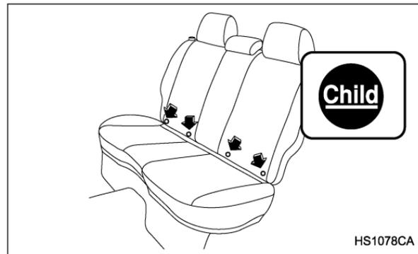
You will find marks "Child" at the bottom of the rear seat seatbacks. These marks indicate the positions of the lower anchorages (bars).
