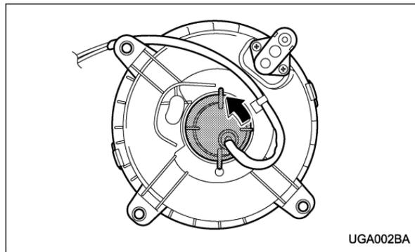
3. Remove the front fog light case cap by turning it counterclockwise.
