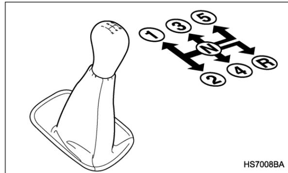
The shift pattern is shown on the shift lever knob. When shifting from 5th gear to reverse gear, first return the shift lever to the neutral position then shift into reverse gear.
