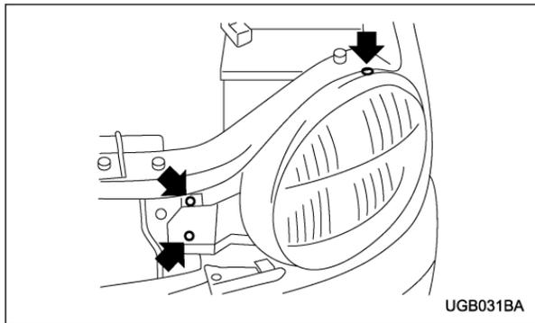
3. Remove three bolts and disconnect connectors,
