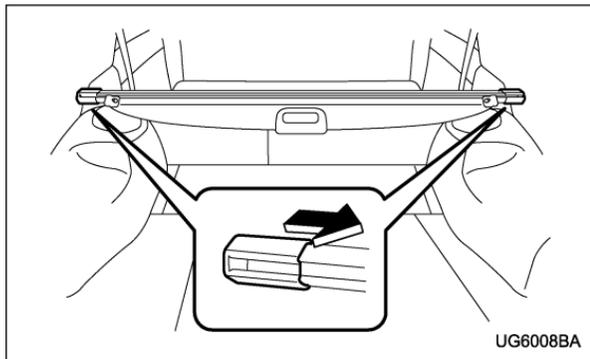
2. Pull either sleeve on the end of the cover housing to shorten the cover's length.
