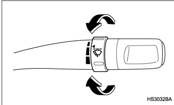
When the wiper switch is in the “
