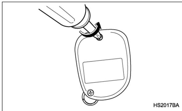
1. Remove the two screws on the back of the transmitter case by using a phillips screwdriver.
