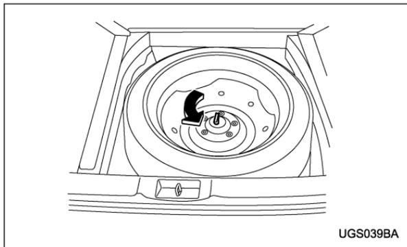
**Sedan:** Remove the floor cover from the trunk. Remove the storage compartment (if so equipped). Turn the attaching bolt counterclockwise, then take the spare tire out.
