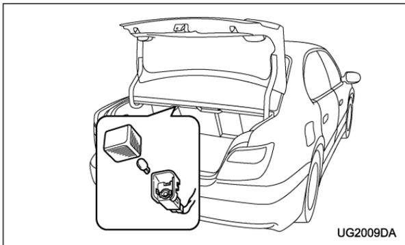
1. Remove the cover by squeezing its sides and pulling it.
