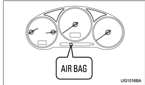
A diagnostic system continually monitors the readiness of the SRS airbag system while the vehicle is being driven. The SRS airbag system warning light "AIRBAG" will show normal system operation by lighting for about 6 seconds when the ignition key is turned to the "ON" position.
