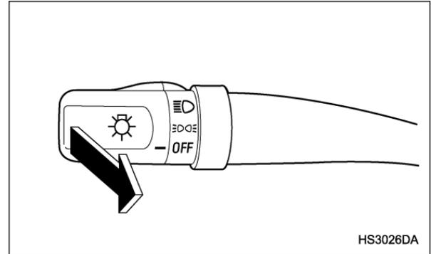
To flash the headlights, pull the lever toward you and then release it. The high beam will stay on for as long as you hold the lever. The headlight flasher works even though the lighting switch is in the “OFF” position.
