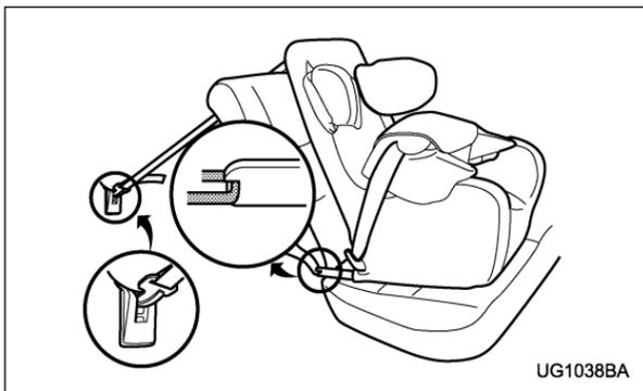
Some types of child restraint systems can be installed on the rear seat of your vehicle without use of the seatbelts. Such child restraint systems are secured to the designated anchorages provided on the vehicle body.
