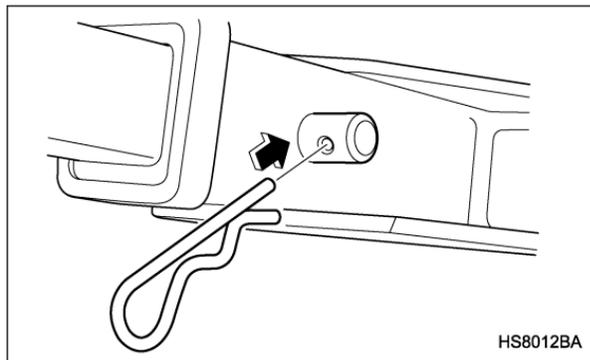
3. Insert the safety pin securely into the hitch pin.
