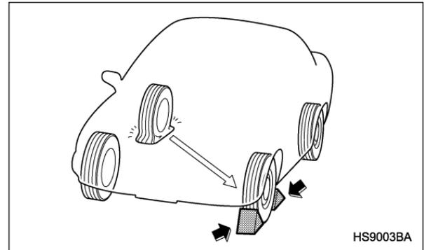
4. Put wheel blocks at the front and rear of the tire diagonally opposite the flat tire.
