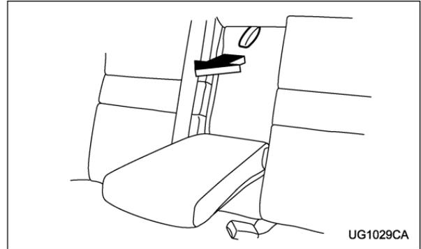
Folding down the armrest and opening the seatback panel affords a loading space for long objects. To open the seatback panel, pull the release tab.
