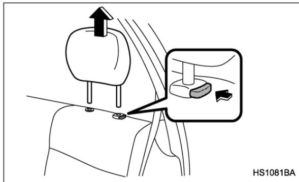
1. Remove the rear seat headrest at the seating position where the child restraint system has been installed with the seatbelt or lower anchorages; lift up the headrest while pressing the release button. Store the headrest in the cargo area. Avoid placing the headrest in the passenger compartment to prevent it from being thrown around in the passenger compartment in a sudden stop or a sharp turn.
