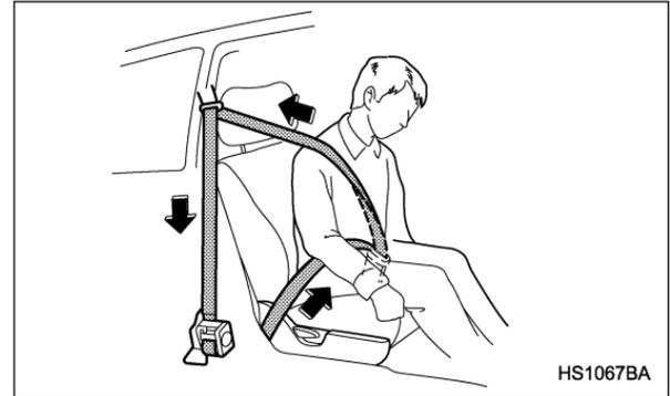
The driver's and front passenger's seatbelts have a seatbelt pretensioner. The seatbelt pretensioners are designed to be activated in the event of an accident involving a moderate to severe frontal collision.
