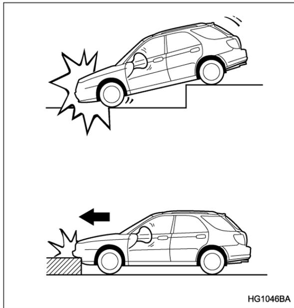
The SRS frontal airbag may be activated when the vehicle sustains a hard impact in the undercarriage area from the road surface (such as when the ve-
