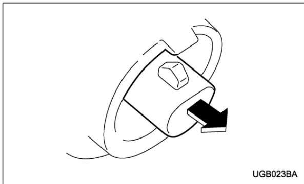
3. Remove the bulb from the headlight assembly.
