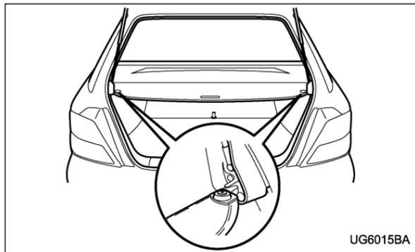
To extend the cover, pull the end of the cover out of the housing, then insert its hooks into the catches as shown. To rewind it, unhook it from the catches and it will rewind automatically. You should hold on to the cover and guide it back into the cover housing while
