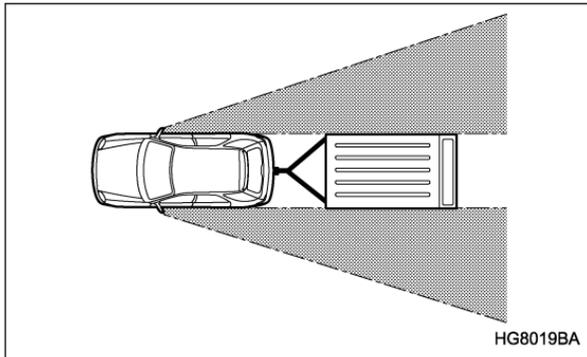
After hitching a trailer to your vehicle, check that the standard side mirrors provide a good rearward field of view without significant blind spots. If significant blind spots occur with the vehicle's standard side mirrors, use towing mirrors that conform with Fed-
