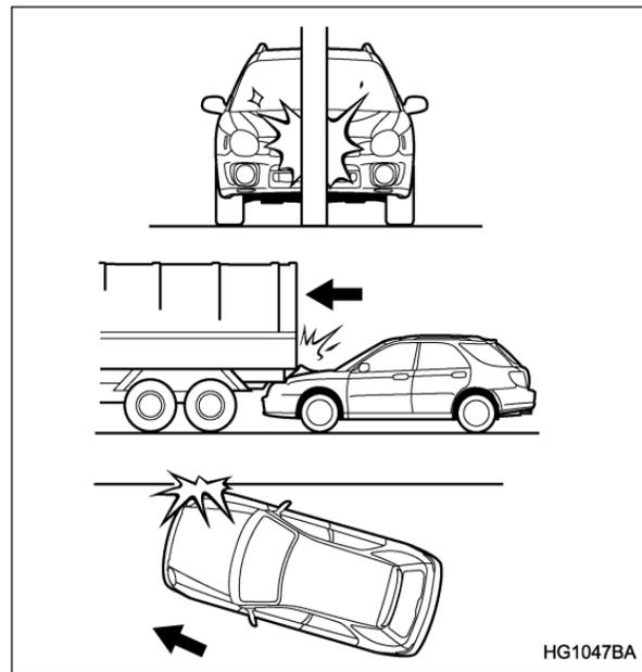
There are many types of collisions which might not necessarily require SRS frontal airbag deployment. If the vehicle strikes an object, such as a telephone
