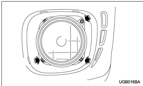
1. Remove the front fog light assembly by removing the three bolts.
