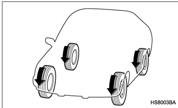
All wheel drive distributes the engine power to all four wheels. AWD vehicles provide better traction when driving on slippery, wet or snow-covered roads and when moving out of mud, dirt and sand. By shifting power between the front and rear wheels, SUBARU AWD can also provide added traction during acceleration and added engine braking force during deceleration.
