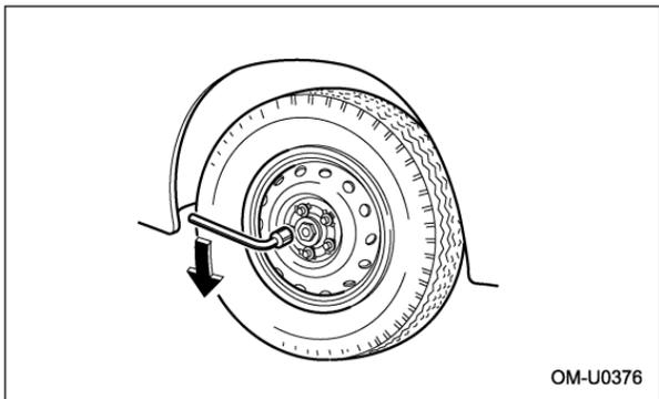
7. Loosen the wheel nuts using the wheel nut wrench but do not remove the nuts.
