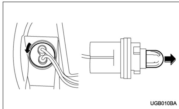
4. Remove the bulb socket from the headlight assembly by turning it counterclockwise.
