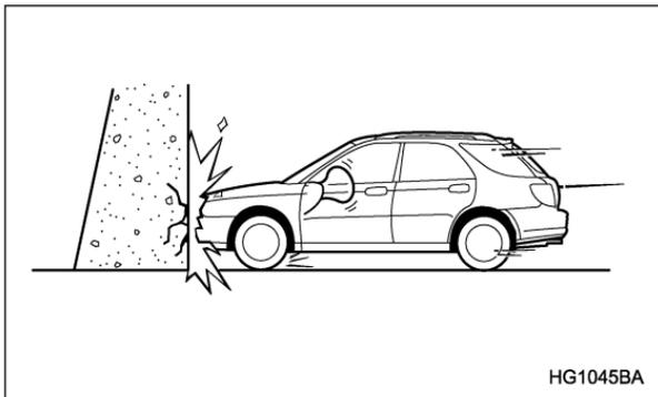
A head-on collision against a thick concrete wall at a vehicle speed of 12 to 19 mph (20 to 30 km/h) or higher activates the SRS frontal airbag. The SRS frontal airbag will also be activated when the vehicle is exposed to a frontal impact similar in fashion and magnitude to the above-mentioned collision.
