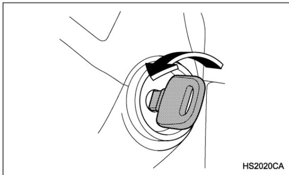
The key can be turned from “ACC” to “LOCK” only when the selector lever is in the “P” position.
