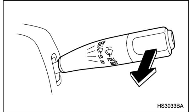
For a single wipe of the wipers, pull the lever toward you. The wipers operate until you release the lever.
