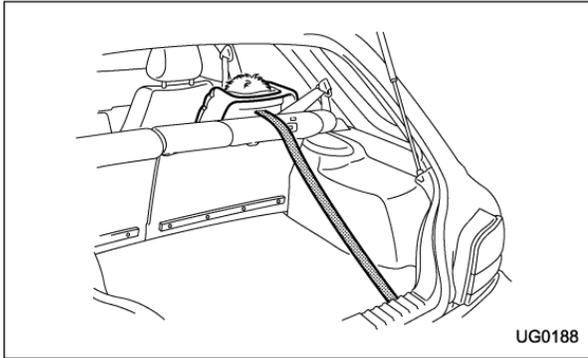
If the child restraint system requires a top tether, latch the hook onto the top tether anchor and tighten the top tether. See the “Top tether anchorages” for additional instructions.
