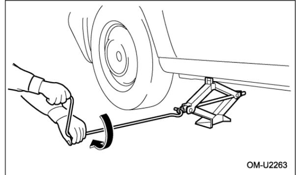
9. Insert the jack handle into the jackscrew, and turn the handle until the tire clears the ground.
