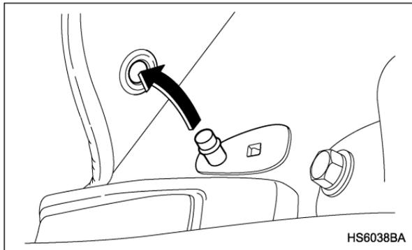
A retaining pin is located on the driver's side of the vehicle next to the fuel filler door release. The floor mat is secured using the built-in grommet, by placing the grommet over the pin and pushing downward.
