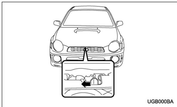
2. Release the secondary hood release located under the front grille by moving the lever toward the left.
