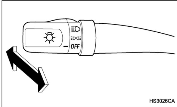
To change from low beam to high beam, push the turn signal lever forward. When the headlights are on high beam, the high beam indicator light “
