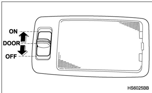
The dome light switch has three positions:
