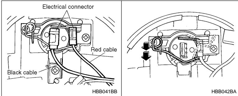
1. Disconnect the electrical connector for the black cable.
