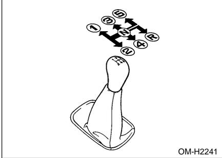
The shift pattern is shown on the shift lever knob. When shifting from 5th gear to reverse gear, first return the shift lever to the neutral position then shift into reverse gear.
