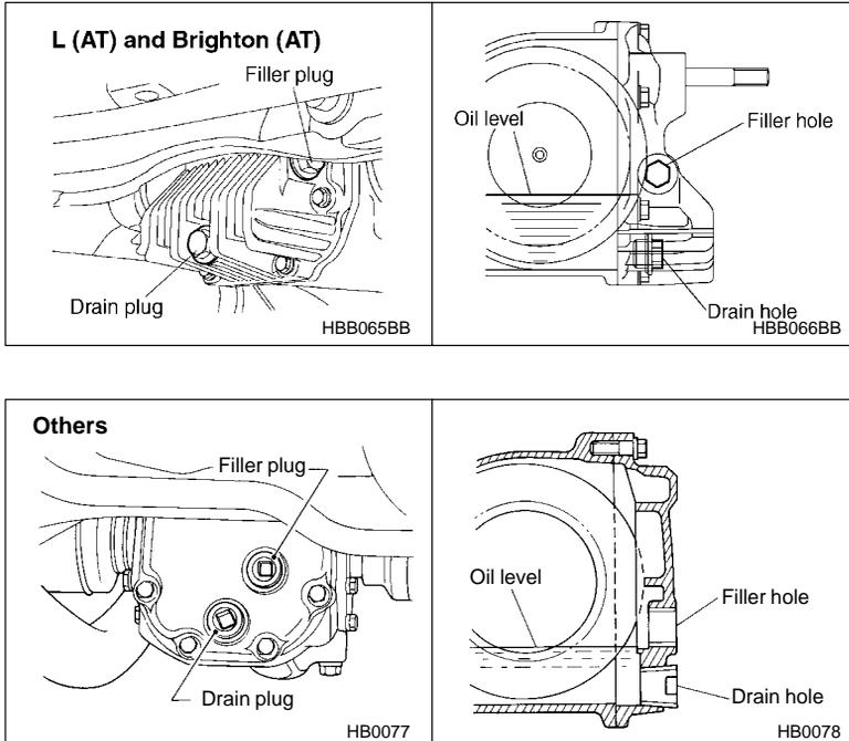
Remove the plug from the filler hole and check the oil level. The oil level should be kept even with the bottom of the filler hole. If the oil level is below the bottom edge of the hole, add oil through the filler hole to raise the level.
