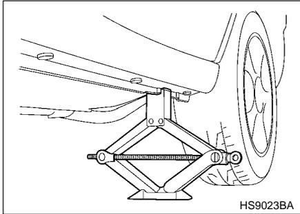
9. Insert the jack handle into the jackscrew, and turn the handle until the tire clears the ground. Do not raise the vehicle higher than necessary.
