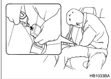
2. After confirming that the webbing is not twisted, insert the connector (tongue) attached at the webbing end into the buckle on the right-hand side until a click is heard. If the belt stops before reaching the buckle, return the belt slightly and pull it out more slowly. If the belt still cannot be unlocked, let the belt retract slightly after giving it a strong pull, then pull it out slowly again.
