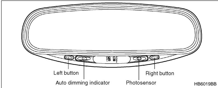
The auto-dimming mirror/compass has an anti-glare feature which automatically reduces glare coming from headlights of vehicles behind you. It also contains a built-in compass.
