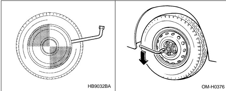
7. Loosen the wheel nuts using the wheel nut wrench but do not remove the nuts.
