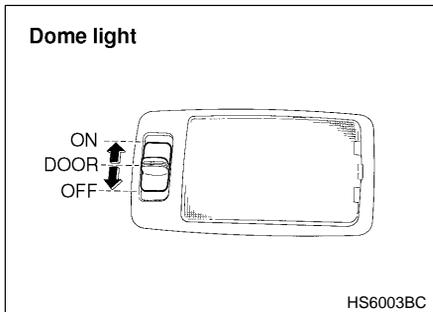
The dome light switch has three positions:
