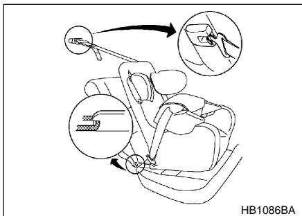
Your vehicle is equipped with four lower anchorages (bars) and three upper anchorages (tether anchorages) for accommodating such child restraint systems.
