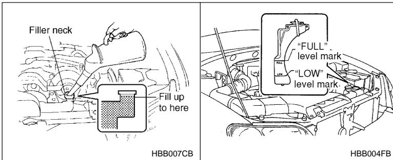
4. Slowly pour the coolant and fill to the radiator filler neck and to the reserve tank's "FULL" level mark. Do not pour the coolant too quickly, as this may lead to insufficient air bleeding and trapped air in the system.
