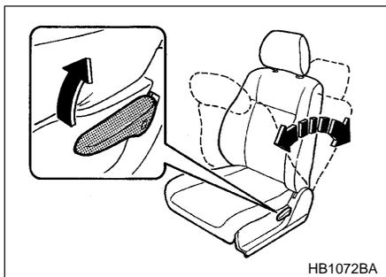
Pull the reclining lever up and adjust the seatback to the desired position. Then release the lever and make sure the seat is securely locked into place.
