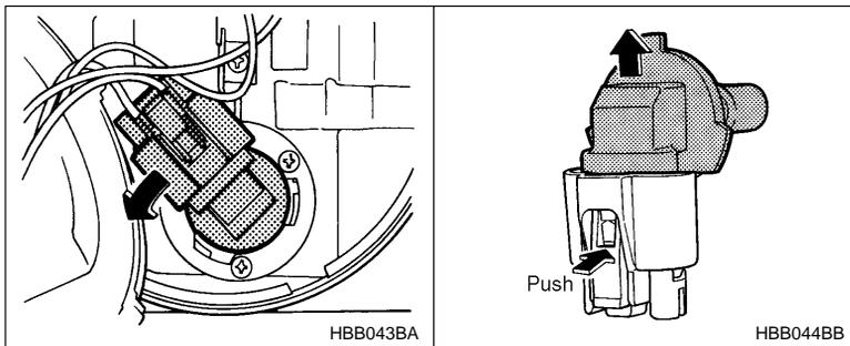
1. Disconnect the electrical connector from the bulb.
