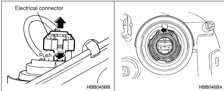
1. Disconnect the electrical connector while pressing the lock release tab.
