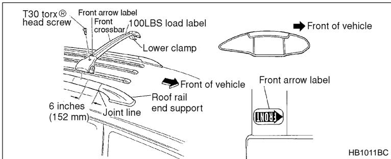
1. Before placing the crossbar on the roof rails, make sure that the T-30 torx® head screw is removed from the top of each crossbar end support.
