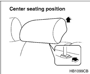
1. Remove the headrest (if so equipped) at the seating position where the child restraint system has been installed with the seatbelt or lower anchorages; lift up the headrest while pressing the release but-
