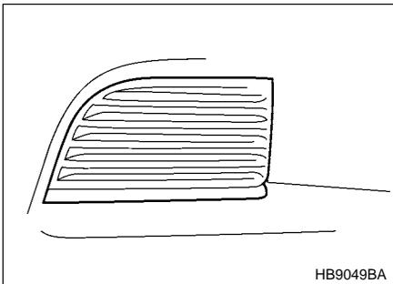
To use the towing hook, insert the top end of the flat tip screwdriver in a slot on the upper part of the cover, and remove the cover while prying it off.
