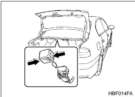
1. Remove the cover by squeezing its sides and pulling it.
