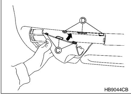
1. Insert the projection **C** into the hole **D**.
