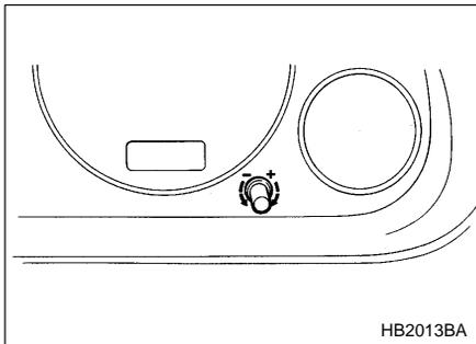
To set the time, turn the setting knob clockwise to advance and counter-clockwise to retard the time.
