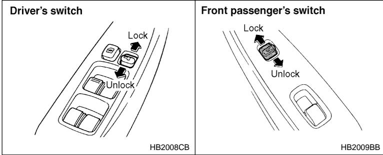
All doors and the rear gate (station wagon) can be locked and unlocked by the power door locking switches located at the driver's side and the front passenger's side doors.
