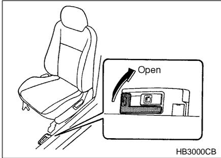
Pull the trunk lid release lever upward.
