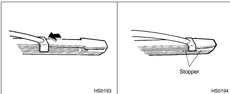
6. Install the wiper blade assembly to the wiper arm. Make sure that it locks in place.
