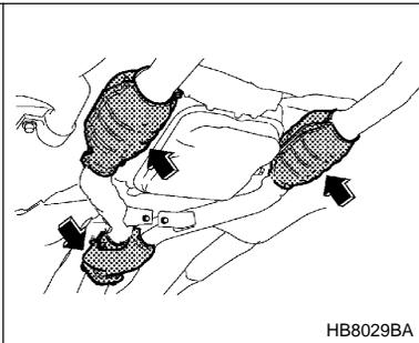
The catalytic converter is installed in the exhaust system. It serves as catalyst to reduce HC, CO and NOx in exhaust gases, thus providing cleaner exhaust.
