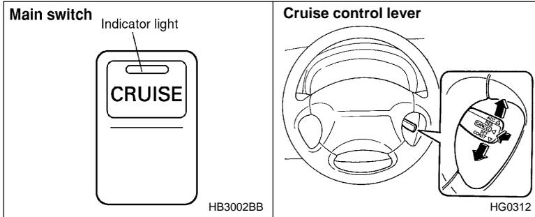
1. Push the “CRUISE” main switch. The indicator light on the switch will come on.
