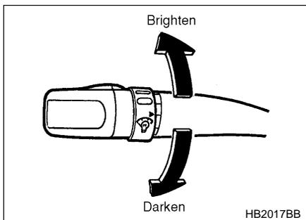
When the lighting switch is in the “☉” or “☾” position, you can adjust brightness of the instrument panel illumination for better visibility. To brighten, turn the control dial counterclockwise. To darken, turn the control dial clockwise.
