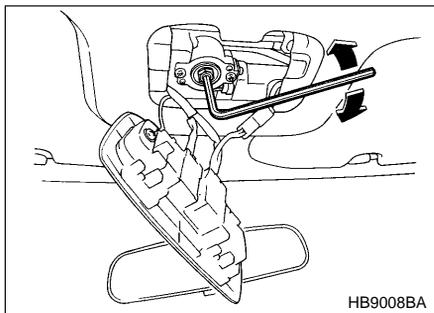
3. Insert the wrench in the end of the motor shaft.
