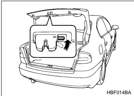
The inside trunk lid release can be cancelled to help prevent unauthorized entry into the trunk. To cancel the trunk lid release, set the lid release cancel lever (located on the inside of the trunk lid, mounted to the trunk lid latch) to the "CANCEL" position. When this lock is in the "CANCEL" position, the trunk can be opened only with the key.
