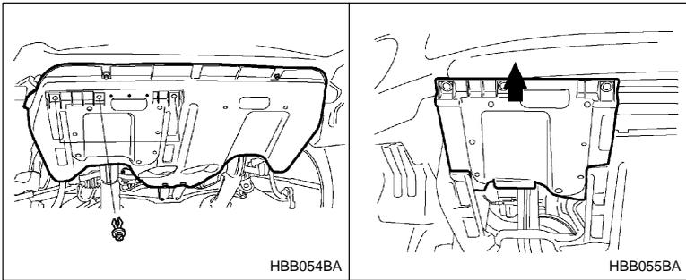
6. Remove three clips at the front of the cover under the oil filter.
