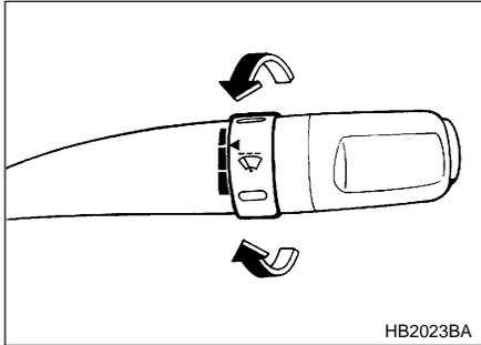
When the wiper switch is in the “
