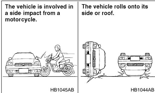
▽ **Examples of the types of accidents in which the SRS side airbag will basically not deploy.**
