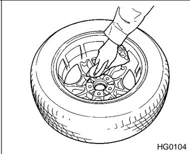
12. Put on the spare tire. Replace the wheel nuts. Tighten them by hand.
