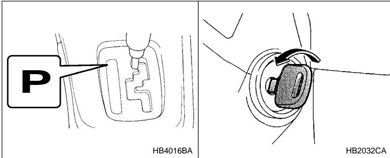
The key can be turned from "ACC" to "LOCK" only when the selector lever is in the "P" position.
