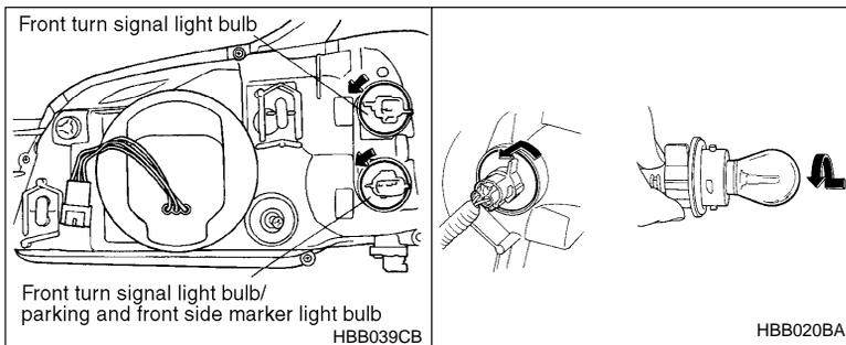
3. Remove the bulb socket from the headlight assembly by turning it counterclockwise.
