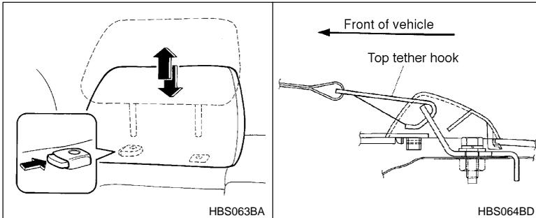
1. Remove the headrest at the seating position where the child seat has been installed with the seatbelt or lower anchorages; lift up the headrest while pressing the release button.
