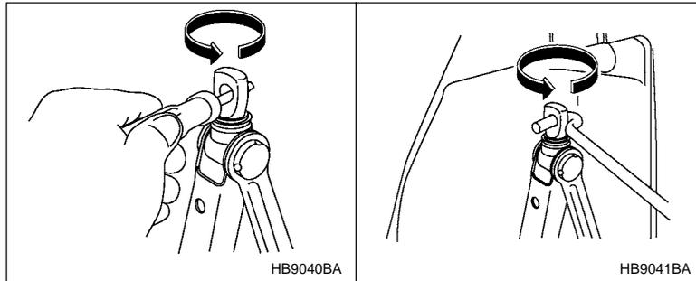
If the jackscrew is too tight to be loosened by hand, loosen it using a screwdriver or the jack handle.
