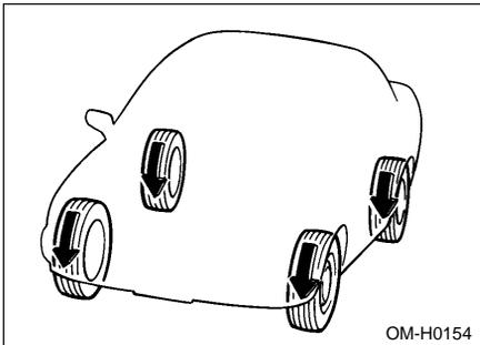
All wheel drive distributes the engine power to all four wheels. AWD vehicles provide better traction when driving on slippery, wet or snow-covered roads and when moving out of mud, dirt and sand. By shifting power between the front and rear wheels, SUBARU AWD can also provide added traction during acceleration, and added engine braking force during deceleration.
