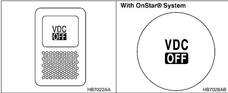
Note: Even when the lighting switch is turned to the “ $\rightarrow\text{D}\leftarrow$ ” or “ $\equiv\text{D}$ ” position, the “OFF” portion of the symbol stamped on the switch will not illuminate in the dark. Only “VDC” portion will illuminate.
