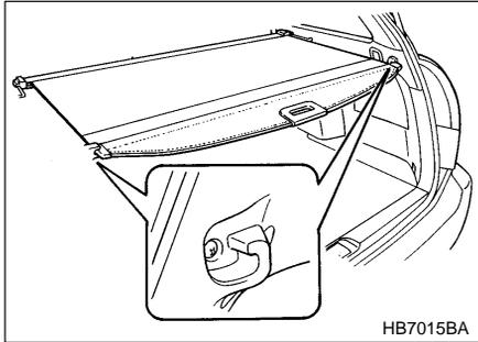
To extend the cover, pull the end of the cover out of the housing, then insert its hooks into the catches as shown. To rewind it, unhook it from the catches and it will rewind automatically. You should hold on to the cover and guide it back into the cover housing while it is rewinding.
