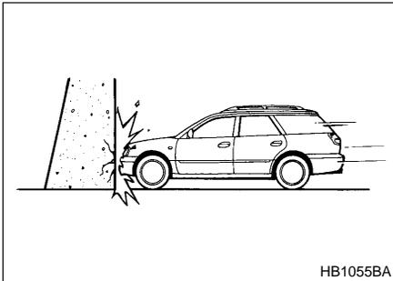
▽ **Examples of the types of accidents in which it is possible that the SRS frontal airbag will deploy.**
