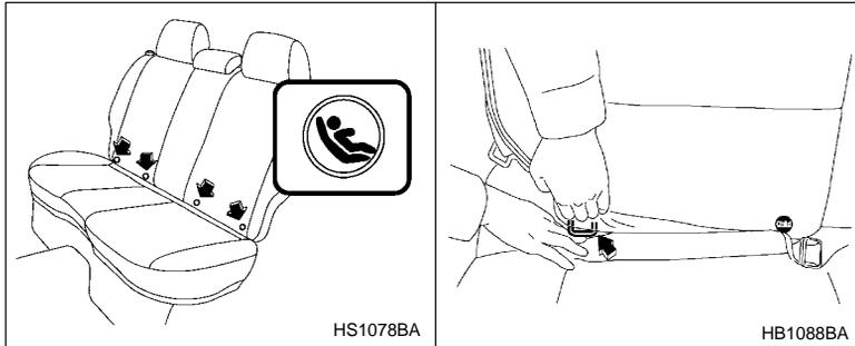
You will find marks “
