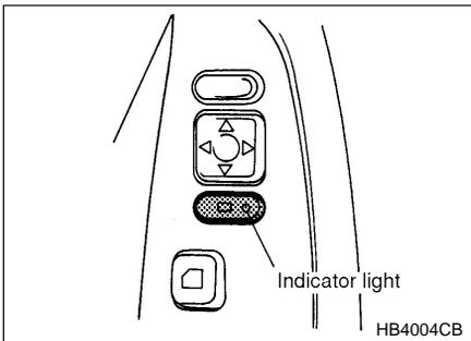
To turn on the outside mirror defogger, push the switch while the engine is running.
