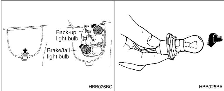
1. Unlatch the rear finisher light cover by moving the knob upward. Open the cover up.
