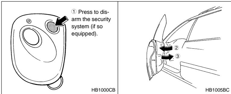
1. Disarm the security system. (if your vehicle is equipped with the optional security system.)
