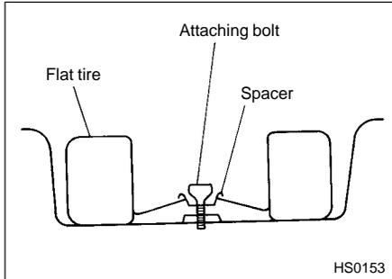
When storing a conventional tire, put the spacer upside down and tighten the attaching bolt firmly.
