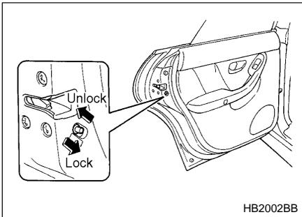
Each rear door has a child safety lock that prevents the doors from being opened even if the inside door handle is pulled.
