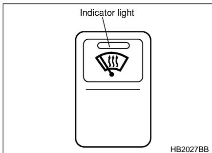
The windshield wiper deicer operates only when the ignition switch is in the “ON” position.
