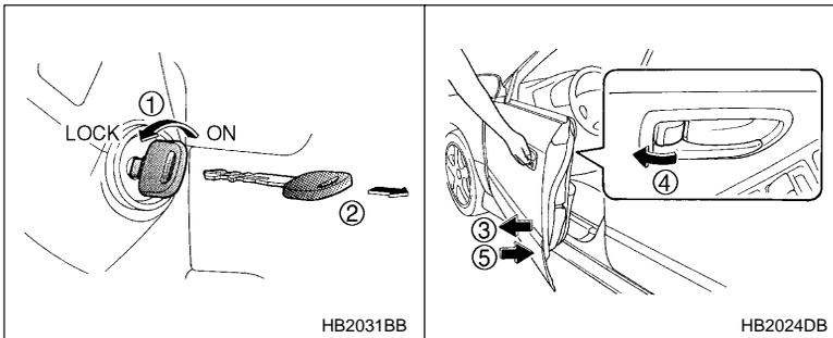
1. Turn the ignition switch to the “ON” position.
