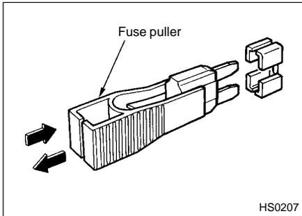
4. Pull out the fuse with the fuse puller.
