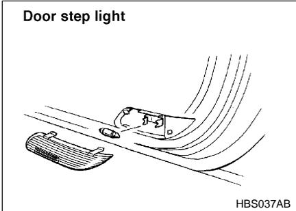
1. Remove the lens by prying the edge of the lens with a regular screwdriver.
