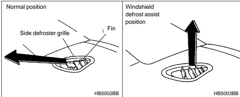
The driver's side defroster grille is adjustable. The normal position as shown in the diagram directs warm air to the side glass. When more rapid defrosting of the windshield is desired, the air flow can be directed temporarily toward the windshield to assist the windshield defroster. If this is done, the driver's side grille should always be returned to its normal position so that the warm air flow can then be used to defrost the driver's side window.
