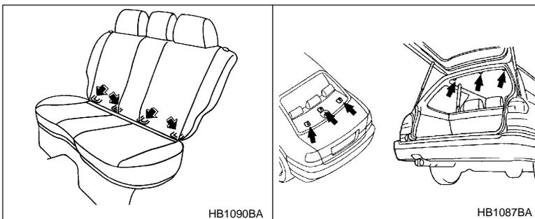
The lower anchorages (bars) are used for installing a child restraint system only on the rear seat window-side seating positions. For each window-side seating position, two lower anchorages are provided.
