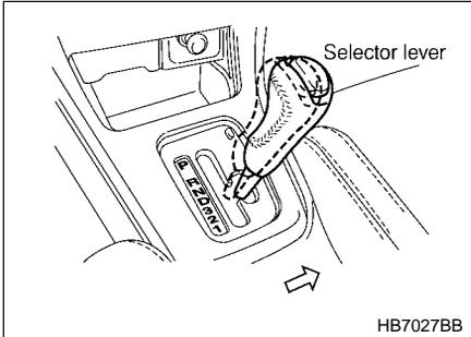
2. Once the SPORTSHIFT mode is selected, the currently selected gear is shown by the shift position indicator in the meter cluster. Next to this indication, arrow-shaped lamps show whether an upshift is possible and whether a downshift is possible.
