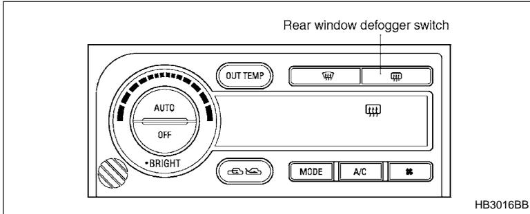
To turn on the defogger, push the switch. To turn it off, push the switch again.
