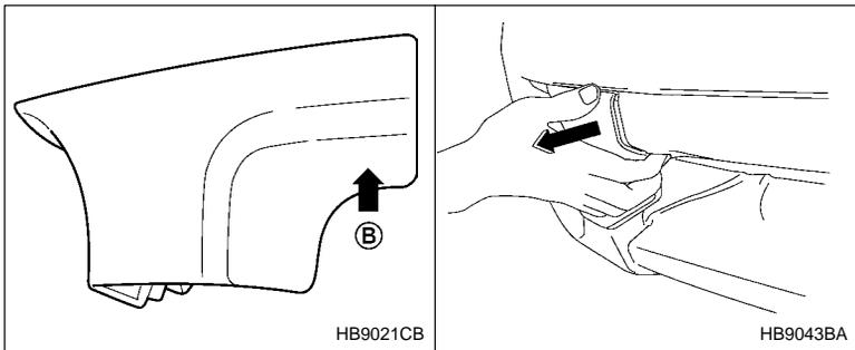
2. Press portion **B** and simultaneously pull the towing hook cover toward you.
