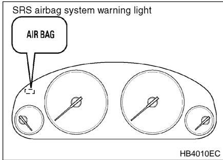
A diagnostic system continually monitors the readiness of the seatbelt pretensioner while the vehicle is being driven. The seatbelt pretensioners share the control module with the airbag system. Therefore, if any malfunction occurs in a seatbelt pretensioner, the SRS airbag system warning light will illuminate. The SRS airbag system warning light will show normal system operation by lighting for about 6 seconds when the ignition key is turned to the "ON" position.
