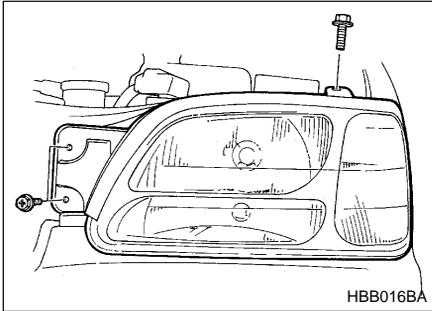
1. Remove the headlight assembly mounting screws located at the top of and the front of the headlight assembly using a phillips screwdriver or an open-end wrench.
