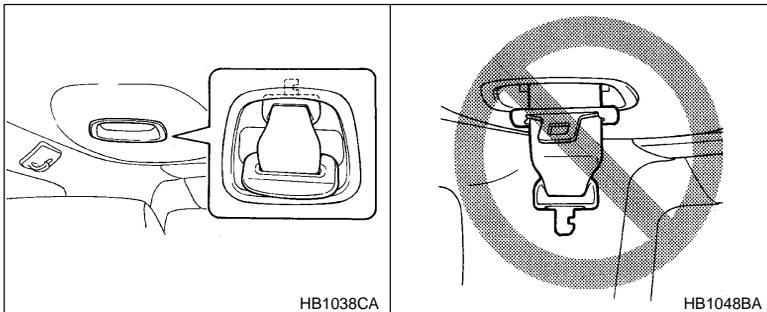
2. Allow the retractor to roll up the belt. You should hold the webbing end and guide it back into the retractor while it is rolling up. Neatly store the tongue plates in the recess in the retractor and then insert the connector (tongue) plate into the slot located at the front of the recess.
