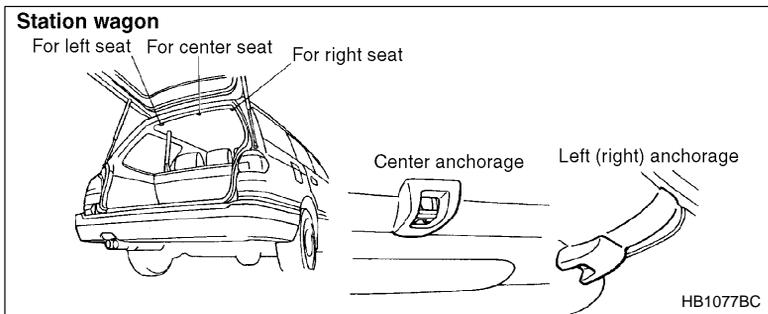
Three anchorages, i.e., ones for the right, center and left positions, are already installed on the rear shelf (on Sedan) or on the rear edge of the roof (on Station wagon).
