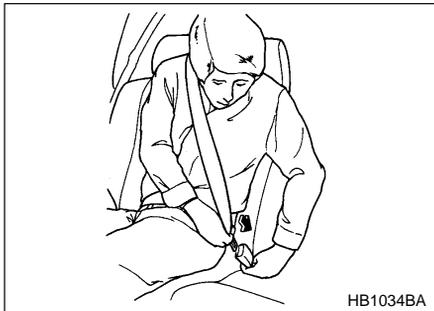
3. Insert the center seatbelt tongue plate in the center seatbelt buckle marked "CENTER" on the left-hand side until it clicks. To make the lap part tight, pull up on the shoulder belt. And place the lap belt as low as possible on your hips, not on your waist.
