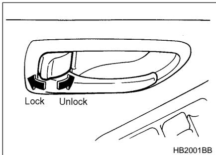
To lock the door from the inside, rotate the lock lever rearward. To unlock the door from the inside, rotate the lock lever forward.
