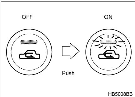
**ON position (Recirculation):** Interior air is recirculated inside the vehicle. Push the air inlet selection button to the ON position. The indicator light will come on.
