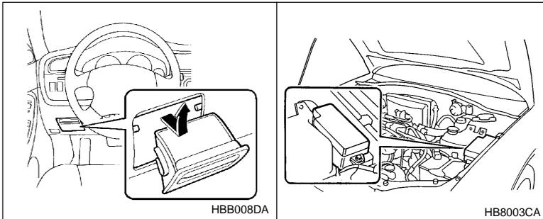
The fuses are designed to melt during an overload to prevent damage to the wiring harness and electrical equipment. The fuses are located in two fuse boxes. One is located under the instrument panel behind the coin tray on the driver's seat side. The other one is housed in the engine compartment. The fuse puller and spare fuses are stored in the main fuse box cover in the engine compartment.
