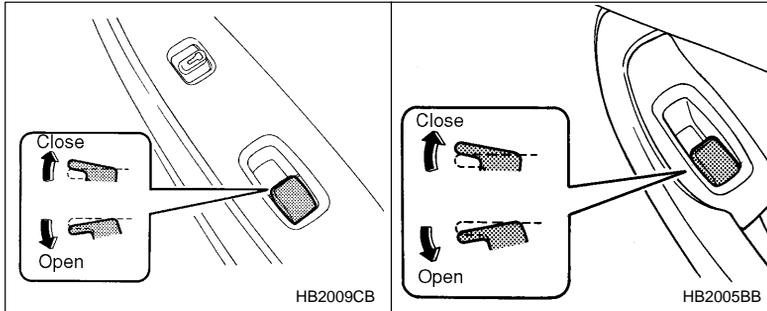
To open the window, push the switch down and hold it until the window reaches the desired position. To close the window, pull the switch up and hold it until the window reaches the desired position.
