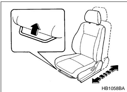
Pull the lever upward and slide the seat to the desired position. Then release the lever and move the seatback and forth to make sure that it is securely locked into place.
