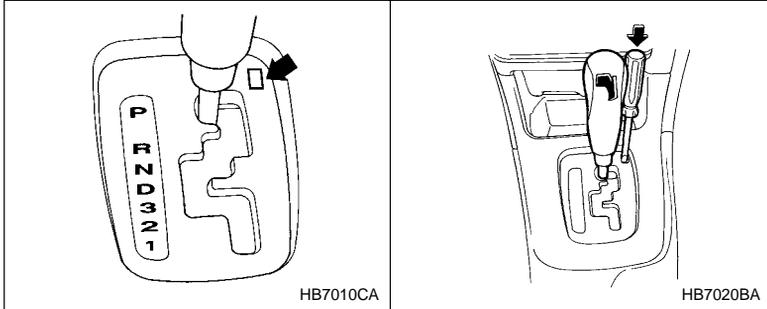
4. Insert the screwdriver into the hole.
