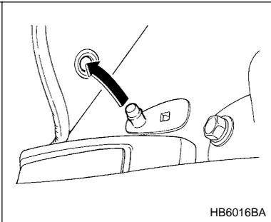
A retaining pin is located on the driver's side of the vehicle next to the fuel filler door release. The floor mat is secured using the built-in grommet, by placing the grommet over the pin and pushing downward.
