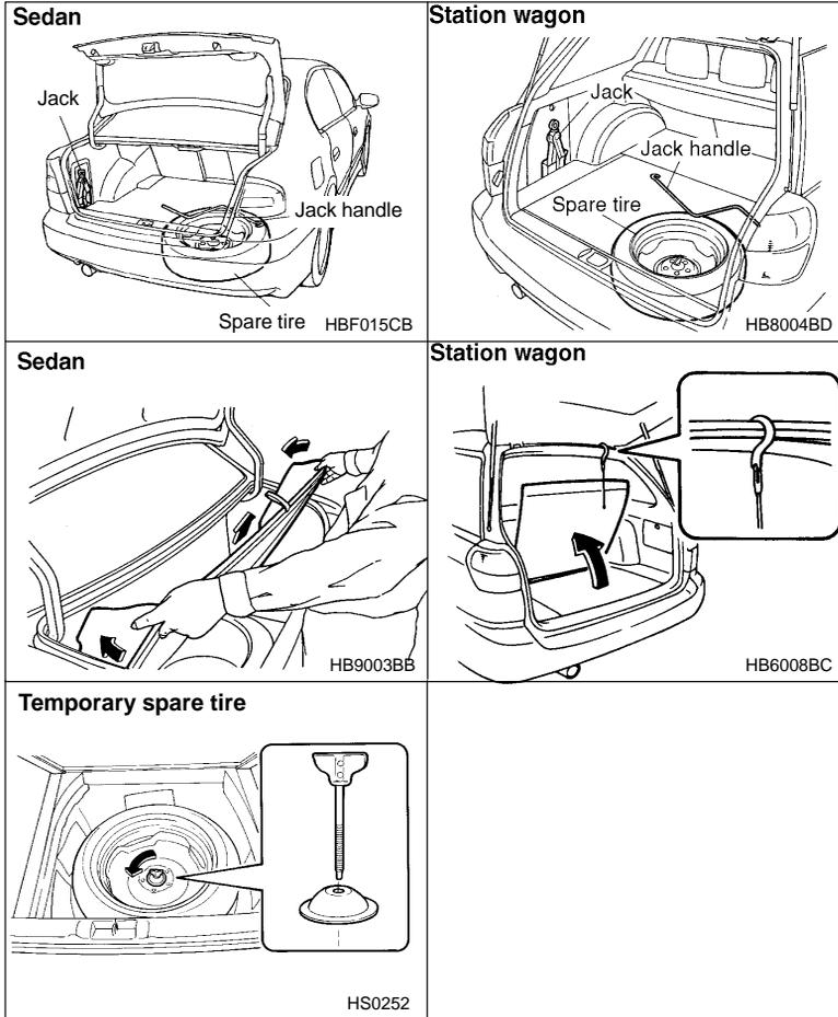
The spare tire is stored under the floor of the trunk or cargo area.
