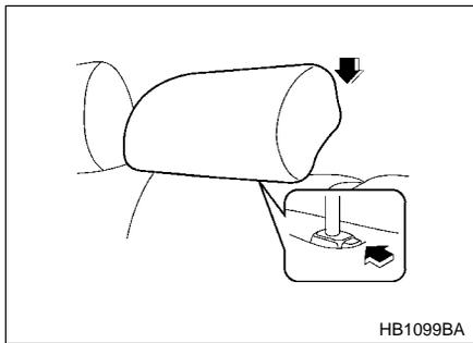
To raise the headrest, pull it up. To lower it, push the headrest down while pressing the release button on the top of the seatback.
