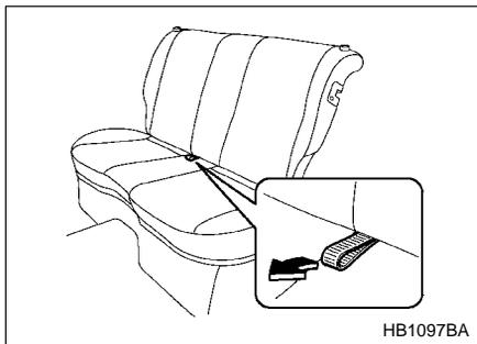
6. Unlock the seatback by pulling the release knob and fold the seatback down. Confirm that the pin located at the bottom of the seat cushion is inserted into the slot at the top of the seatback.
