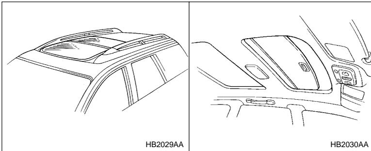
The front moonroof has a tilting function and the rear moonroof has a sliding function.
