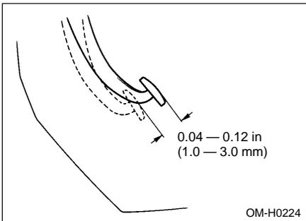
Stop the engine and firmly depress the brake pedal several times. Lightly press the brake pedal down with one finger to check the free play with a force of less than 2 lb (10 N, 1 kg). If the free play is not within proper specification, contact your SUBARU dealer.
