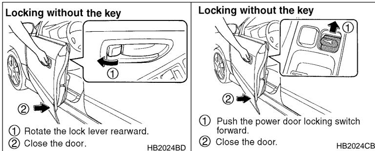
To lock the door from the outside without the key, rotate the lock lever rearward and then close the door.
