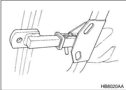
5. Use only a hitch ball that is appropriate for the ball mount and your trailer. The hitch ball must be securely installed on the ball mount.
