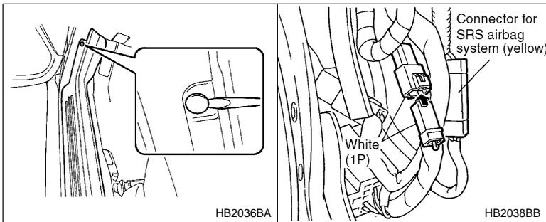
1. Remove the side sill cover on the driver's side.
