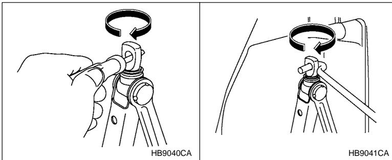
After placing the jack in its storage location, turn the jackscrew clockwise by hand until it becomes too hard to turn. Then, tighten it by an additional 1/4 – 1/3 of a turn using a screwdriver or the jack handle. Unless the jack is properly secured, it may rattle while the vehicle is moving.
