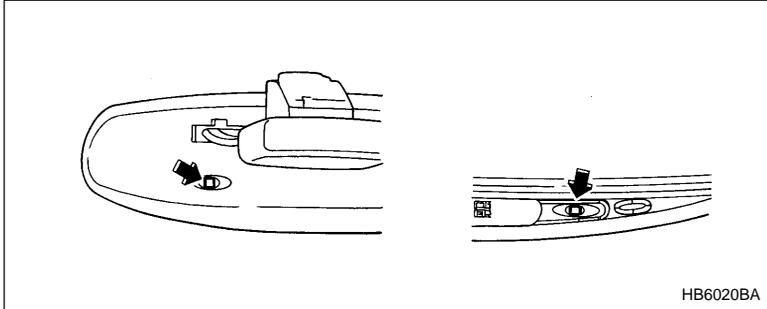
The mirror has a photosensor attached on both the front and back sides. If the glare from the headlights of vehicles behind you strikes the mirror, these sensors detect it and make the reflection surface of the mirror dimmer to help prevent you from being blinded. For this reason, use care not to cover the sensors with stickers, or other similar items. Periodically wipe the sensors clean using a piece of dry soft cotton cloth or an applicator.
