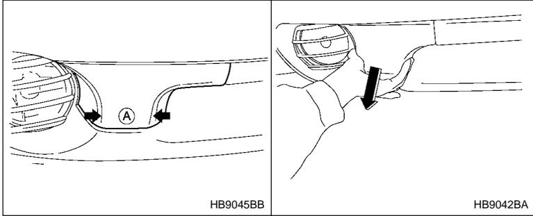
1. Squeeze the sides of portion **A** and pull the towing hook cover toward you.
