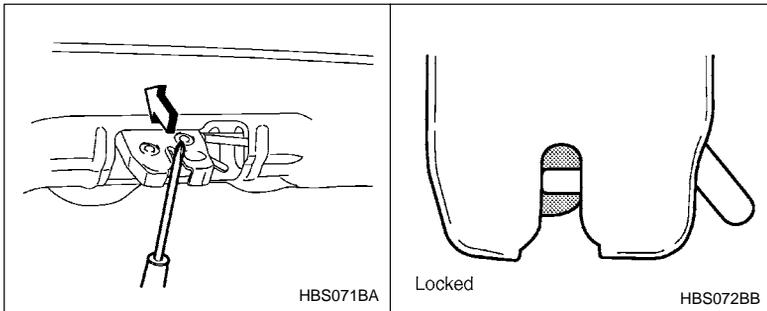
2. Use a screwdriver with a thin blade. Slide the screwdriver blade from the slit aperture of the lock assembly fully to the end until you hear a click. This places the latch in the locked position.
