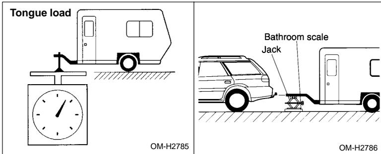
The tongue load can be adjusted by proper distribution of the load in the trailer. Never load the trailer with more weight in the back than in the front; approximately 60 percent of the trailer load should be in the front and approximately 40 percent in the rear. Also, distribute the load as evenly as possible on both the left and right sides. Be sure that all cargo is firmly secured to prevent a change in weight distribution while driving.
