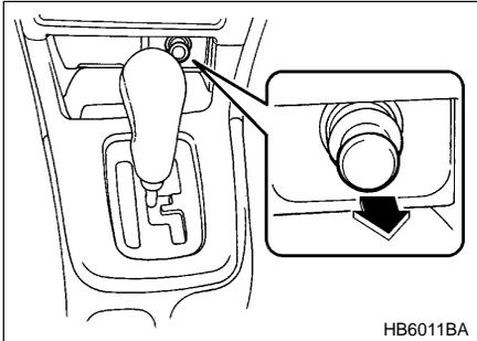
The electrical power socket located on the lower part of the instrument panel can be used as cigarette lighter socket. A cigarette lighter plug is an optional accessory. It is available from your SUBARU dealer. The cigarette lighter socket may also be used as a power source for an in-car use electrical appliance.
