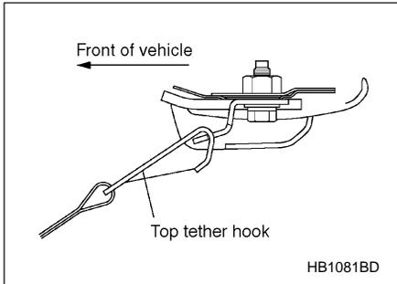
2. Fasten the top tether hook of the child restraint system to the appropriate upper anchorage.
