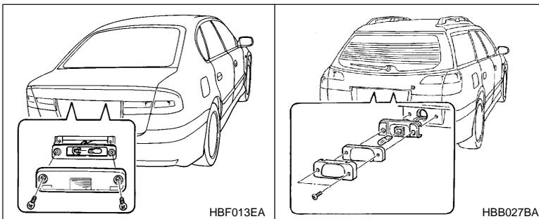
1. Remove the mounting screws using a phillips screwdriver.
