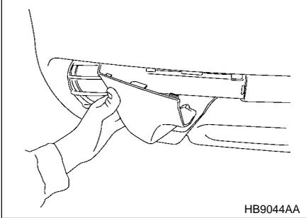
3. Turn the towing hook cover clockwise, pivoting it about the side that is next to the fog lamp. Pull out the towing hook cover to remove it.
