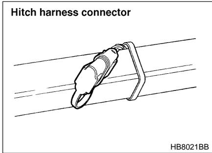
9. Confirm proper function of the hitch wire harness by individually activating the brake, right turn signal, left turn signal, stop, and parking lights on the trailer.
