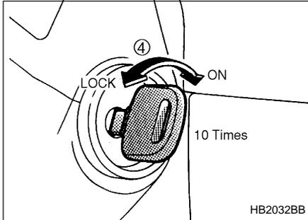
4. Place the ignition key into the ignition switch and cycle the switch from LOCK to ON ten times **within 15 seconds**. Be sure to stop at the LOCK position. The horn will sound once to indicate that you are in the transmitter programming mode.
