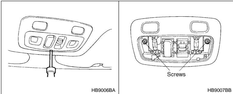
2. Remove the map light lens by prying the edge of the lens with a regular screwdriver, then remove the switch body retaining screws and take off the moonroof switch.
