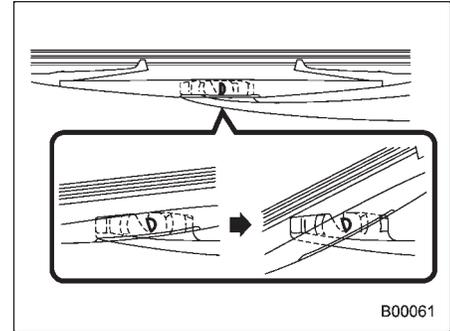
2. Turn the wiper blade assembly counterclockwise.
