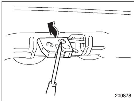
2. Use a screwdriver with a thin blade. Slide the screwdriver blade from the slit aperture of the lock assembly fully to the end until you hear a click.
