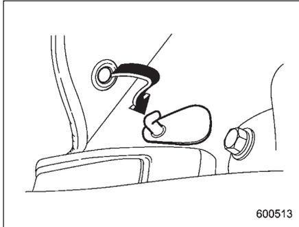
A retaining pin is located on the driver's side of the vehicle next to the fuel filler door release.
