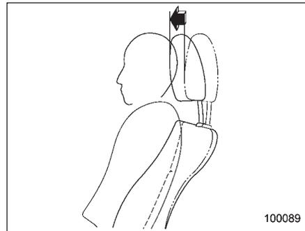
The front seats of your vehicle are equipped with active head restraints. They automatically tilt forward slightly in the event the vehicle is struck from the rear, decreasing the amount of rearward head movement and thus reducing the risk of whiplash. For maximum effectiveness, the head restraint should be adjusted so that the center of the head restraint is closest to the top of the occupant's ears.
