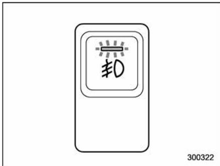
The front fog lights operate only when the headlights are on low beam. Push the front fog light button to turn the front fog lights on.
