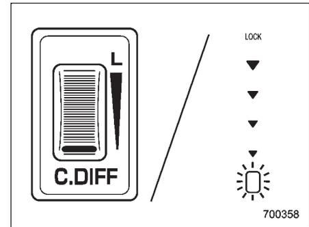
Turn the dial rearward to reduce the initial LSD torque; when the white line reaches the rearmost position, the initial LSD torque will be minimum and the "O" indicator light will come on. Under this condition, only the Mechanical LSD torque will limit the differential action.
