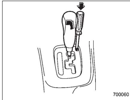
4. Insert the screwdriver into the hole.
