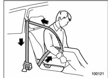
The driver's and front passenger's seatbelts have a seatbelt pretensioner. The seatbelt pretensioners are designed to be activated in the event of an accident involving a moderate to severe frontal collision.
