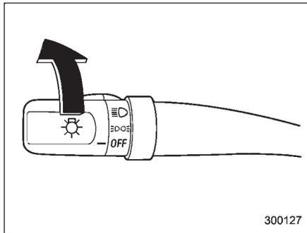
To turn on the headlights, turn the knob on the end of the turn signal lever.
