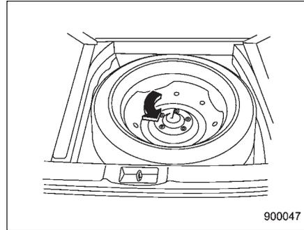
**Sedan:** Remove the floor cover from the trunk. Turn the attaching bolt counterclockwise, then take the spare tire out.
