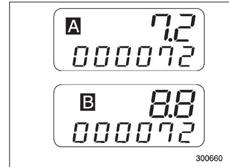
The trip meter shows the distance that the vehicle has been driven since you last set it to zero.
