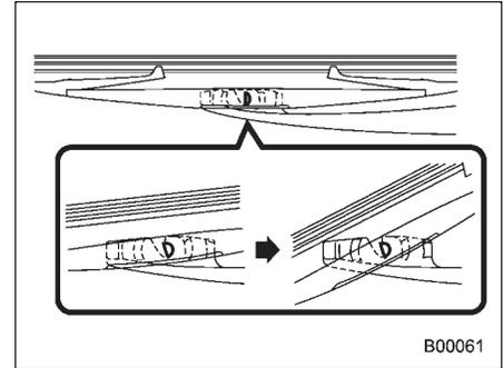
2. Turn the wiper blade assembly counterclockwise.
