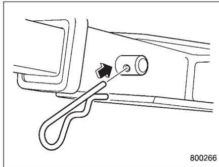
3. Insert the safety pin securely into the hitch pin.
