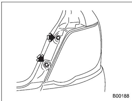
3. Remove the upper and lower bolts. Then, slide the rear combination lamp assembly to the rear and remove it from the vehicle.
