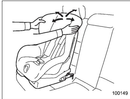
5. Before seating a child in the child restraint system, try to move seat back and forth and right and left to verify that it is held securely in position.
