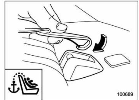
1. Attach the child restraint top tether hook to the appropriate upper anchorage.
