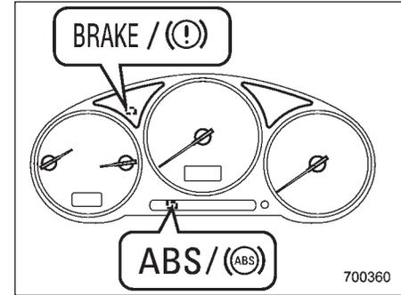
If a malfunction occurs in the EBD system, the system stops working and the brake system warning light and ABS warning light come on simultaneously.
