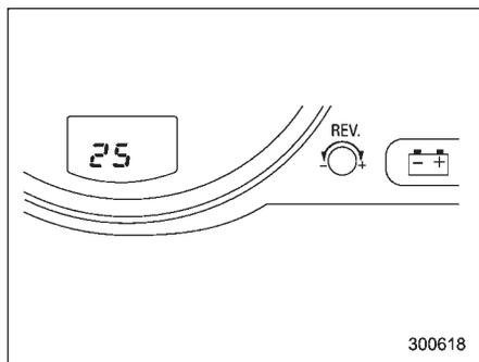
1. Turn the REV setting knob clockwise or counterclockwise, then release it and let it return to its initial position. The buzzer will sound. The REV alarm system is now ready to be set.
