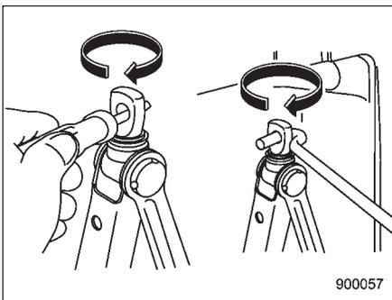
After placing the jack in its storage location, turn the jackscrew clockwise by hand until it becomes too hard to turn. Then, tighten it by an additional 1/4 – 1/3 of a turn using a screwdriver or the jack handle. Unless the jack is properly secured, it may rattle while the vehicle is moving.
