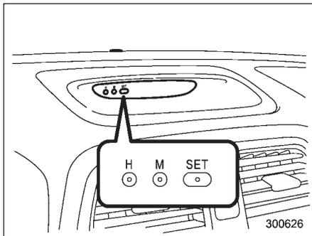
To set the hour, press the “H” button. To set the minutes, press the “M” button. To reset the minutes to “00” with a radio time signal, push the “SET” button.
