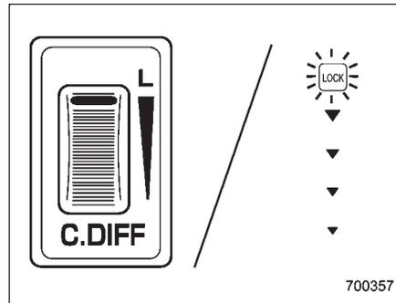
Turn the dial forward to increase the initial LSD torque; when the white line on the dial reaches the frontmost position, the initial LSD torque setting is maximum. The center differential will then be almost completely locked and the "LOCK" indicator light will come on.
