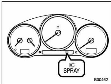
Add water to the intercooler water spray tank when the intercooler water spray warning light in the combination meter comes on. The warning light comes on when the water in the tank has decreased to approximately 0.4 liters (0.4 US qt, 0.4 Imp qt).
