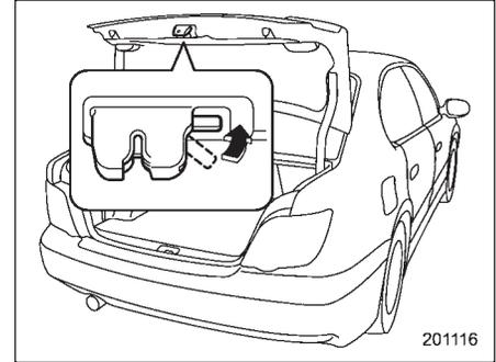
The inside trunk lid release can be canceled to prevent unauthorized entry into the trunk. To cancel the trunk lid release, set the lid release cancel lever (located on the inside of the trunk lid, mounted to the trunk lid latch) to the "CANCEL" position. When this lock is in the "CANCEL" position, the trunk can be opened only with the key.
