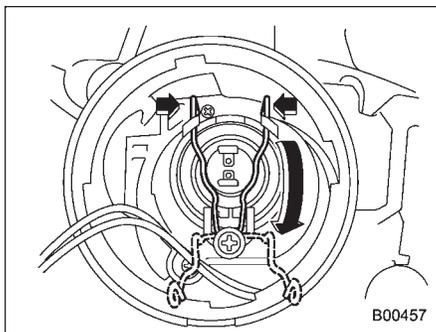
3. Remove the retainer spring.
