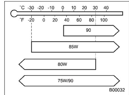
SAE viscosity No. and applicable temperature
