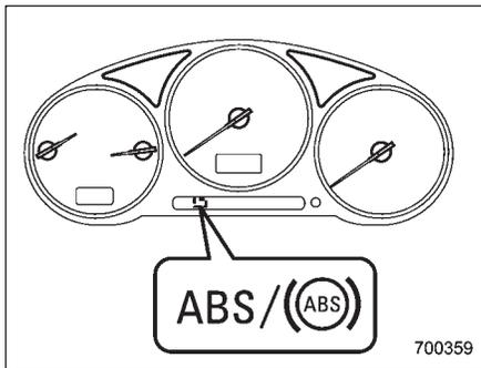
The ABS warning light comes on when the ignition switch is turned to the "ON" position and goes out after approximately 2 seconds.
