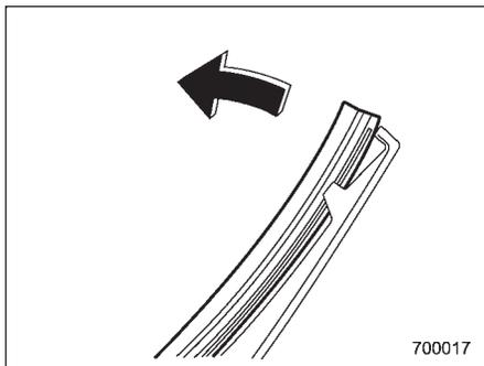
1. Pull out the end of the blade rubber assembly from the plastic support.
