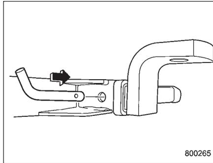
2. Insert the hitch pin into the hole on the hitch receiver tube so that the pin passes through the ball mount.
