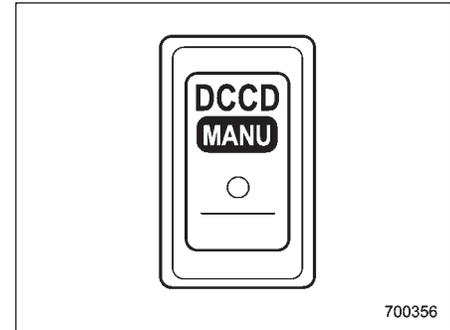
Press the "DCCD-MANU" switch on the center console to switch from auto mode to manual mode. The "AUTO" indicator light in the combination meter will go off. Press the switch again to go back to auto mode. The "AUTO" indicator light in the combination meter will come on.
