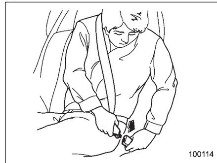
4. Insert the center seatbelt tongue plate into the center seatbelt buckle marked "CENTER" on the left-hand side until it clicks.
