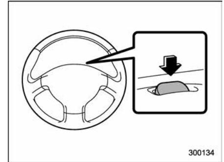
The parking light switch operates regardless of the ignition switch position.
