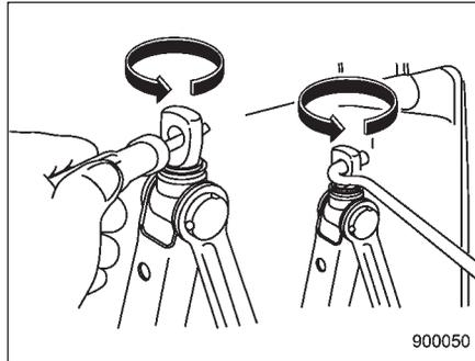
If the jackscrew is too tight to be loosened by hand, loosen it using a screwdriver or the jack handle.
