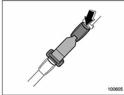
To connect the extender to the seatbelt, insert the tongue plate into the seatbelt buckle so that the “PRESS” signs on the buckle-release buttons of the extender and the seatbelt are both facing outward as shown in the diagram. You will hear a click when the tongue plate locks into the buckle.
