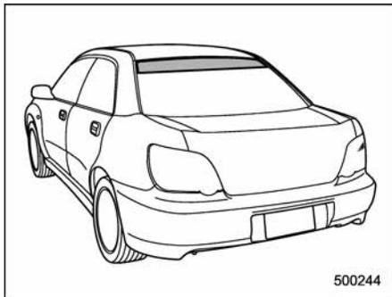
The antenna is printed on the inner surface of the rear window glass.
