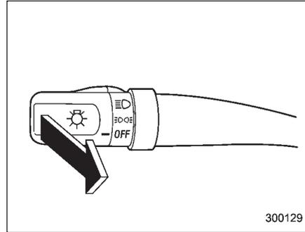
To flash the headlights, pull the lever toward you and then release it. The high beam will stay on for as long as you hold the lever. The headlight flasher works even though the light switch is in the “OFF” position.
