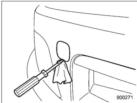
2. Pry off the cover on the front bumper using a screwdriver, and you will find a threaded hole for attaching the towing hook.
