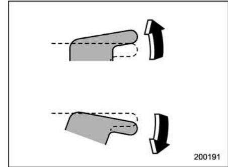
To open the passengers' windows, push the appropriate switch down and hold it until the window reaches the desired position.
