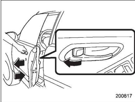
4. Before closing the doors, lock all doors with the inside door lock levers.
