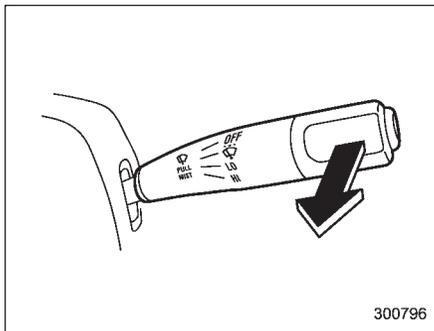
For a single wipe of the wipers, pull the lever toward you. The wipers operate until you release the lever.
