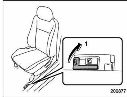
Pull the trunk lid release lever upward.
