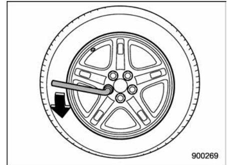
6. Loosen the wheel nuts using the wheel nut wrench but do not remove the nuts.
