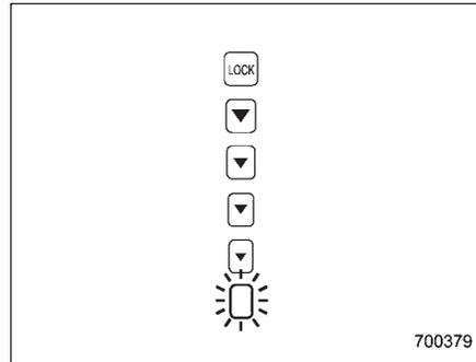
The bottom indicator light "☺" flashes in the event of failure of the driver's control center differential. Have the vehicle inspected by your SUBARU dealer. For details, refer to Chapter 7, "Driver's Control Center Differential (DCCD) (WRX-STI)".
