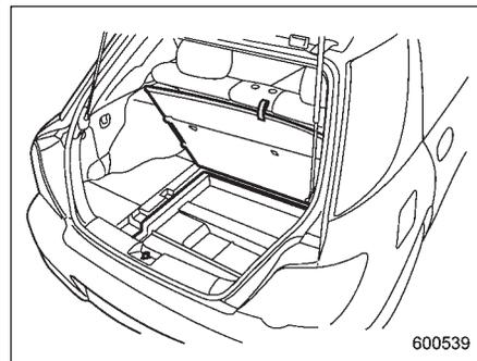
The storage compartment is located under the floor of the cargo area and can be used to store small items. To open the lid, pull the tab up.
