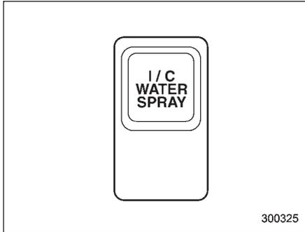
Water is sprayed for approximately 2 seconds every time the switch is pressed and then released.
