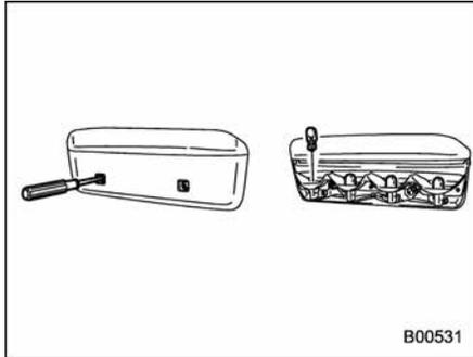
1. Remove the mounting screws using a Phillips screwdriver and then remove the high mount stop light cover.
