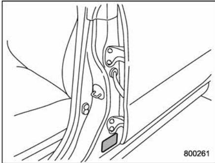
The certification plate attached to the driver's side doorjamb shows GVWR (Gross Vehicle Weight Rating) and GAWR (Gross Axle Weight Rating).
