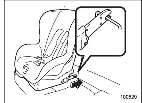
2. While following the instructions supplied by the child restraint system manufacturer, connect the lower hooks onto the lower anchorages located at “Ⓢ” marks on the bottom of the rear seatback. When the hooks are connected, make sure the adjacent seatbelts are not caught.
