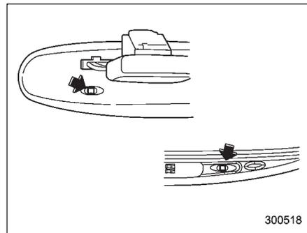
The mirror has a photosensor attached on both the front and back sides. If the glare from the headlights of vehicles behind you strikes the mirror, these sensors detect it and make the reflection surface of the mirror dimmer to help prevent you from being blinded. For this reason, use care not to cover the sensors with stickers, or other similar items. Periodically wipe the sensors clean using a piece of dry soft
