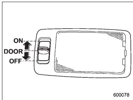
The dome light switch has three positions:
