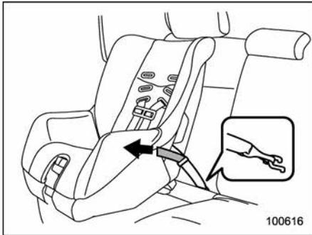
3. [If your child restraint system is of a flexible attachment type (which uses tether belts to connect the child restraint system properly to the lower anchorages)] While pushing the child restraint into the seat cushion, pull both left and right lower tether belts up to secure the child restraint system firmly by taking up the slack in the belt.
