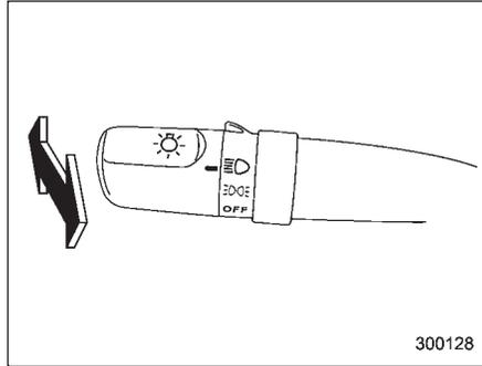
To change from low beam to high beam, push the turn signal lever forward. When the headlights are on high beam, the high beam indicator light “
