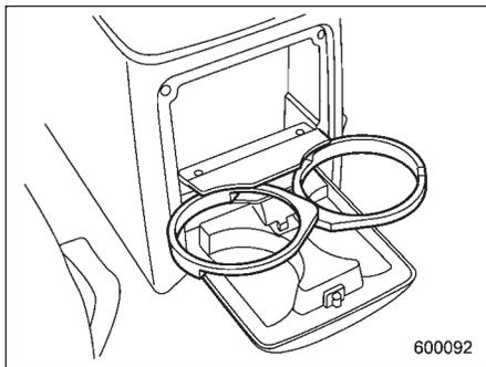
A dual cup holder is located at the back of the center console. To use the cup holder, open the lid by pulling its upper edge.
