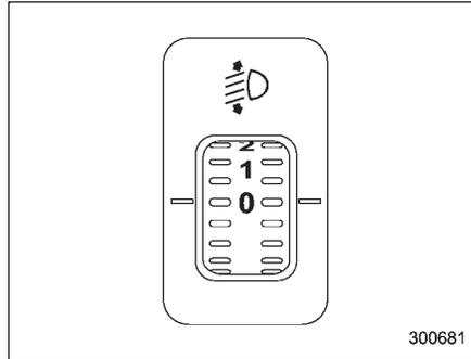
The WRX-STI version has High-Intensity Discharge (HID) headlights on the low beam setting. The HID headlights generate more light than conventional halogen headlights. Therefore a driver of an oncoming vehicle may experience too much glare when your headlight beam height adjustment is high due to the vehicle carrying heavy load.
