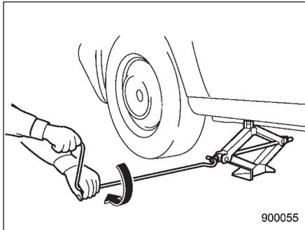
8. Insert the jack handle into the jackscrew, and turn the handle until the tire clears the ground. Do not raise the vehicle higher than necessary.
