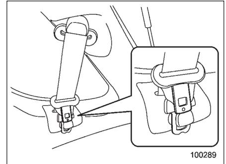
2. Allow the retractor to roll up the belt.
