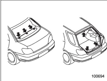
The tether anchorages (upper anchorages) are provided for all the seating positions (center and both window-side ones) of the rear seat.
