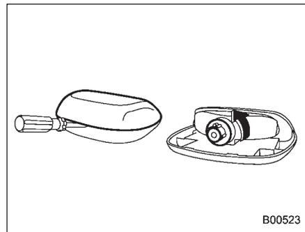
1. Remove the high mount stop light cover by prying the edge with a screwdriver.
