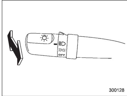
To change from low beam to high beam, push the turn signal lever forward. When the headlights are on high beam, the high beam indicator light "HID" on the instrument panel is also on.
