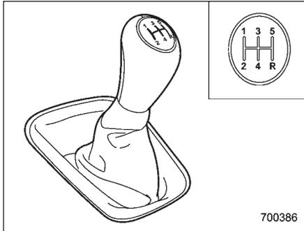
The manual transmission is a fully synchromeshed, 5-forward-speed and 1-reverse-speed transmission.
