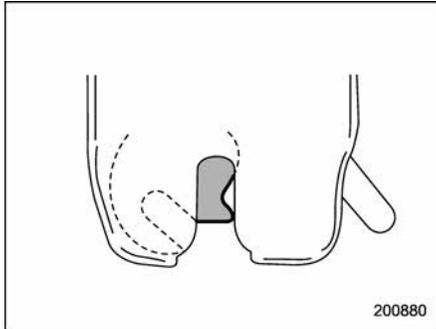
3. Move the release handle, from outside the vehicle, in the direction of the arrow to check if the latch is released.
