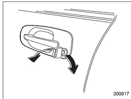
To lock the driver's door from the outside with the key, turn the key toward the rear. To unlock the door, turn the key toward the front.
