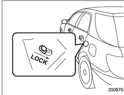
Each rear door has a child safety lock that prevents the doors from being opened even if the inside door handle is pulled.
