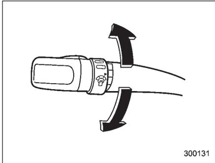
When the headlight switch is in the “☰” or “☷” position, you can adjust brightness of the instrument panel illumination for better visibility.
