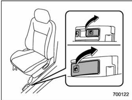
1. To open the fuel filler lid, pull the lid release lever up. The lever is on the floor at the left of the driver's seat.
