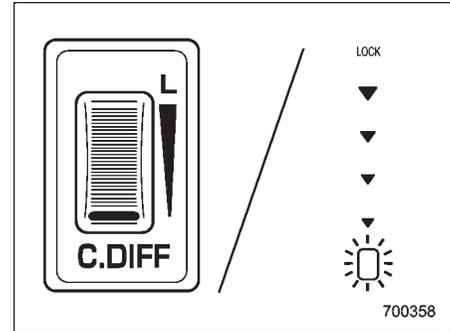
Turn the dial rearward to reduce the initial LSD torque; when the white line reaches the rearmost position, the initial LSD torque will be minimum and the "L" indicator light will come on. Under this condition, only the Mechanical LSD torque will limit the differential action.
