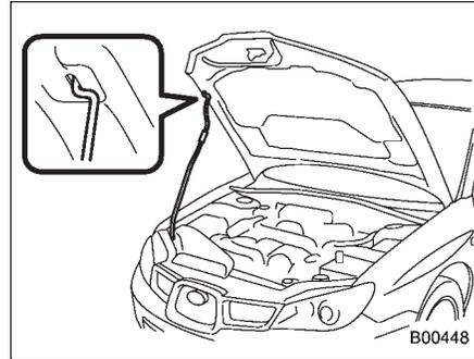
Lift up the hood, release the hood prop from its retainer and put the end of the hood prop into the slot in the hood.
