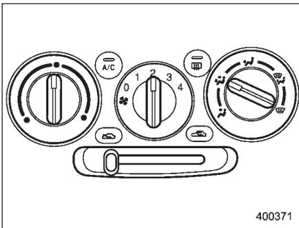
This setting allows you to direct air of different temperatures from the instrument panel and foot outlets. The air from the foot outlets is slightly warmer than from the instrument panel outlets.
