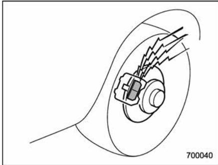
The right front disc brake and the right rear disc brake have audible wear indicators on the brake pads. If the brake pads wear close to their service limit, the wear indicator makes a very audible scraping noise when the brake pedal is applied.
