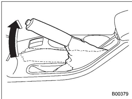
Check the parking brake stroke according to the maintenance schedule in the “Warranty and Maintenance Booklet”. When the parking brake is properly adjusted, braking power is fully applied by pulling the lever up seven to eight notches gently but firmly (approximately 44 lbs [196 N, 20 kg]). If the parking brake lever stroke is not within the specified range, have the brake system checked and adjusted at your SUBARU dealer.
