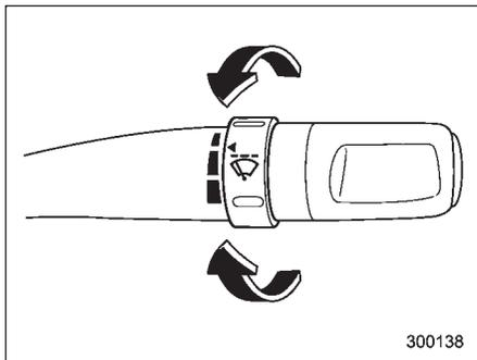
When the wiper switch is in the "OFF" position, turn the dial to adjust the operating interval of the wiper.
