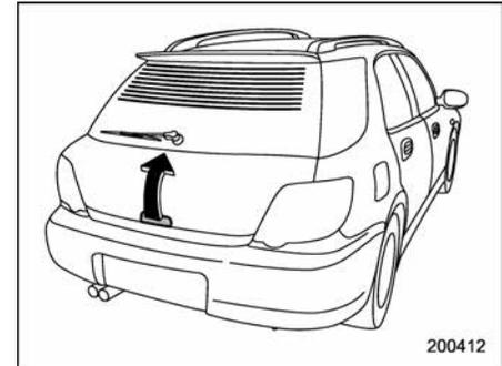
The rear gate can be locked and unlocked using either the keyless entry system or the power door locking switches.
