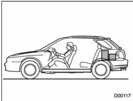
Vehicle capacity weight of the vehicle is 900 lbs (408 kg), which is indicated on the vehicle placard with the statement “The combined weight of occupants and cargo should never exceed
