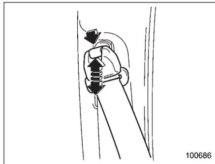
The shoulder belt anchor height should be adjusted to the best position for the passenger. To adjust the anchor height, push the release button and slide the anchor up or down. Pull down on the anchor to make sure that it is locked in place.
