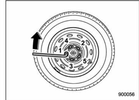
13. Use the wheel nut wrench to securely tighten the wheel nuts to the specified torque, following the tightening order in the
