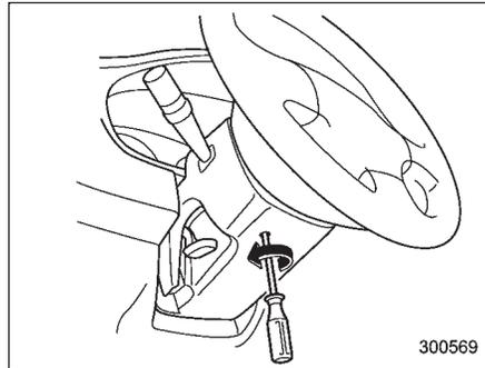
2. Remove the cover under the steering column using a Phillips screwdriver.
