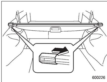
2. Pull either sleeve on the end of the cover housing to shorten the cover's length.
