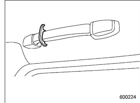
The coat hook is attached to the rear left and rear right passenger's hand grip.
