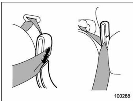
2. After drawing out the seatbelt, pass it through the belt guide as follows: First insert one edge of the belt into the open gap in the belt guide; then slide the rest of the belt in, so that the whole belt fits inside.
