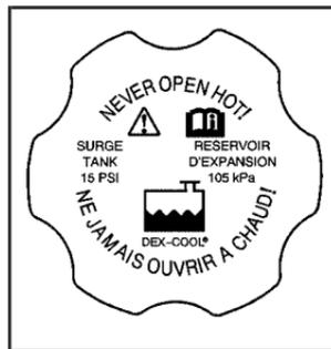
1. You can remove the coolant surge tank pressure cap when the cooling system, including the coolant surge tank pressure cap and upper radiator hose, is no longer hot.
