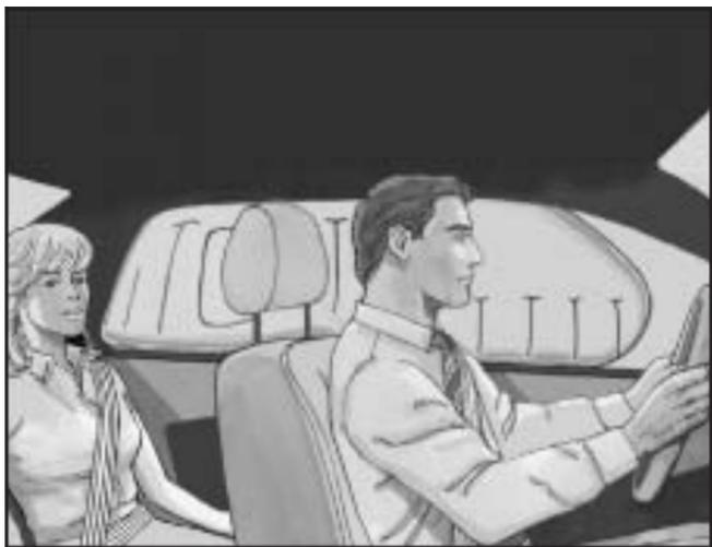
The roof-mounted side impact airbag for the driver and the person seated directly behind the driver is in the ceiling above the side windows.
