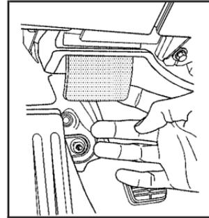
2. Pull down on the rear edge of the lever to release the hood latch.
