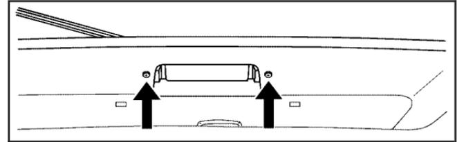
1. Remove the two screws holding the license plate lamp assembly to the fascia.
