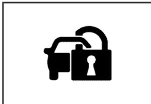
This light flashes when the vehicle security system is activated.
