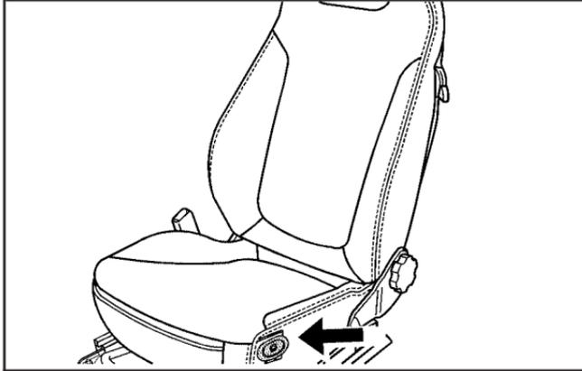
The switch is located on the outboard side of the driver's seat. To use the adjuster, first move the seat to where you want it. See *Manual Seats on page 8*. To raise or lower the seat, hold the switch up or down.
