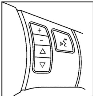
Radio controls are located on the right side of the steering wheel and if your vehicle has this feature, some audio controls can be adjusted at this location. They include the following.
