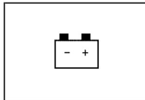
The charging system light will come on briefly when you turn on the ignition, and when the engine is not running, as a check to show you it is working.
