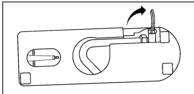
2. Unlock the air compressor hose from the sealant canister by pulling up on the lever.
