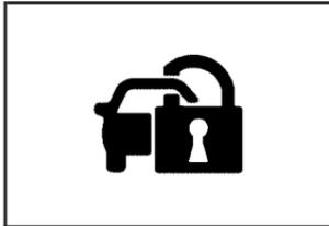
The security light, located on the instrument panel cluster, will turn on to indicate that arming has been initiated.
