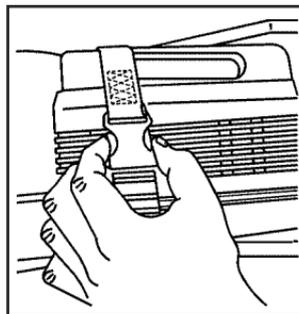
4. Remove the tire inflator kit strap by squeezing the two tabs of the quick release buckle.
