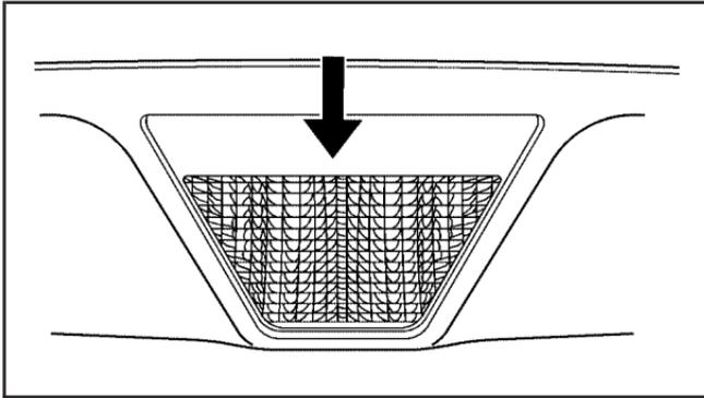
The back-up lamps are located in the rear bumper.
