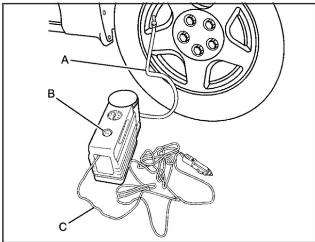
4. Attach the sealant filling hose (A) onto the tire valve stem. Turn it clockwise until it is tight. Make sure the inflator kit on/off switch (B) is in the O (off) position.
