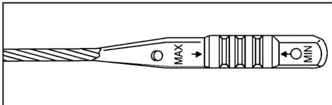
If the oil is below the MIN (minimum) mark, you will need to add at least one quart/liter of oil. But you must use the right kind. This section explains what kind of oil to use. For engine oil crankcase capacity, see *Capacities and Specifications* on page 331.
