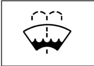
Open the cap with the washer symbol on it. Add washer fluid until the tank is full. See *Engine Compartment Overview on page 242* for reservoir location.
