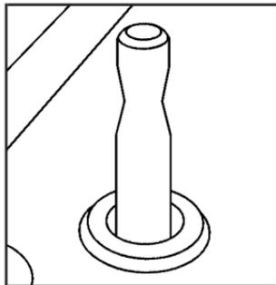
From inside the vehicle, use the manual door lock knob. Pull up or down on the knob to unlock or lock the door.
