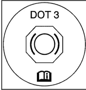
Your brake master cylinder reservoir is filled with DOT-3 brake fluid. See *Engine Compartment Overview* on page 242 for the location of the reservoir.
