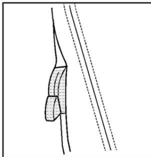
The seats have a latch located on the outboard side near the top of the seatback that enables the front seatback(s) to fold forward.
