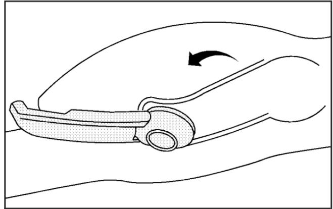
5. The convertible top front latch, located above the inside rearview mirror, must be unlatched. Pull the latch down and turn it counterclockwise to unlatch it.
