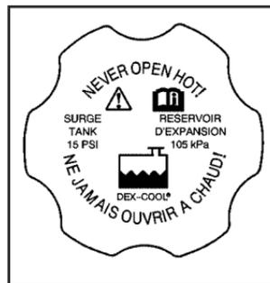
1. Remove the coolant surge tank pressure cap when the cooling system, including the coolant surge tank pressure cap and upper radiator hose, is no longer hot. Turn the pressure cap slowly counterclockwise about two or two and one-half turns. If you hear a hiss, wait for that to stop. This will allow any pressure still left to be vented out the discharge hose.
