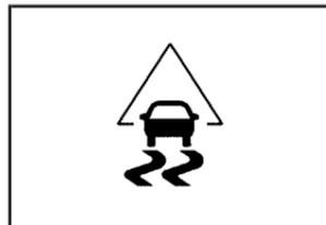
This light will flash when your traction control system is limiting wheel spin. You may feel or hear the system working, but this is normal.
