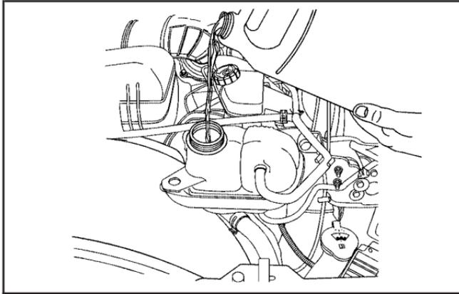
The coolant surge tank is located in the engine compartment on the driver's side of the vehicle. See *Engine Compartment Overview on page 242* for more information on location.
