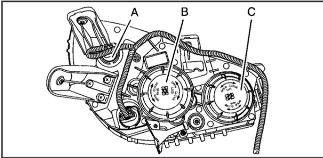
2. Remove the bulb access cover from the bulb (high or low-beam only) you need to change.
