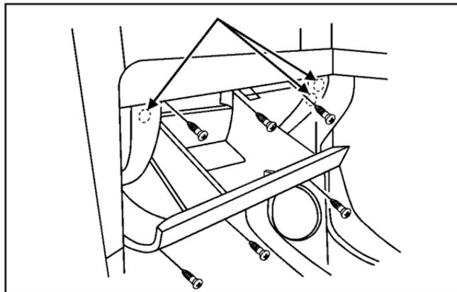
2. Lower the loosened glove box housing.
