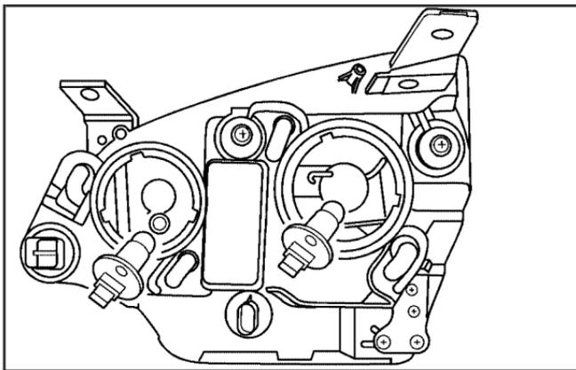
7. Disconnect the electrical connector from the bulb assembly.
