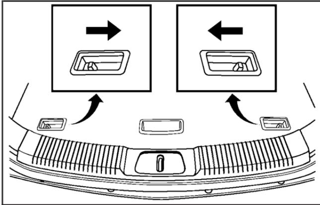
2. Push the levers on the load floor.
