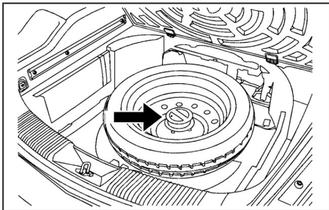
5. Remove the wheel retainer bolt holding down the spare tire by turning it counterclockwise.
