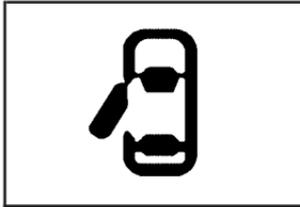
This light will come on when a door is open. Before driving, check that all doors are properly closed.
