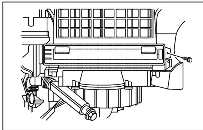
4. Remove the air filter cover screw.
