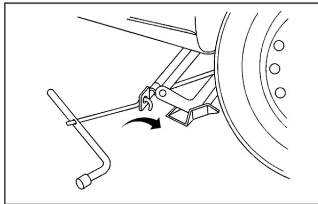
4. Position the lift head at the jack location nearest the flat tire. Make sure all of the jack lift head is touching the jacking flange under the body. Do not place the jack under a body panel. The lower body panel has an arrow to aid in locating the jacking location.
