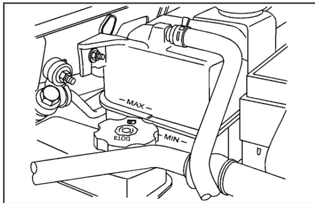
3. Fill the coolant surge tank with the proper DEX-COOL<sup>®</sup> coolant mixture, to between the MIN and MAX lines.
