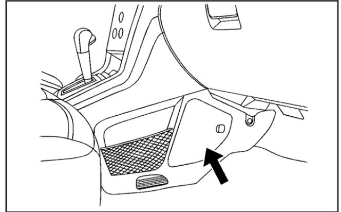
Pull the latch of the fuse box cover straight back to access the fuses.
