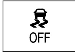
The TCS button is located on the instrument panel.
