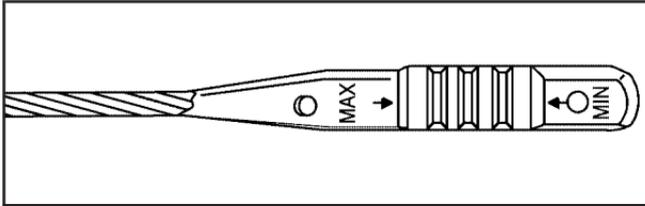
If the oil is below the MIN (minimum) mark, add at least one quart/liter of the recommended oil. This section explains what kind of oil to use. For engine oil crankcase capacity, see *Capacities and Specifications* on page 5-104.
