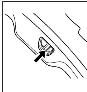
To open the liftgate if the vehicle's battery is disconnected or the voltage is low, access the release lever.
