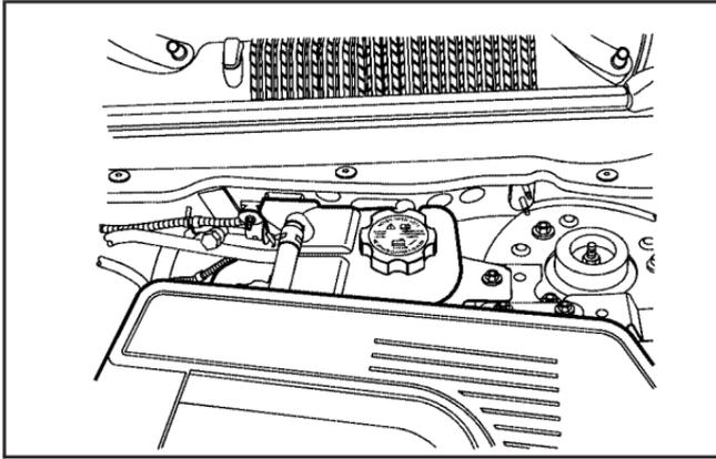
The surge tank is located on the driver side of the engine compartment. See *Engine Compartment Overview* on page 5-12 for more information on location.
