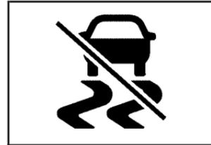
One of these TCS warning lights will be displayed on the instrument panel when the TCS is off.
