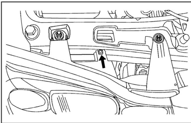
7. Locate the vertical headlamp aiming screws, which are under the hood near each headlamp assembly. The adjustment screw can be turned with a 6 mm socket.
