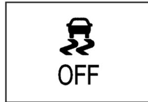
The traction control system can be activated again by pressing the traction control button.
