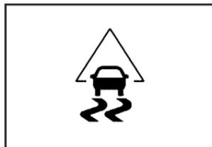
It will flash when the ESP system is both on and activated.
