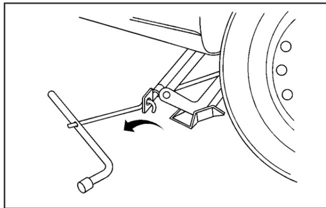
12. Lower the vehicle by turning the jack handle counterclockwise.
