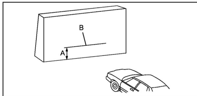
4. At the wall measure from the ground upward (A) to the recorded distance from Step 3 and mark it.
