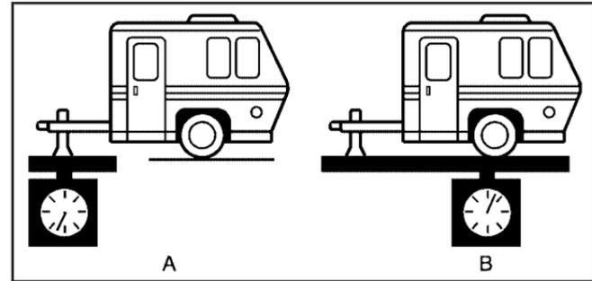
If you are using a weight-carrying hitch, the trailer tongue (A) should weigh 10 percent of the total loaded trailer weight (B). If you are using a weight-distributing hitch, the trailer tongue (A) should weigh 12 percent of the total loaded trailer weight (B).
