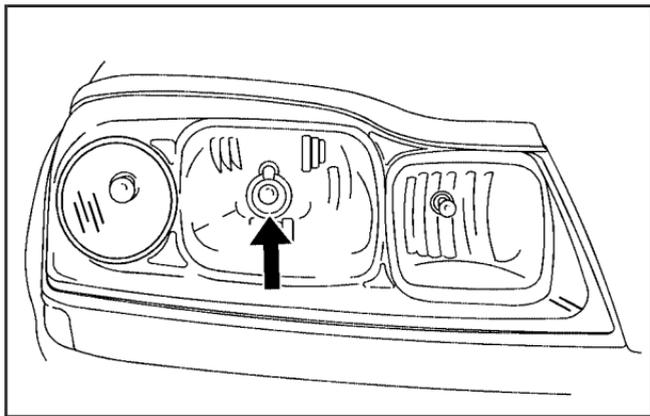
2. Locate the aim dot on the lens of the low-beam headlamp.
