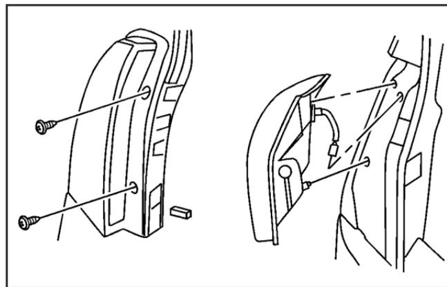
2. Remove the two screws holding in the taillamp assembly.
