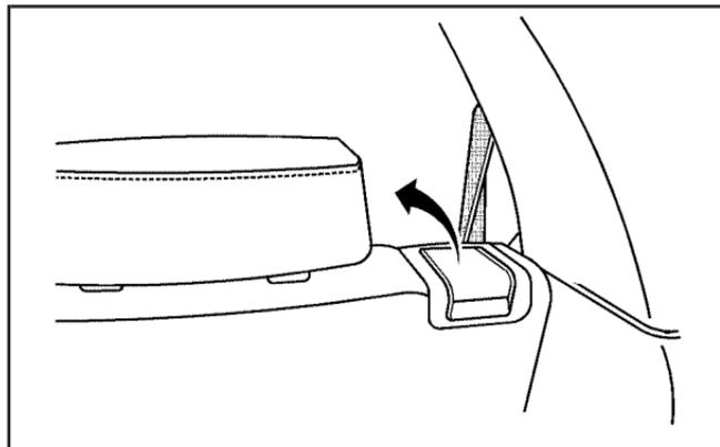
2. Lift the lever located on the top of the seatback to release the seatback and fold the seatback forward.
