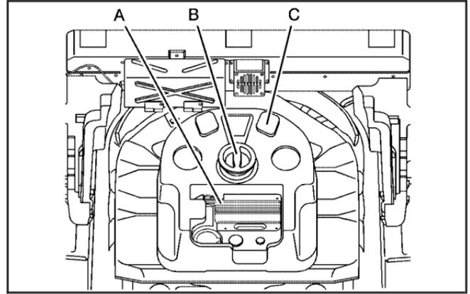
6. Remove the foam retainer bolt (B) holding down the foam container.
