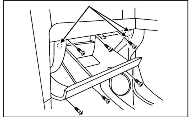
2. Lower the loosened glove box housing.
