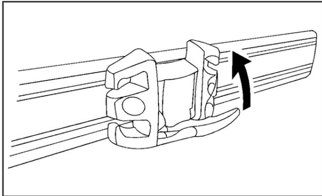
The adapters are used to hold the net. Slide the adapters to the desired location on the upper and lower groove of the rail and turn the handle up to lock it in place. Compress the rods of the net and insert them into the corresponding openings of the adapter. The longer rod is for the upper adapter.
