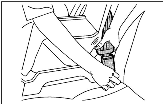
3. Push the latch plate into the buckle until it clicks. Make sure the release button is positioned so you would be able to unbuckle the safety belt quickly if necessary.
