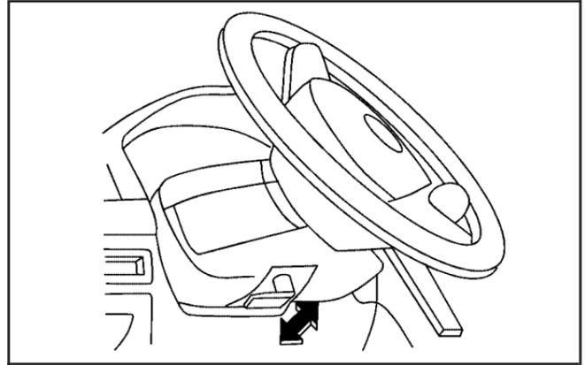
The tilt lever is on the lower left side of the steering column.
