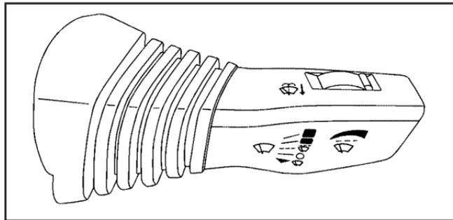
The lever on the right side of the steering column operates the windshield wipers. Push up or pull down on the lever to place it in one of the following positions.
