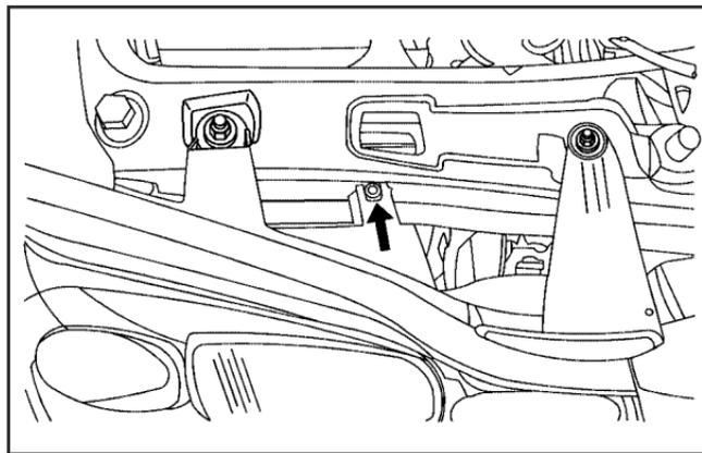
7. Locate the vertical headlamp aiming screws, which are under the hood near each headlamp assembly. The adjustment screw can be turned with a E8 Torx<sup>®</sup> socket.
