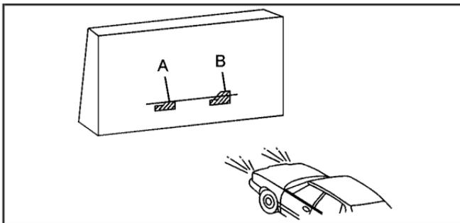
9. Make sure that the light from the headlamp is positioned at the bottom edge of the horizontal tape line. The lamp on the left (A) shows the correct headlamp aim. The lamp on the right (B) shows the incorrect headlamp aim.
