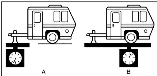
If you are using a weight-carrying hitch, the trailer tongue (A) should weigh 10 percent of the total loaded trailer weight (B). If you are using a weight-distributing hitch, the trailer tongue (A) should weigh 12 percent of the total loaded trailer weight (B).
