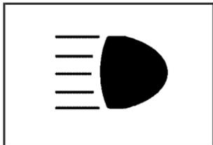
This indicator light turns on in the instrument panel cluster when the high beams are on.
