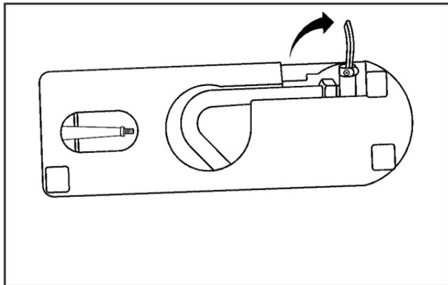
1. Unlock the air only hose from the sealant canister by pulling the lever up.
