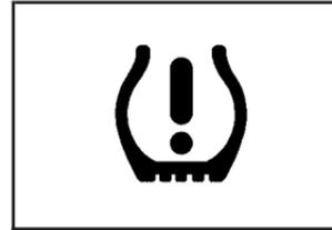
The tire pressure light comes on briefly when the engine is started.
