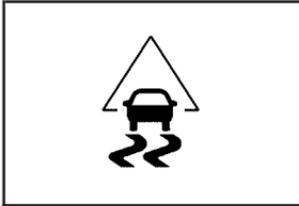
This light will flash when your traction control system is limiting wheel spin.
