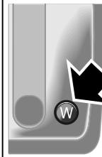
The Winter mode facilitates starting off and driving on icy roads. Third gear is selected automatically for starting off to reduce wheelspin.
