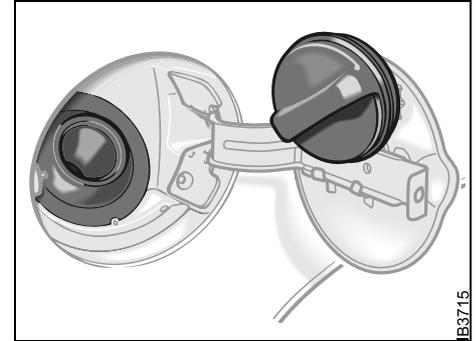
*When refueling, hang the filler cap inside the fuel door*
