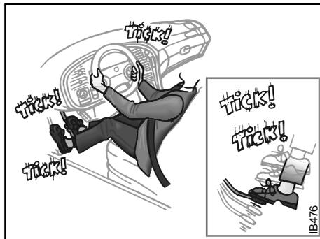
*Braking with ABS brakes.
