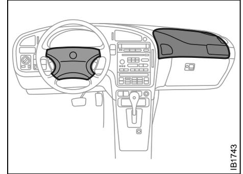
*Accessories and other equipment must not be fitted to the surfaces marked as these are where the airbags inflate in the event of a crash*
