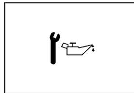
When this light comes on, it means that an oil change and other maintenance procedures are required for your vehicle.
