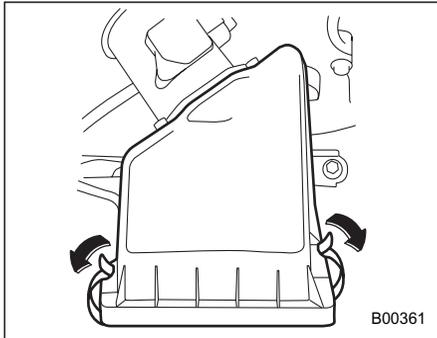
1. Unsnap the two clamps holding the air cleaner case cover.
