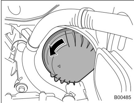
2. Remove the bulb cover by turning it counterclockwise.
