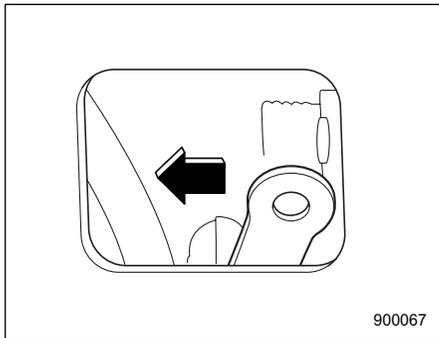
3. Unlock the rear liftgate by pressing the lever inside the trim to the left.
