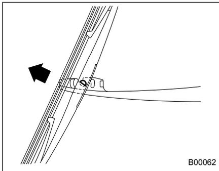
3. Pull the wiper blade assembly toward you to remove it from the wiper arm.
