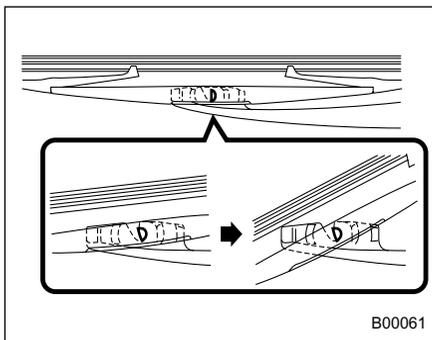
2. Turn the wiper blade assembly counterclockwise.
