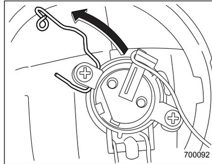
3. Push the retainer spring in the direction of the arrow to remove it from the hook.
