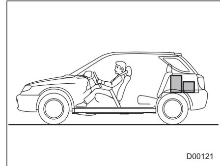
Vehicle capacity weight of the vehicle is 900 lbs (408 kg), which is indicated on the vehicle label with the statement “The combined weight of occupants and cargo should never exceed 900 lbs or 408 kg”.
