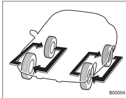
Tire wear varies from wheel to wheel. To maximize the life of each tire and ensure that the tires wear uniformly, it is best to rotate the tires every 7,500 miles (12,500 km). Rotating the tires involves switching the front and rear tires on the right-hand side of the vehicle and similarly switching the front and rear tires on the left-hand side of the vehicle. (Each tire must be kept on its original side of the vehicle.)
