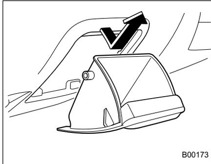
To remove the coin tray, open the cover and pull the coin tray out.
