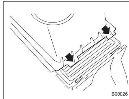
4. To install the air cleaner case cover, insert the two projections on the air cleaner case cover into the slits on the air cleaner case and then snap the two clamps on the air cleaner case cover.
