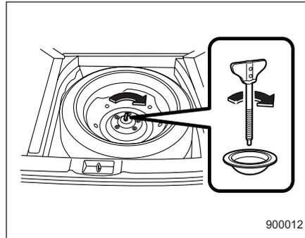
14. Store the flat tire in the spare tire compartment. Put the spacer and tighten the attaching bolt firmly.
