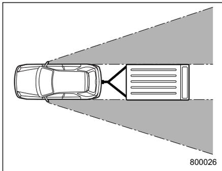
After hitching a trailer to your vehicle, check that the standard side mirrors pro-
