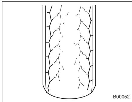
Ride comfort is poor. Also, the tire magnifies the effects of road-surface bumps and dips, possibly resulting in vehicle damage.
