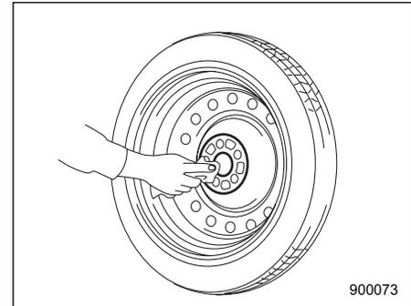
10. Before putting the spare tire on, clean the mounting surface of the wheel and hub with a cloth.
