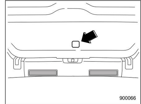
1. Remove the access cover at the bottom-center of the rear liftgate trim.
