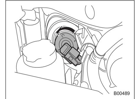
1. Remove the bulb from the headlight assembly by turning it counterclockwise.
