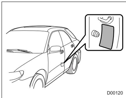
The vehicle label is affixed to the driver's side B-pillar (US). On Canadian vehicles this label is located inside the glovebox.
