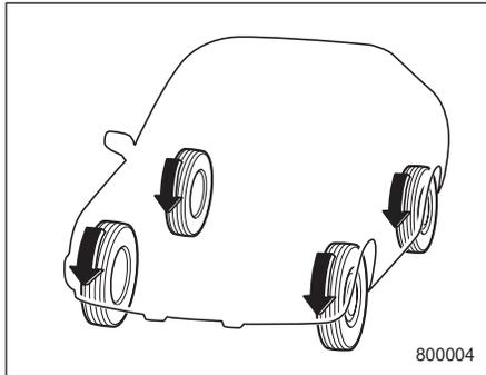
All-Wheel Drive distributes the engine power to all four wheels. AWD vehicles provide better traction when driving on slippery, wet or snow-covered roads and when moving out of mud, dirt and sand. By shifting power between the front and rear wheels, AWD can also provide added traction during acceleration and added engine braking force during deceleration.
