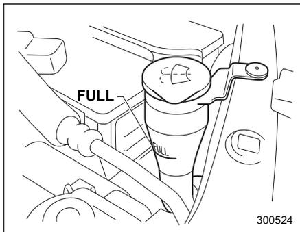
Remove the washer tank filler cap, then check the fluid level indicated by the level gauge (attached to the inside of the cap). If the level is near the "Low" mark, add flu-
