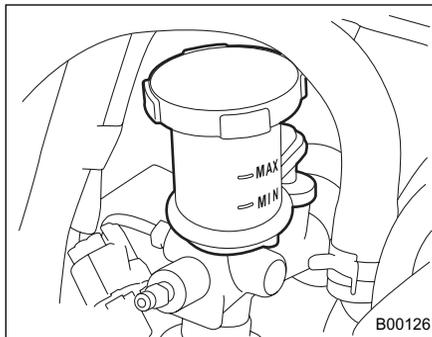
Check the fluid level on the outside of the reservoir. If the level is below “MIN” level mark, add the recommended clutch fluid to “MAX” level mark. Use only clutch fluid from a sealed container.
