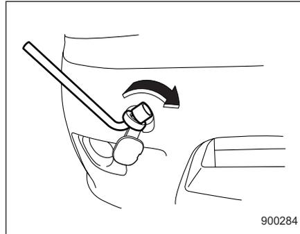
4. Tighten the towing hook securely using the wheel nut wrench.
