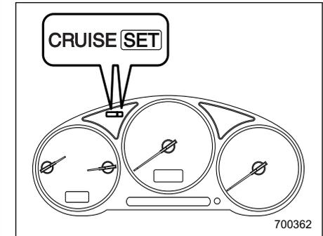
At this time, the “ SET ” indicator light is illuminated in the instrument cluster.
