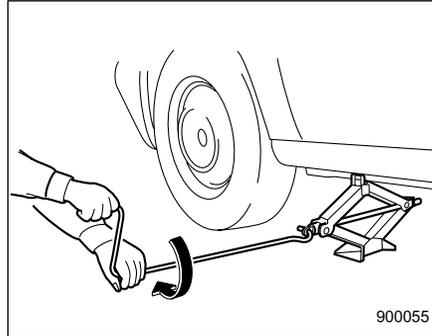
8. Insert the jack handle into the jackscrew, and turn the handle until the tire clears the ground. Do not raise the vehicle higher than necessary.
