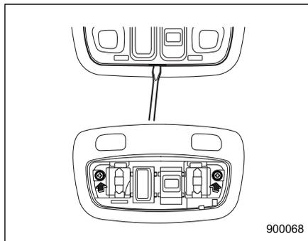
2. Remove the map light lens by prying the edge of the lens using a flat-head screwdriver.
