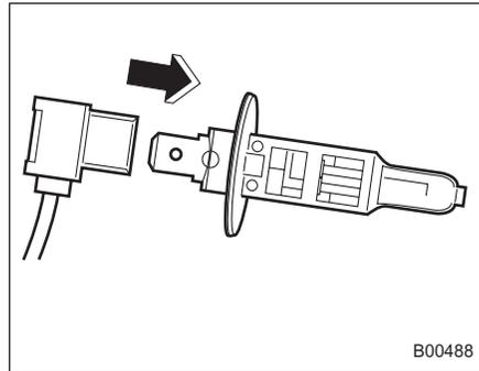
4. Pull the bulb out of the electrical connector. Replace the bulb with a new one.
