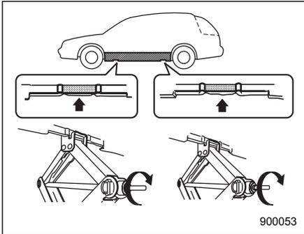
7. Place the jack under the side sill at the front or rear jack-up point closest to the flat tire.
