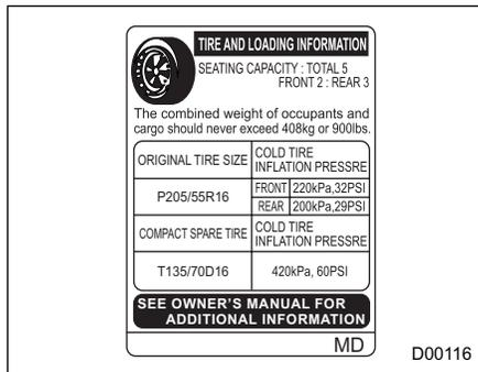
The vehicle label shows original tire size, recommended cold tire inflation pressure on each tire at maximum loaded vehicle weight, seating capacity and loading information.
