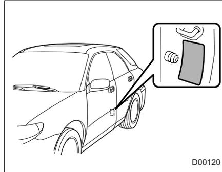
The load capacity of your vehicle is determined by weight, not by available cargo space. The maximum load you can carry in your vehicle is shown on the vehicle label attached to the driver's side door pillar. It includes the total weight of driver and all passengers and their belongings, any optional equipment such as a trailer hitch, roof rack or bike carrier, etc., and the tongue load of a trailer.
