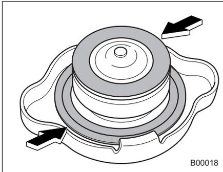
7. Put the radiator cap back on and tighten firmly. At this time, make sure that the
