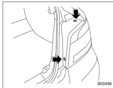
1. Using a Phillips screwdriver, remove the upper and lower clips that secure the side cover of the rear combination light assembly.
