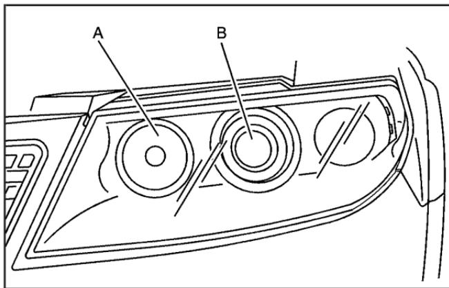
5. Remove the bulb socket that needs to be replaced by turning it counterclockwise.
