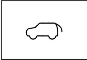
If this light comes on, the liftgate or liftglass is not completely shut.
