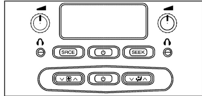
**⏻ (Power):** Press this button to turn the RSA on or off. The rear speakers are muted when the power is turned on.
