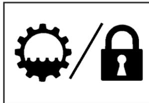
The automatic transmission dipstick handle with this symbol on it is located in the engine compartment on the passenger's side of the vehicle.
