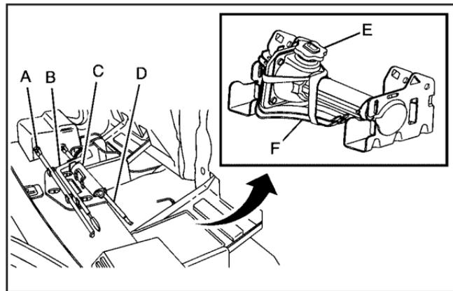
6. Make sure the tire is stored securely. Push, pull (A), and then try to turn (B) the tire. If the tire moves, use the wheel wrench and socket end of the extension to tighten the cable.
