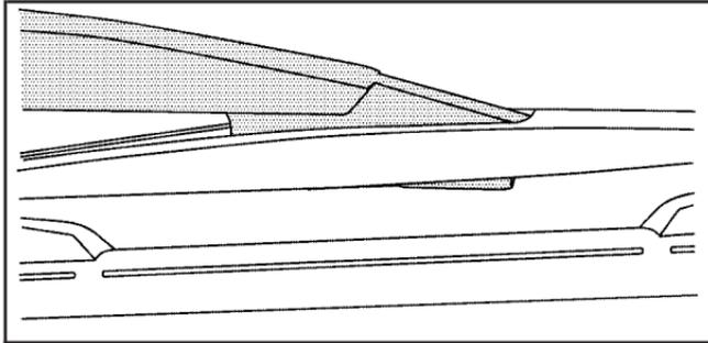
1. Lift the wiper blade assembly up and out of the park rest position.
