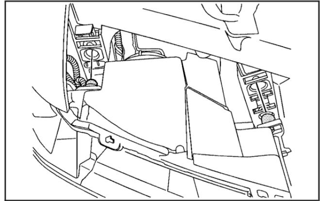
3. Pull the headlamp assembly away from the vehicle to access the electrical connectors.
