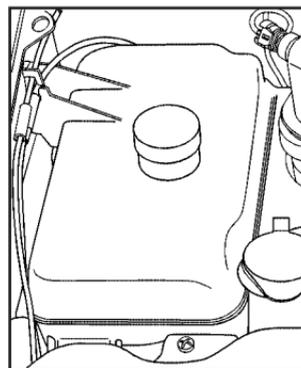
The coolant level should be at least up to the FULL COLD mark. If it is not, you may have a leak at the pressure cap or in the radiator hoses, heater hoses, radiator, water pump, or somewhere else in the cooling system.
