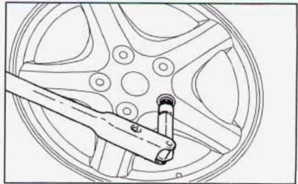
If your wheel has a bolt-on center cap, loosen the plastic caps using the wheel wrench.
