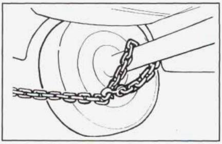
Attach a separate safety chain around each outboard end of the rear axle.
