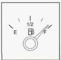
Your fuel gage shows about how much fuel is in your tank. The gage works only when the ignition switch is in the RUN position. When the gage pointer first indicates EMPTY (E) you need to get more right away.
