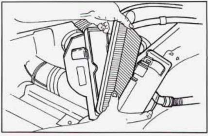
Pull the air cleaner straight up. Unclamp the metal clips.
