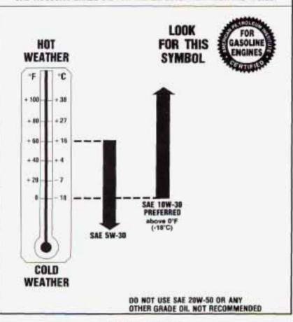
As shown in the chart, if you have the 3800 engine, SAE 10W-30 is best for your vehicle. However, you can use SAE 5W-30 if it's going to be colder than 60°F (16°C) before your next oil change. When it's very cold, you should use SAE 5W-30. These numbers on an oil container show its viscosity, or thickness. Do not use other viscosity oils, such as SAE 20W-50.
