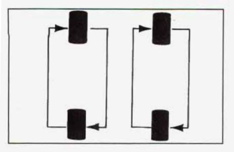
If you have P245/50ZR16 or P275/40ZR17 Goodyear Eagle GS-C tires, they must roll in a certain direction for the best overall performance. The direction is shown by an arrow on the sidewall. Because these tires are directional, they should be rotated as shown here. These tires should only be moved from front to rear and rear to front on the same side of the vehicle. Don't include the compact spare tire in your tire rotation.
