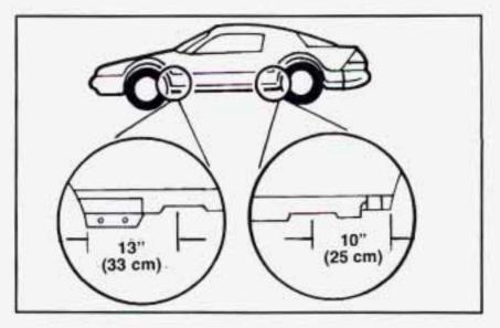
Position the jack under the vehicle. There is a notch in the vehicle's rocker flange on the coupe model. Raise the jack head until it fits firmly into the notch nearest the flat tire.
