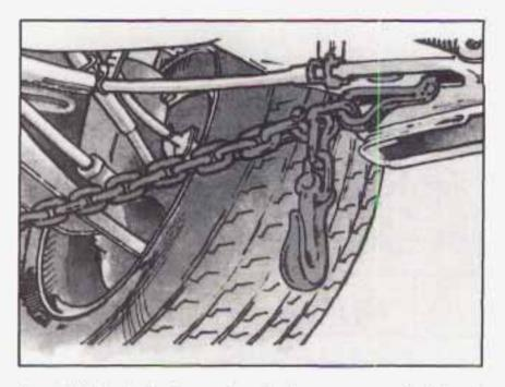
Attach T-hook chains to slots in frame rearward of front wheels on both sides.
