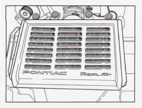
If you have the 5.7L LT1 engine (with the WS6 option), your air cleaner will be located over the radiator near the front of the engine.
