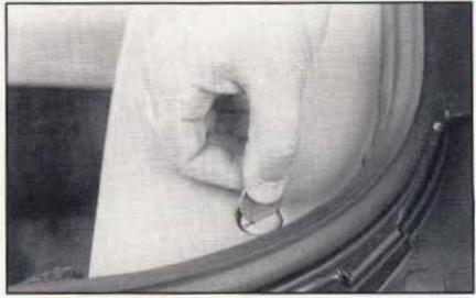
Find the plastic screw heads in the trim panel over the spare tire. (See "Compact Spare Tire" later in this section for more information about the compact spare.) Use a coin or a key to turn the screw heads until the slots point front and back. Gently lift the trim panel and move it out of the way.
