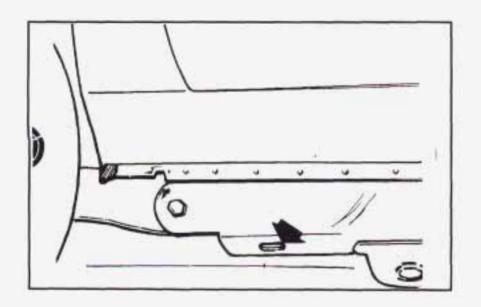
Attach T-hook chains in front of rear wheels in bottom of frame rail on both sides.
