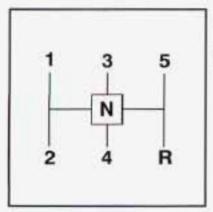
This is your shift pattern. Here's how to operate your transmission: FIRST (1): Press the clutch pedal and shift into FIRST (1). Then slowly let up on the clutch pedal as you press the accelerator pedal.
