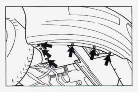
Using a screwdriver, remove the plastic screws from the deflector under the vehicle. Move the deflector out of the way.
