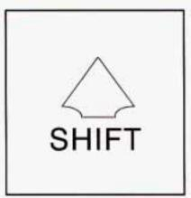
This light comes on when you need to shift to the next higher gear. See "Manual Transaxle" in the Index.
