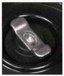
Turn the wing nut counterclockwise and remove it. Then lift off the spacer and remove the spare tire.
