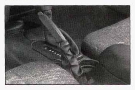
To set the parking brake, hold the regular brake pedal down with your right foot. Pull up on the parking brake handle. If the ignition is on, the brake system warning light will come on. To release the parking brake, hold the regular brake pedal down. Pull the parking brake lever up until you can press the release button. Hold the release button in as you move the brake lever all the way down.
