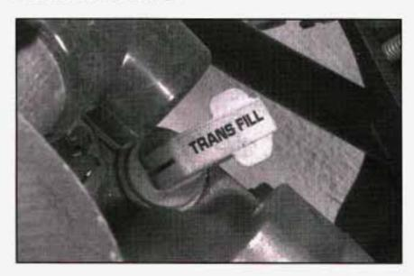
The manual transaxle dipstick is white and is located on the driver's side rear of the engine.
