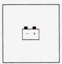
The charging system indicator light will come on briefly when you turn on the ignition, but the engine is not running. The light will go out when the engine is started.
