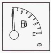
Your fuel gage tells you about how much fuel you have left, when the ignition is on. When the indicator nears EMPTY (E), you still have a little fuel left, but you should get more soon. An amber light will come on below the gage when the fuel tank is near EMPTY (E). Here are four things that some owners ask about. None of these show a problem with your fuel gage:
