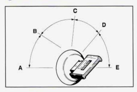
With the key in the ignition switch, you can turn the switch to five positions. ACCESSORY (A): This position lets you use things like the radio and windshield wipers when the engine is off. To use ACCESSORY, push in the key and turn it toward you. Your steering wheel will stay locked.
