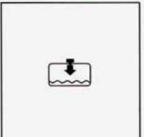
If the low coolant light comes on, it means you're low on engine coolant.
