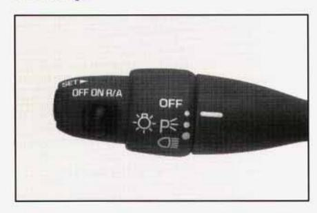
Rotate the turn signal lever middle ring up one position to turn on:
