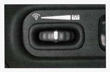
You can brighten or dim your instrument cluster lamps by rotating the instrument panel intensity control switch. Rotate the switch all the way to the right to turn on the interior courtesy lamps. Rotate the switch to the left to turn off the instrument cluster lamps and displays.
