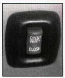
Open the sunshade by hand when using the vent position. Press and release the rear of the switch and the sunroof will open to the vent position.
