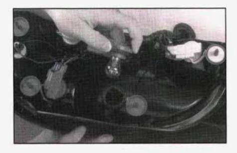
To remove a socket, push in the lock tab and turn the socket counterclockwise to pull it out
