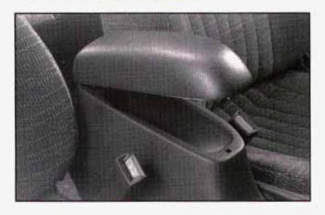
The armrest opens into a storage area for cassette tapes, gloves, etc. To open it, lift up on the front portion of the armrest.
