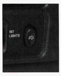
The button for your fog lamps is beside the instrument panel intensity control.
