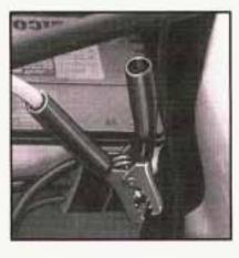
Now connect the black negative (-) cable to the good battery's negative (-) terminal.
