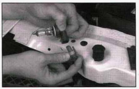
Unclip the bulb assembly from the wiring harness.
