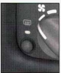
The rear window defogger uses a warming grid to remove fog from the rear window. Press the defogger switch. The indicator light will glow. If your vehicle is traveling under 45 mph (70 km/h), the rear window defogger will turn off automatically after about 10 minutes of use. If your vehicle is traveling over 45 mph (70 km/h), the defogger will operate continuously. You can turn the defogger off by turning off the ignition or pressing the switch again.
