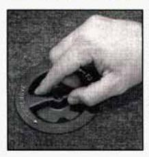
The equipment you'll need is in the trunk. Pull the carpeting from the floor of the trunk. Turn the center retainer nut on the compact spare cover counterclockwise to remove it.
