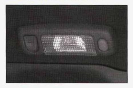
These overhead lamps and the interior courtesy lamps will come on when you open the doors.
