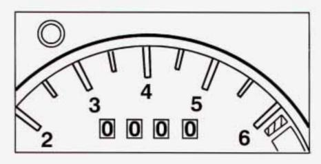
The trip odometer can tell you how far you have driven since you last reset it. To reset the trip odometer to zero, press the knob at the top left side of the instrument panel cluster.
