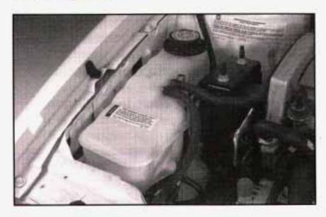
The coolant surge tank is located on the passenger's side of the engine compartment.
