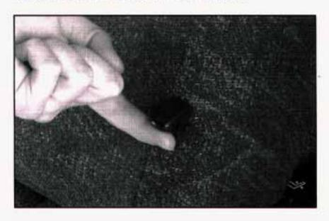
The front seatback folds forward to let people get into the back seat. To fold a front seatback forward, lift the seatback latch.
