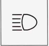
To change the headlamps from low beam to high or high to low, pull the turn signal lever all the way toward you. Then release it. When the high beams are on, a light on the instrument panel also will be on.
