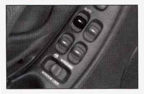
The power window switches are located on the door armrests; the driver's door armrest has controls for all of the windows. These switches will only work when the ignition is on.
