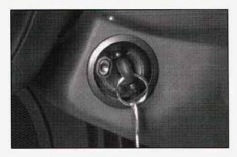
The key cannot be removed from the ignition unless the key release button is used.
