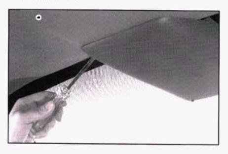
Using a flat screwdriver, remove the screws holding the bulb assembly.
