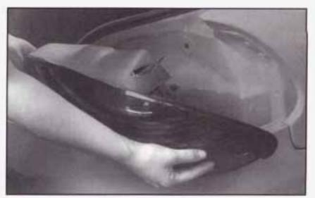
Carefully remove the taillamp assembly. Be careful to avoid scratching or chipping the paint on the vehicle.
