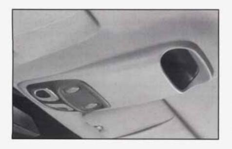
The optional overhead console has reading lamps, storage compartments (including one for your garage door opener and one for sunglasses) and an accessory power outlet. These features are explained on the following pages. **READING LAMPS:** To turn either reading lamp on or off, press the switch next to it.
