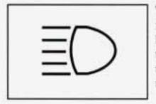
To change your headlamps from low beam to high beam, or high to low, pull the multifunction lever all the way toward you. Then release it.
