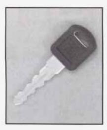
The master key can be used for the ignition, as well as all door locks and storage compartments.
