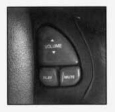
If your vehicle has this feature, you can control certain radio and remote playback functions using the buttons on your steering wheel. VOLUME: Press the up or down arrow to increase or decrease volume.
