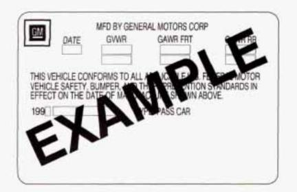
The other label is the Certification label, found on the rear edge of the driver's door. It tells you the gross weight capacity of your vehicle, called the GVWR (Gross Vehicle Weight Rating). The GVWR includes the weight of the vehicle, all occupants, fuel and cargo. Never exceed the GVWR for your vehicle or the Gross Axle Weight Rating (GAWR) for either the front or rear axle.
