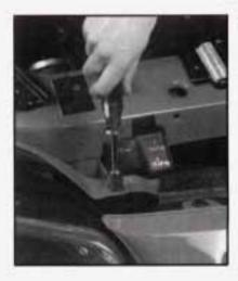
Remove the two bolts from the top of the headlamp assembly.
