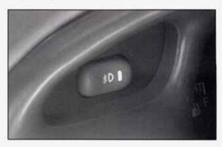
The fog lamps switch is located in the upper, left corner of the instrument panel, to the left of the instrument panel cluster. To turn the fog lamps on, press the right side of the fog lamps switch. A light will glow on the switch to let you know that they are on. (Your parking lamps must be on, or your fog lamps won't come on.) Press the left side of the switch to turn the fog lamps off.
