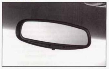
Your vehicle may have an electrochromic day/night rearview mirror. Push the button on the bottom of the mirror to turn this feature on. The mirror will darken gradually to reduce glare from headlamps behind you. This may take a few moments. One photocell on the front of the mirror senses when it is becoming dark outside. Another photocell, facing rearward, senses headlamps behind you. To turn the electrochromic feature off, press the button on the bottom of the mirror again.
