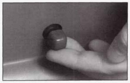
If you have this option, there will be a toggle switch on the left side of the driver's seat cushion, just in front of the reclining seatback lever. To increase or decrease lumbar support, push the switch forward or rearward. To adjust the lumbar support up or down, push the switch up or down.
