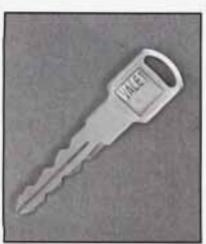
The valet key can be used for the ignition and the two side doors only. It will not open the trunk, glove box or fold down rear seat trunk access panel (if equipped). When a new vehicle is delivered, it will come with a bar coded tag attached to the key ring.
