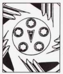
If there is a wheel cover, loosen the plastic nut caps with the wheel wrench. They won't come off. Then, using the flat end of the wheel wrench, pry along the edge of the cover until it comes off. Be careful; the edges may be sharp. Don't try to remove the cover with your bare hands.
