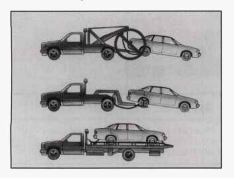
Use wheel-lift or car-carrier equipment. Additional ramping may be required for car-carrier equipment. Use safety chains and wheel straps. For rear towing, the parking brakes must be applied.
