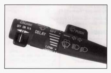
You control the windshield wipers by turning the band marked WIPER. For a single wiping cycle, turn the band to MIST. Hold it there until the wipers start, then let go. The wipers will stop after one cycle. If you want more cycles, hold the band on MIST longer. For steady wiping at low speed, turn the band to LOW. For high-speed wiping, turn the band further, to HIGH. To stop the wipers, turn the band to OFF.
