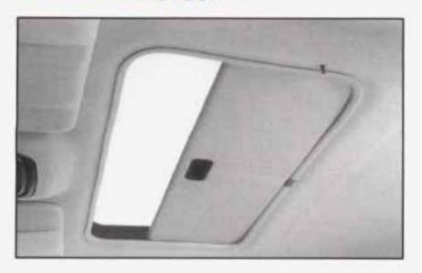
Your sunroof includes a sliding glass panel and a two-piece sunshade. The switch works only when the ignition or RAP is on. See "Retained Accessory Power" in the Index.
