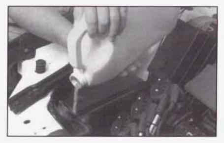
Fill the radiator with the proper DEX-COOL<sup>®</sup>
