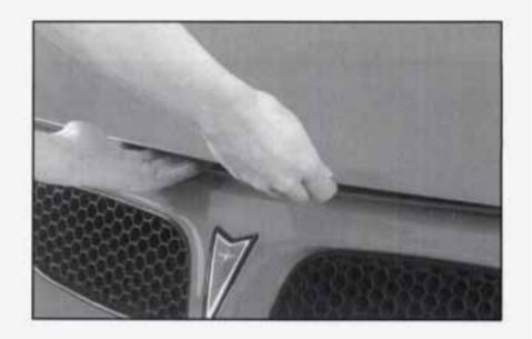
Next go to the front of the vehicle and release the secondary hood release. Lift the hood.
