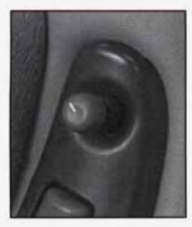
The electric mirror control is near the driver's window, on the armrest. Turn the control to the left to adjust the left mirror or to the right to adjust the right mirror. Then move the control in the direction you want to move the mirror.
