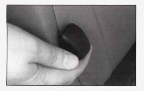
On two-door models, the right front seat is designed to make it easy to get in and out of the rear seat. Tilt the right seatback fully forward. The whole seat will now slide forward. If the seat will not tilt, lift the seatback latch, located on the back of the seat to tilt the seatback forward. The whole seat will now slide forward. After someone gets into the rear seat area, move the right front seatback to its original position. Then move the seat rearward until it locks.
