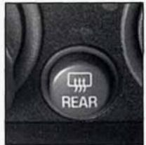
Your comfort control system has a button to operate your rear window defogger. The electronic comfort control system has a button marked REAR. The system with automatic temperature control has a button marked R.DEF. The rear window defogger uses a warming grid to remove fog from the rear window. Press the button to turn the rear defogger on. It will turn itself off after about ten minutes.
