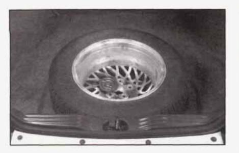
When storing a full-size tire, you must use the extension to help avoid wheel surface damage. Use the extension and protector/guide located in foam holder. To store a full-size tire, place the tire valve stem facing down, with protector/guide through a wheel bolt hole, remove the protector and attach the retainer securely. When reinstalling the compact spare, put the protector/guide back in the foam holder. Store the cover as far forward as possible.
