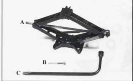
Turn the nut holding the jack to the left and remove it. Then remove the jack and wrench.
