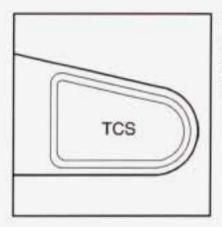
To turn the system off, press the TCS button on the far right end of the trip computer.
