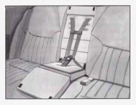
If your vehicle has this option, there's a built-in child restraint in the center rear seat position. This child restraint system conforms to all applicable Federal Motor Vehicle Safety Standards. This child restraint is designed for use only by children who weigh between 22 and 60 pounds (10 and 27 kg) and whose height is between 33.5 and 51 inches (850 and 1 295 mm) and who are capable of sitting upright alone.
