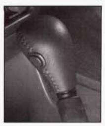
Press the performance shift button, located on the side of the console shift knob, to allow the transaxle to shift at higher engine speeds, increasing acceleration performance.
