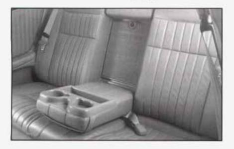
If your vehicle has rear seat armrests, you will also have a trunk access panel. To use the trunk access panel, pull your rear armrest down, unlock the access panel and pull it down.
