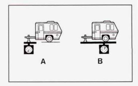
If you're using a weight-carrying hitch, the trailer tongue (A) should weigh 10 percent of the total loaded trailer weight (B). If you have a weight-distributing hitch, the trailer tongue (A) should weigh 12 percent of the total loaded trailer weight (B). After you've loaded your trailer, weigh the trailer and then the tongue, separately, to see if the weights are proper. If they aren't, you may be able to get them right simply by moving some items around in the trailer.
