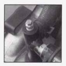
After the engine cools, open the coolant air bleed valve or valves.
