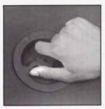
The equipment you'll need is in the trunk. Turn the center nut on the compact spare cover to the left to remove it.
