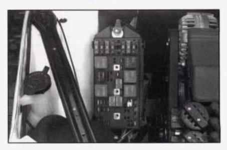
Some fuses are in a fuse block on the passenger's side of the engine compartment. Pull off the cover labeled FUSES to expose the fuses.
