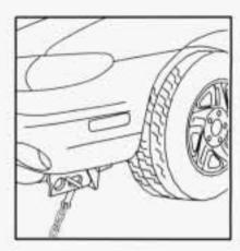
These slots are to be used when loading and securing to car-carrier equipment.
