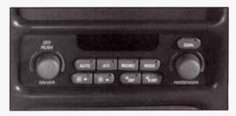
With this system, you set a "desired cabin" temperature. You can then either let the system automatically control airflow direction and amount (to maintain the desired cabin temperature) or you can manually adjust it. The system works best if you keep your windows closed while using it.
