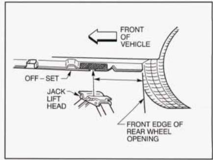
For jacking at the vehicle's front location, put jack lift about 6 inches (15 cm) from the rear edge of the front wheel opening or between the two bolts as shown. For jacking at the vehicle's rear location, put the jack lift head about 5.5 inches (14 cm) from the front edge of the rear wheel opening or just behind the off-set as shown.
