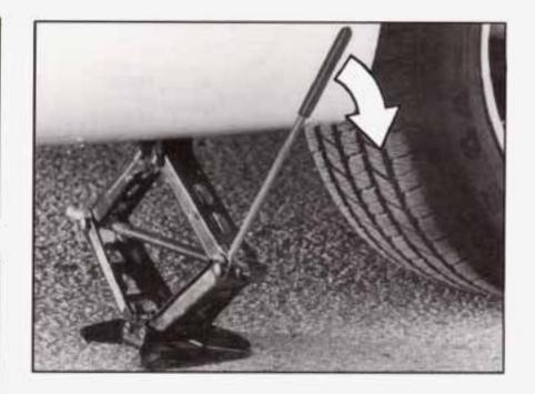
3. Raise the vehicle by turning the jack handle to the right. Raise the vehicle far enough off the ground for the spare tire to fit under the vehicle. Remove all wheel nuts and take off the flat tire.
