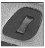
Your vehicle may be equipped with an express-open sunroof. Press the control switch rearward and release it to open the glass panel and sunshade.
