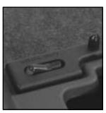
The trunk release lockout switch in the trunk allows you to secure items in the trunk.
