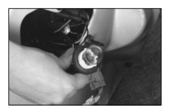
4. Replace the bulb and reverse the steps to install the new bulb assembly.
