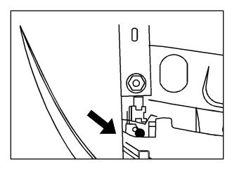
Start with the horizontal aim. The adjustment screws can be turned with
