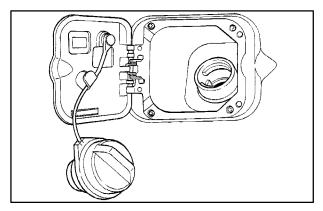
While refueling, hang the tethered cap on the hook on the inside of the fuel door.
