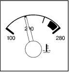
This gage shows the engine coolant temperature.
