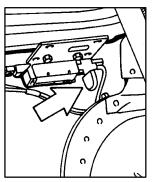
If your vehicle has a fuel door lock, the fuel door can be opened manually in case of an electrical power failure. Open the trunk. The release mechanism is on the driver's side of the vehicle, at the top of the trunk compartment. Pull the tab rearward to release the fuel door.
