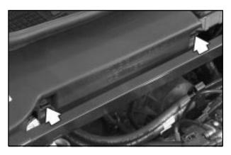
To check the fuses in this underhood fuse center, turn the two knobs one-quarter turn counterclockwise and loosen the metal wing nut on the passenger's side of the cover. Then remove the cover. The inside of the cover has a chart that explains the features and controls governed by each fuse and relay.
