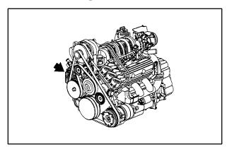
The power steering fluid reservoir is located on the rear passenger side of the engine compartment.
