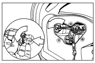
3. Turn the bulb socket assembly counterclockwise to remove it from the lamp assembly.
