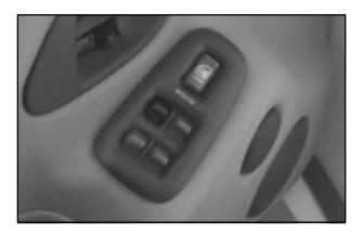
With power door locks, you can lock or unlock all the doors of your vehicle using the driver's or front passenger's door lock switch.
