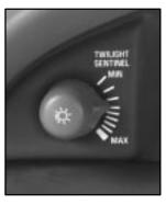
At night, you can turn off all exterior lamps when you are in PARK (P) by turning the twilight sentinel knob all the way to MIN.
