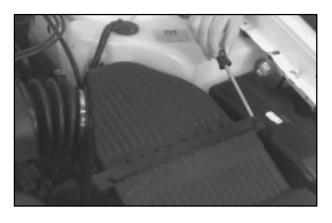
1. Remove the screws on the air cleaner housing cover.
