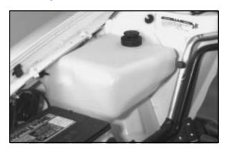
The vehicle must be on a level surface. When your engine is cold, the coolant level should be at the FULL COLD mark or a little higher. When your engine is warm, the level should be up to the FULL HOT mark or a little higher.
