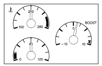
Vehicles equipped with the supercharged engine have this boost gage that indicates vacuum during light to moderate throttle and boost under heavier throttle. The gage displays the air pressure level in psi going into the engine's combustion chamber.
