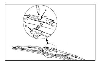
Replacement blades come in different types and are removed in different ways. Here's how to remove the type with a release hole:
