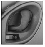
To lock the door from the inside, slide the locking lever rearward. To unlock the door, slide the locking lever forward.
