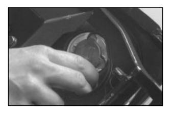
3. Tip the assembly and turn the bulb assembly counterclockwise to remove it.
