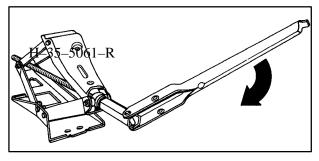
2. Turn the wheel wrench clockwise to raise the jack lift head until it fits under the vehicle.
