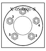
11. Tighten the wheel nuts firmly in a crisscross sequence.
