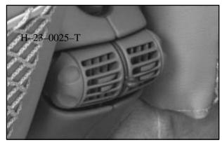
If you have the rear seat passenger outlet, it's attached to the back of the console. You can adjust the airflow toward either seating area, the floor or upward. Turn the end knobs up and down to direct airflow. Increase or reduce the amount of airflow by adjusting the lever between the two rear vents up or down. Open and close the louvers to direct airflow from side-to-side.
