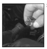
3. Disconnect the electrical connector which is attached to the air temperature sensor located in the hose.
