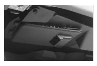
The driver's side fuse block is to the left of the steering wheel, under the instrument panel.
