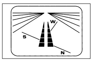
Some vehicles are equipped with an electronic compass. As with all compasses, this unit senses the earth's magnetic field to show the direction the car is pointing.
