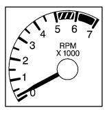
The tachometer shows your engine speed in revolutions per minute (rpm). Do not run your engine at speeds in the red area.
