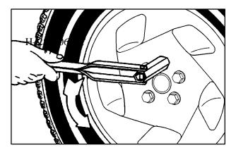
1. Use the wheel wrench to loosen the wheel nuts, but don't remove them.
