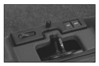
Some vehicles have an air inflator for use in maintaining proper air pressure for the tires. The air inflator is located in the trunk. The ON switch will work only with the ignition on.
