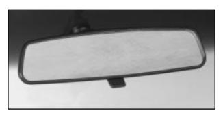
When you are sitting in a comfortable driving position, adjust the mirror so you can see clearly behind your vehicle. Grip the mirror in the center to move it up or down and side to side. The day/night adjustment allows you to adjust the mirror to avoid glare from the lamps behind you. Push the tab away from you for daytime use; pull it toward you for night use.
