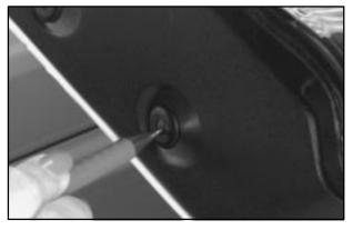
1. Push in on the center of the plastic push pin with a pen. The push pin should eject.
