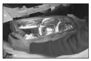
2. Slide the headlamp assembly outward (to the left) and lift it out.
