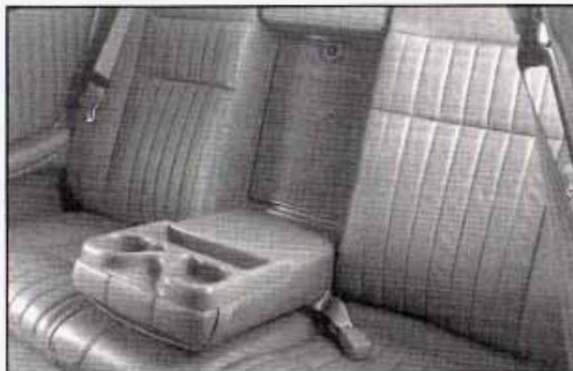
This feature allows access to the trunk from the rear seat area. To use the trunk access panel, pull the rear armrest down, unlock the access panel with the ignition key and pull it down.
