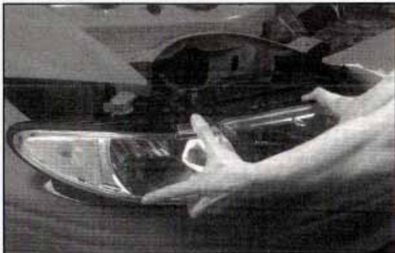
3. Carefully remove the headlamp assembly from the vehicle. Be careful to avoid scratching or chipping the paint on the vehicle while removing.
