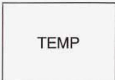
This light tells you that the engine coolant has overheated or the radiator cooling fan is not working.
