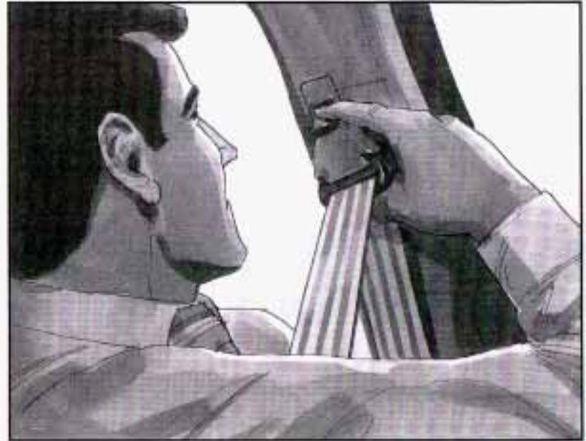
To move it down, squeeze the release lever and the shoulder belt guide as shown and move the height adjuster to the desired position. You can move the adjuster up just by pushing up on the shoulder belt guide. After you move the adjuster to where you want it, try to move it down without squeezing the release lever to make sure it has locked into position.
