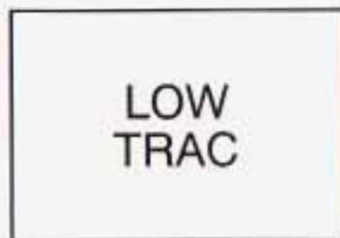
If your vehicle has the Enhanced Traction System or the Traction Control System, this light will also come on while the system is limiting wheel spin.
