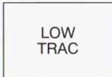
This light will come on when your Enhanced Traction System is limiting wheel spin. See *Enhanced Traction System Warning Light on page 3-29*.
