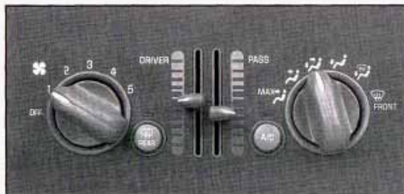
Use the mode knob located on the right side of the climate control panel to select the following modes:
