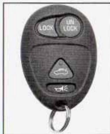
**LOCK:** To lock all the doors, press the LOCK button. See *Power Door Locks* on page 2-9 for more details on power door lock features.
