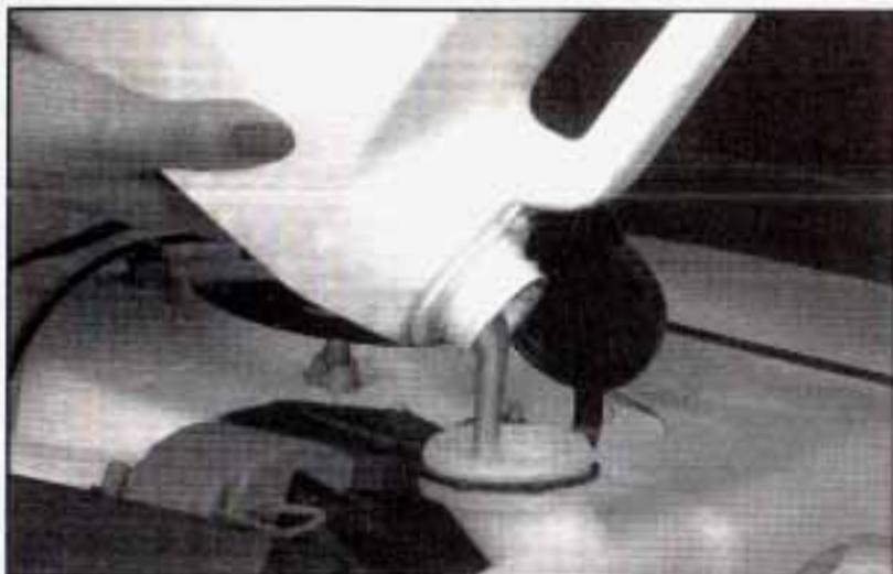
8. Then fill the coolant recovery tank to COLD mark.
