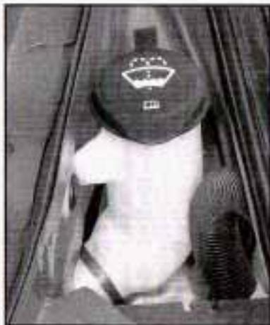
Open the cap with the washer symbol on it. Add washer fluid until the tank is full.
