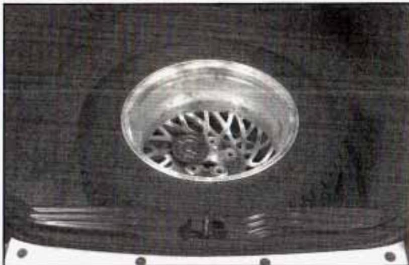
When storing a full-size tire, you must use the extension to help avoid wheel surface damage. Use the extension and protector/guide located in the foam holder. To store a full-size tire, place the tire in the trunk valve stem facing down, with the protector/guide placed through a wheel bolt hole. Remove the protector and attach the retainer securely. When putting the compact spare back in the trunk, place the protector/guide back in the foam holder. Store the cover as far forward as possible.
