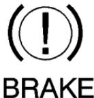
When your brake fluid falls to a low level, your brake warning light will come on. See *Brake System Warning Light* on page 3-27.
