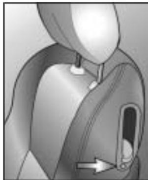
3. Press and hold the button under the front seat lever to return the seat to its original position. The seat will pause for two seconds when it reaches its original position.
