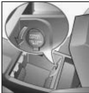
The vehicle has an accessory power outlet which can be used to plug in electrical equipment such as a cellular telephone, compact disc player, etc.
