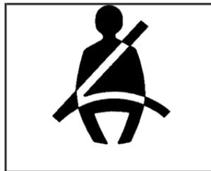
When the key is turned to ON, the safety belt light will come on and stay on for several seconds and a chime will be sounded for eight seconds, then it will flash continuously until the driver's belt is buckled.
