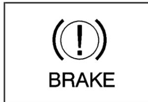
To check that the light is working, the symbol is displayed when the ignition is first turned ON and the park brake applied.
