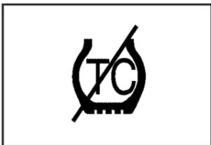
This symbol, along with the message TRACTION CONTROL OFF will display in the DIC for three seconds when the traction control system is disabled.
