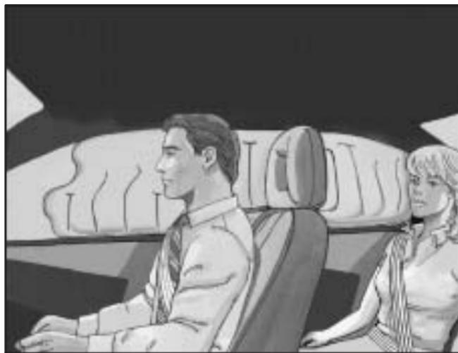
The side impact airbag for the right front passenger and the person seated directly behind that passenger is in the ceiling above the side windows.
