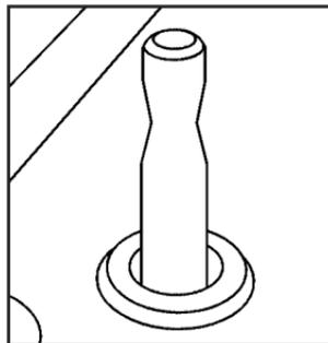
To manually lock or unlock the doors from inside the vehicle, push down or pull up on the door lock pin located on the top of each door panel.
