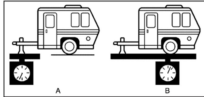
When using a weight-carrying hitch or a weight-distributing hitch, the trailer tongue (A) should weigh 10 to 15 percent of the total loaded trailer weight (B).
