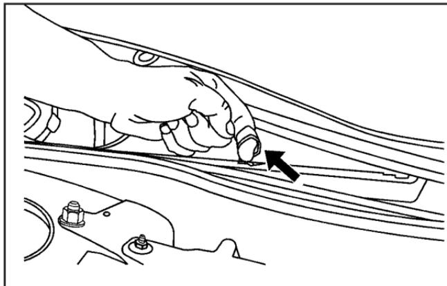
8. Remove the passenger compartment air filter by pulling on the tab.
