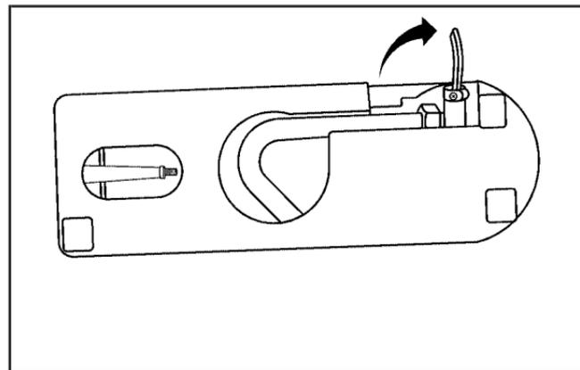
2. Unlock the air compressor hose from the sealant canister by pulling up on the lever.
