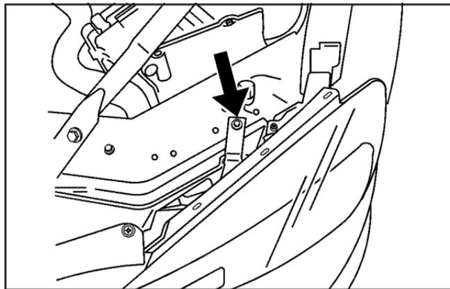
2. Locate the metal retaining clip. Remove the bolt.
