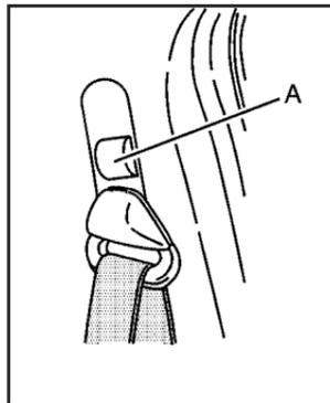
To move it down, pull the release button (A) out and move the height adjuster to the desired position. You can move the height adjuster up just by pushing up on the shoulder belt guide.
