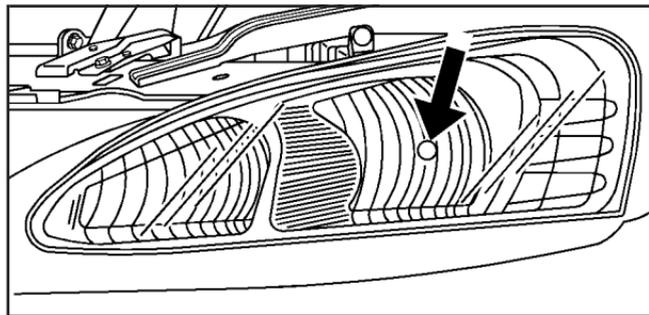
1. Find the aim dot on the lens of the low-beam lamp.
