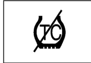
This symbol, along with the message TRACTION CONTROL OFF will display on the DIC for three seconds when the ETS is not on.
