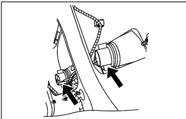
2. Turn the appropriate lamp socket a quarter turn counterclockwise and remove it.
