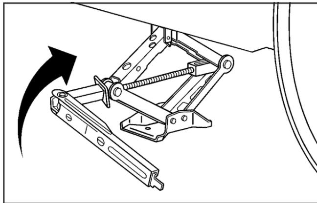
4. Raise the vehicle by turning the jack handle clockwise. Raise the vehicle far enough off the ground for the compact spare tire to fit underneath the wheel well of the vehicle.
