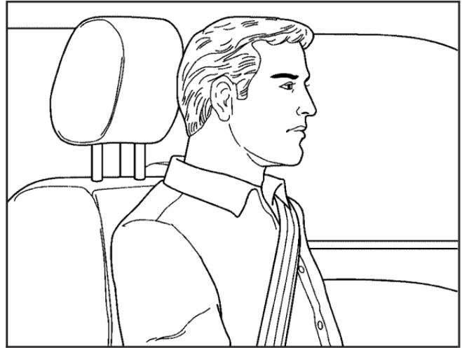
Adjust the head restraint so that the top of the restraint is closest to the top of the occupant's head. This position reduces the chance of a neck injury in a crash.
