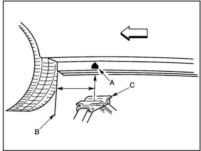
2. Find the jacking location using the diagram. For jacking at the vehicle's front location, put the jack lift head (C) about 6 inches (15 cm) from the rear edge of the front wheel opening (B). Line up the jack with the arrow (A) as shown.
