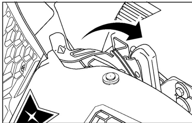
2. Go to the front of the vehicle and release the secondary hood latch, located near the center front of the engine compartment, by moving it to the right.
