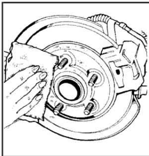
6. Remove any rust or dirt from the wheel bolts, mounting surfaces and spare wheel.
