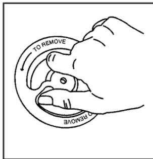
4. Turn the center nut on the compact spare tire cover counterclockwise to remove it.
