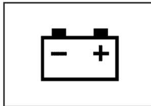
This symbol comes on with the CHARGING SYSTEM FAILURE warning message.
