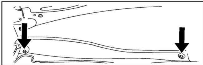
6. Remove the two air inlet grille retainers using a flat tool to first pry up on the center post and then the remainder of the fastener can be pulled out.
