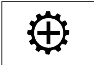
This symbol can appear on the instrument panel if the vehicle has a V8 or supercharged engine and the shift lever is in the manual transaxle position.
