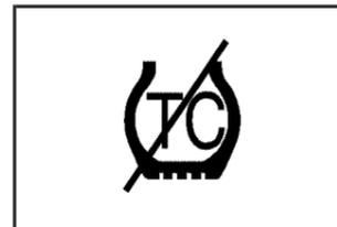
When the traction control system is not working, one of these symbols will come on the instrument panel cluster.
