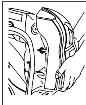
6. Remove the taillamp assembly by pulling it out from the vehicle.
