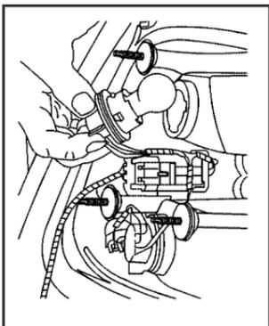
7. Turn the appropriate lamp socket a quarter turn counterclockwise and remove it.
