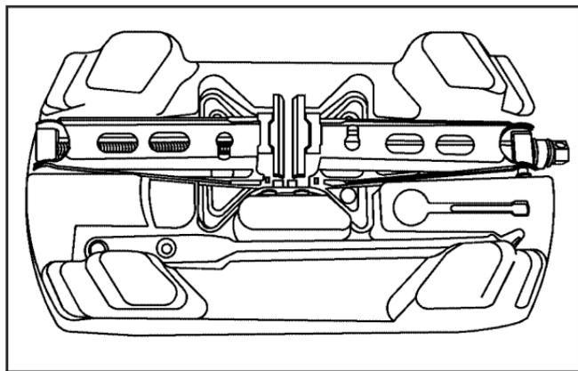
7. Turn the nut holding the jack counterclockwise and remove it. Then remove the jack and wrench.
