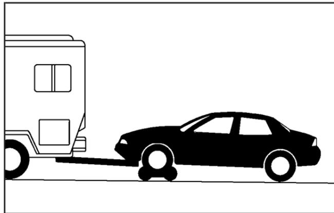
The vehicle can be towed using a dolly. To tow your vehicle using a dolly, follow these steps:
