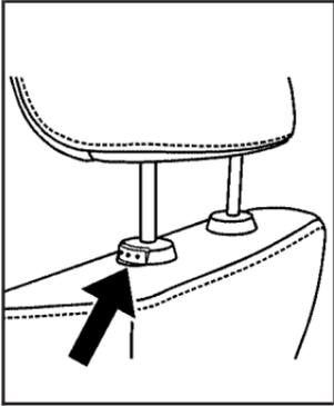
Pull up the head restraint to raise it. Press the release button, located at the base of the head restraint, and push the head restraint down to lower it.
