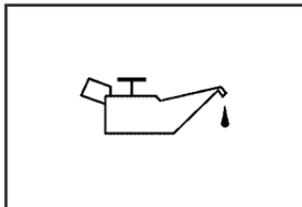
If there is a problem with the vehicle's oil pressure, this light may stay on when the engine is started, or it may come on while the vehicle is being driven.
