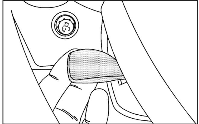
To tilt the steering wheel, hold it and pull the lever. Move the steering wheel to a comfortable driving position and release the lever to lock it into place.
