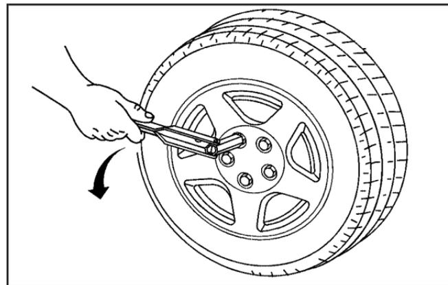
To remove the steel wheel covers and wheel nut caps, loosen the plastic nut caps with the wheel wrench in a counterclockwise direction. If needed, you can finish loosening them with your fingers. The plastic nut caps will not come off.
