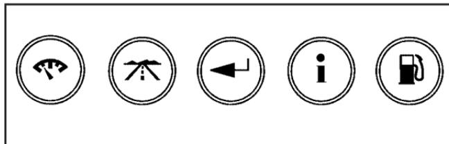
The buttons on the DIC trip computer are gages, trip odometer, set/reset, options, and fuel.
