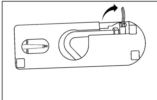
1. Unlock the air compressor inflator hose from the sealant canister by pulling the lever up.
