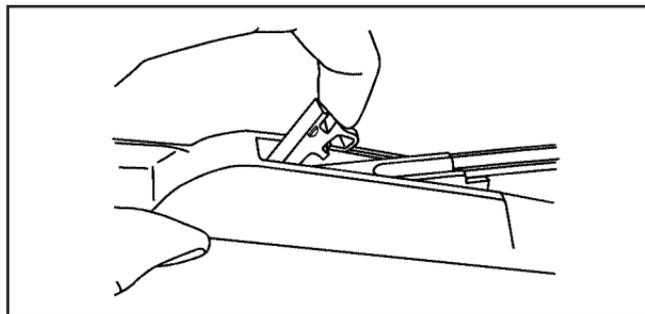
2. While holding the wiper arm, pull the clip up from the blade connecting point, and pull the blade assembly down toward the windshield to remove it from the wiper arm.
