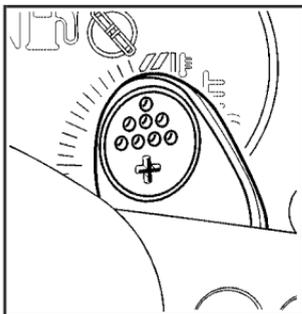
3. The paddles are located on the steering wheel. They are used to up-shift or down-shift the transaxle.
