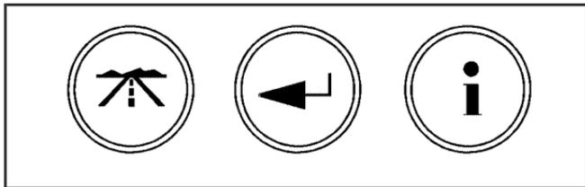
The buttons on the base level are trip odometer, set/reset, and options.
