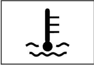
This light indicates that the engine coolant has overheated or the radiator cooling fan is not working.
