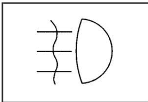
This symbol appears on the instrument panel cluster when the fog lamps are on.
