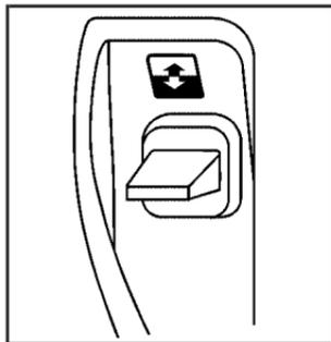
The switch to control the sunroof is located in the headliner.
