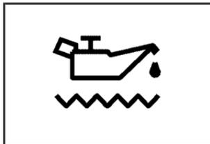
If this symbol, along with the LOW OIL LEVEL message appears on the Driver Information Center (DIC), it means you need to check the engine oil level right away.
