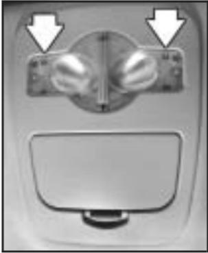
The overhead console has two reading lamps. Press the sides of each lens to turn the reading lamps on or off.
