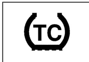
This symbol, along with the TRACTION CONTROL ACTIVE message, comes on the DIC screen when the system is active.
