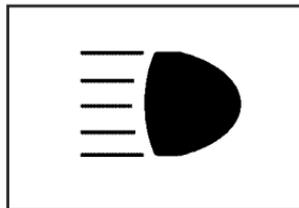
This symbol appears on the instrument panel cluster when the high-beam headlamps are on.
