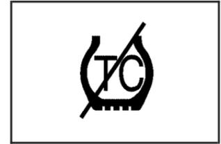
One of these lights will appear on the instrument panel to indicate that the ETS is not on.
