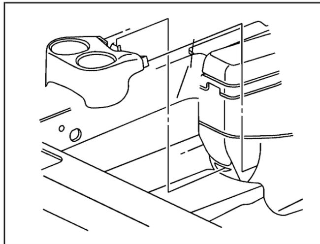
Remove the rear cupholder by pulling it from the console.
