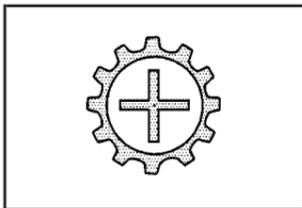
The up-shift light on the instrument panel cluster, or the up-shift symbol on the HUD, if equipped, is given as a prompt to use the TAP-Shift<sup>®</sup> paddle.
