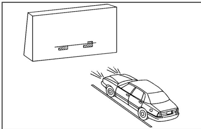
6. Ensure the top edge of the cut-off is positioned at the bottom edge of the horizontal tape line.
