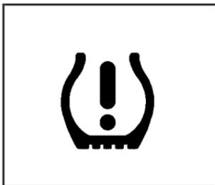
This symbol, along with the CHECK TIRE PRESSURE warning message, will appear in the Driver Information Center (DIC) if the pressure in one tire becomes 12 psi (83 kPa) lower than the other three tires.
